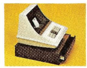
**Data Terminal** A self-contained, free standing unit with computer logic.
