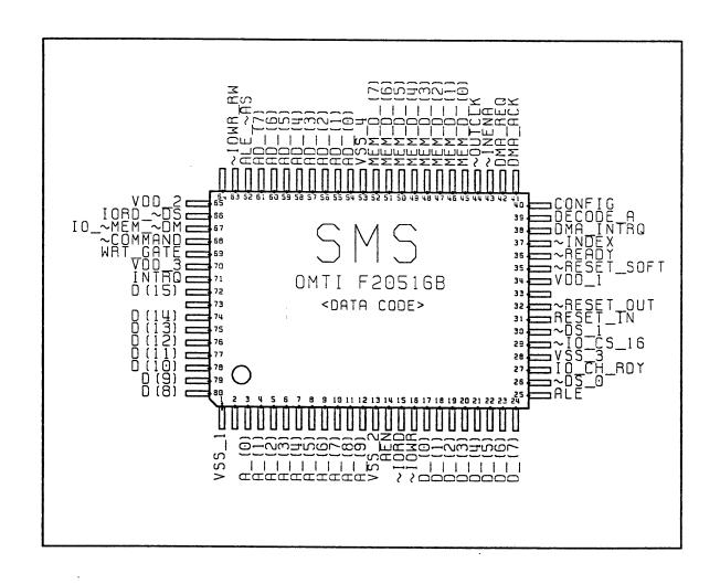
Figure 3. Pin Assignment 5098B 80 Pin PFP
