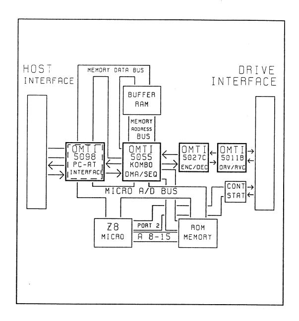
Figure 2. Controller Block Diagram
