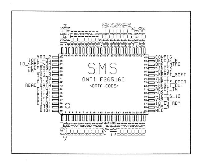
Figure 3. Pin Assignment 5098C 80 Pin PFP
