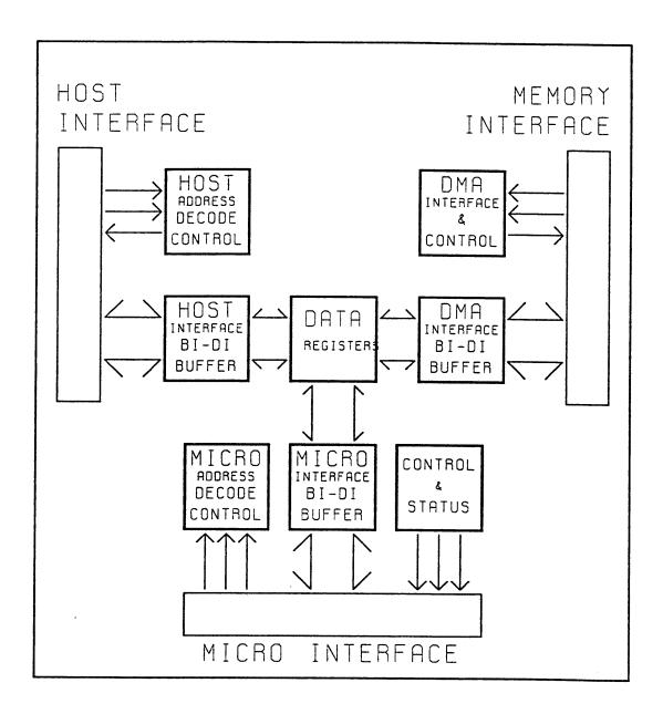
Figure 1. Internal Block Diagram
