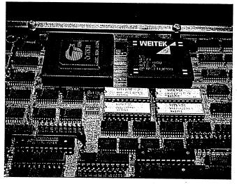
Powered by a 33-MHz Cypress Sparc chip, the Solbourne Series 5 CPU board blazes away at 22 mips
