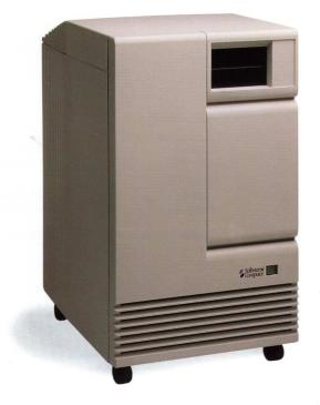
The Series5/670 combines up to 65 MIPS of compute power with up to 256 Mbytes of RAM and up to 2.6 Gbytes of bigh speed SCSI storage in a compact deskside unit.
