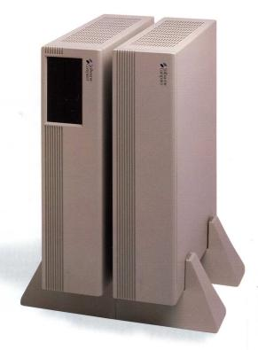
The Series 5/530 combines up to 40 MIPS of compute power with up to 256 Mbytes of RAM and up to 2.6 Gbytes of high speed SCSI storage in a compact under-desk twin tower configuration.
