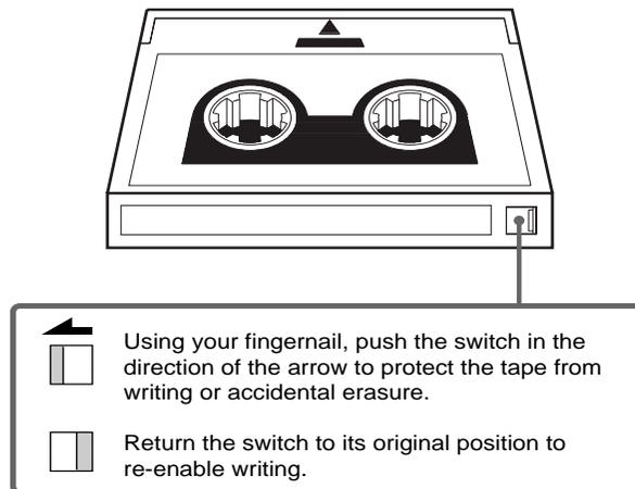
**Figure 4-1. Write-protect switch**
