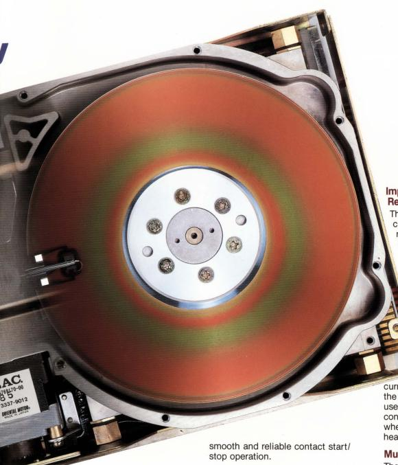
head movement. The speed and accuracy of the seek mode are further enhanced by a built-in microprocessor which controls the input step pulse.
