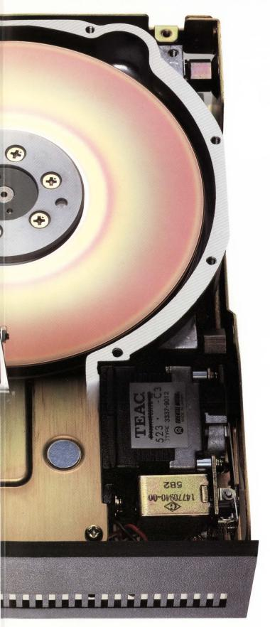
filter also ensures that a normal flow of air is maintained, protecting the heads and disks against temperature fluctuations. The head and disk unit is also protected from heat radiated by the motor through a configuration which maintains a stable temperature within the drive. This leads to substantial reductions in tracking errors, and makes it possible to initiate read/write operations as soon as the power is turned on.
