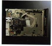
All components of the drive are laid out to take maximum advantage of Sony's robot technology. With only a single printed circuit board, all adjustments and inspections are performed using fully automated equipment, thereby further enhancing the quality and reliability of Sony's most advanced 3.5 inch floppydisk drives.
