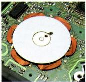
positioned with extreme accuracy by installing the rotor on the main chassis. The coils of the disk motor are directly mounted on the PCB which contributes to the drive's slimness, and through the use of a digital servo control mechanism, accurate rotational speed is maintained.
