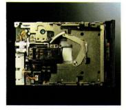
All components of the drive are laid out to take maximum advantage of Sony's robot technology. With only a single printed circuit, board, all adjustments and inspections are performed using fully automated equipment, thereby further enhancing the quality and reliability of Sony's most advanced 3.5 inch floppydisk drives
