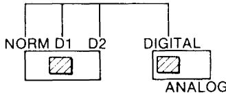
D2-DIGITAL: For TTL graphics cards on the IBM PC, AT and XT. (automatic adjustment between EGA, CGA and MDA)
