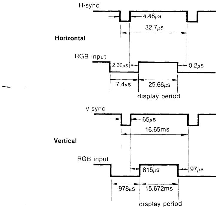
The indicated values apply when the line period is  $32.7\mu s$  and the field period is  $16.65ms$ .
