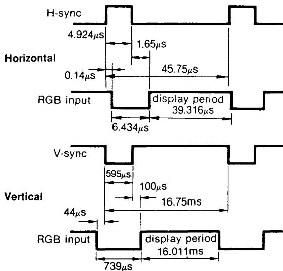
The indicated values apply when the line period is 45.75 $\mu$ s and the field period is 16.75ms.
