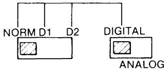
D1-DIGITAL: For microcomputers having TTL RGB and I signal output, such as the IBM PC, AT and XT using the standard color graphics card.
