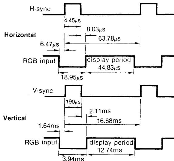
The indicated values apply when the line period is 63.78 $\mu$ s and the field period is 16.68ms.
