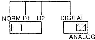
NORM-DIGITAL: For microcomputers having TTL RGB output, such as the IBM 3270.
