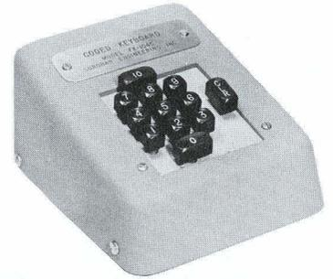
Almost all Soroban tape preparation equipments incorporate the versatile and reliable, custom designed series FK automatic coding keyboards. Since few users have comparable requirements, Soroban has established assembly procedures which permit prompt delivery of custom coding equipments. Keyboards can be supplied with key configurations and output codings tailored to meet unique customer requirements.
