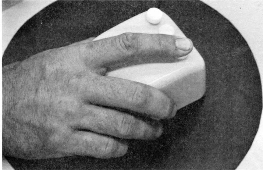
FIGURE 14. The user returns his left hand to the keyset and his right hand to the mouse. To confirm his command to compile the pattern "Research" he presses the right hand button on top of the mouse.
