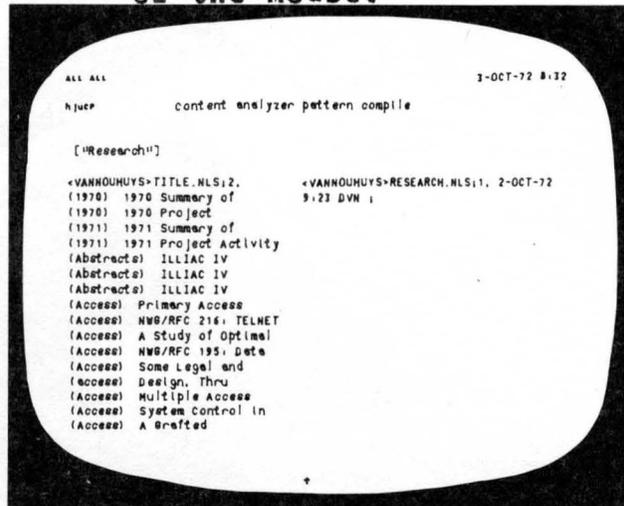
FIGURE 15. The text he entered appears in the literal feedback line on the upper left. The content analyser will act as a filter and pass only statements that contain the word Research. Patterns may be much more complex and include logical operators and classes of characters as well as specific characters.
