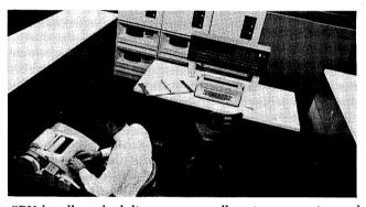
SPU handles scheduling, resource allocation, swapping and I/O functions. They share from 32K-256K of 36-bit plus parity two-usec main memory. The SPU has 16 registers; the ALP has multiple accumulators, seven index registers, and working locations in control memory.
