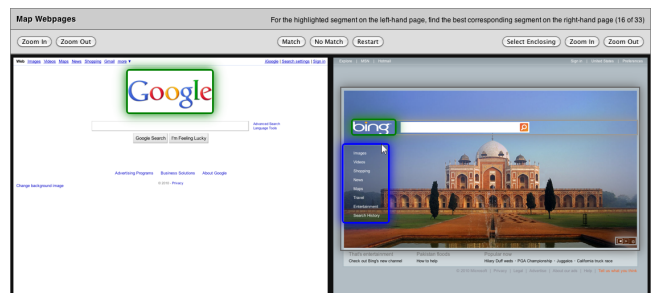
Figure 3: The Bricolage Collector Web application asks users to match each highlighted region in the left (content) page to the corresponding region in the right (layout) page. Zoom in for detail.
