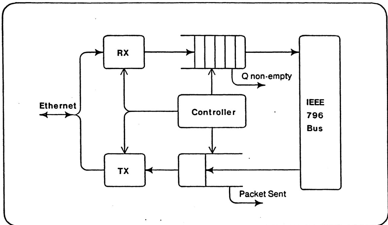
Figure 3: SUN Ethernet Block Diagram
