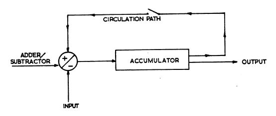
To clear an accumulator it is simply necessary to break the circulation path, and write in either zeros or new information.
