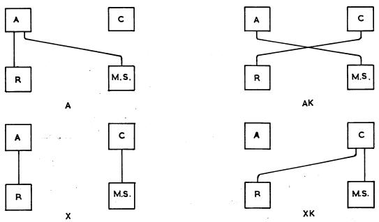
In each of these four combinations 'reading' from the stores has been taking place. 'Writing' into the Main Store occurs when D=1, and 'writing' into the Registers occurs when E=1.
