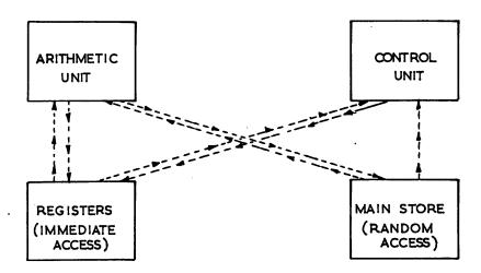
Any word transferred to the Main Store or Registers is automatically stored in a particular location, specified by the instruction causing the transfer. Any word transferred to the Arithmetic Unit is either added to or subtracted from the existing contents, or it replaces the existing contents. Any word transferred to the Control Unit will be an instruction, and if it includes test digits its execution will depend on certain conditions in the machine.
