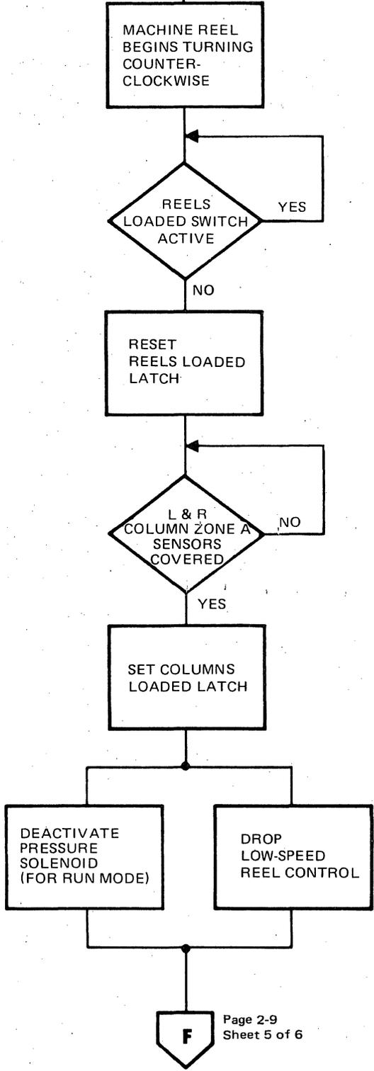
Figure 2-3. Thread/Load Flow Chart (Sheet 4 of 6)
