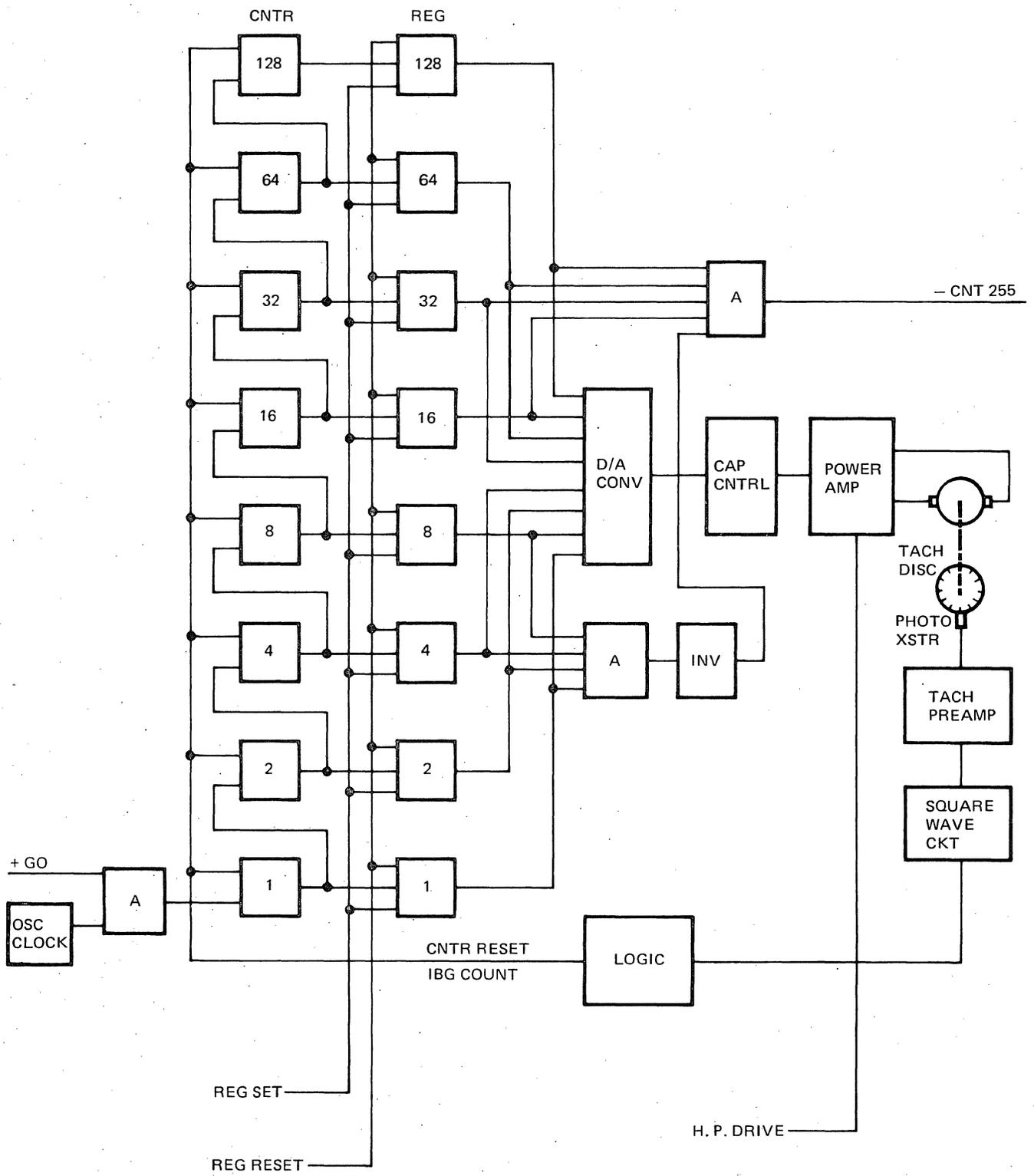
Figure 3-13. Capstan Velocity Control Block Diagram
