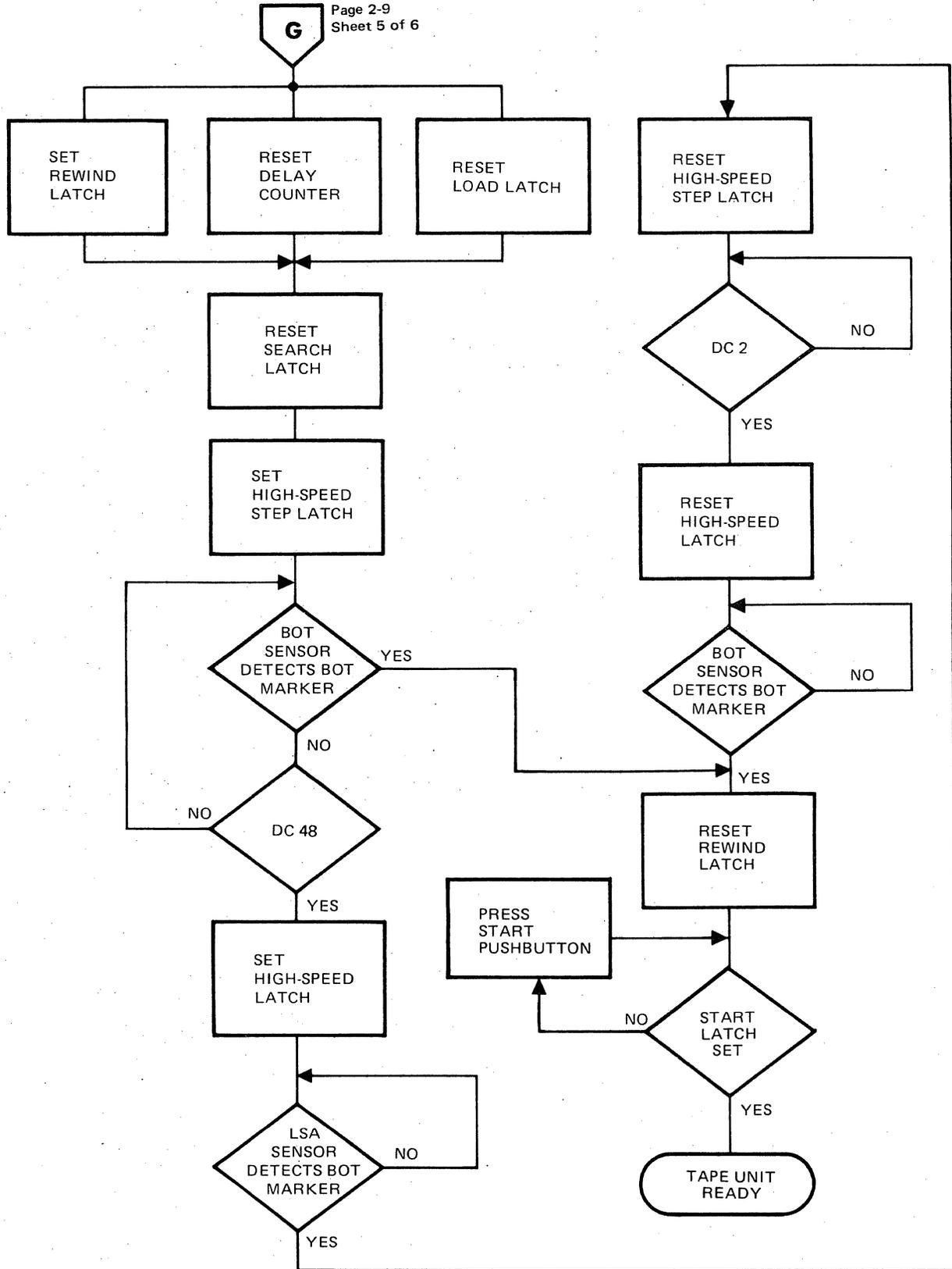
Figure 2-3. Thread/Load Flow Chart (Sheet 6 of 6)
