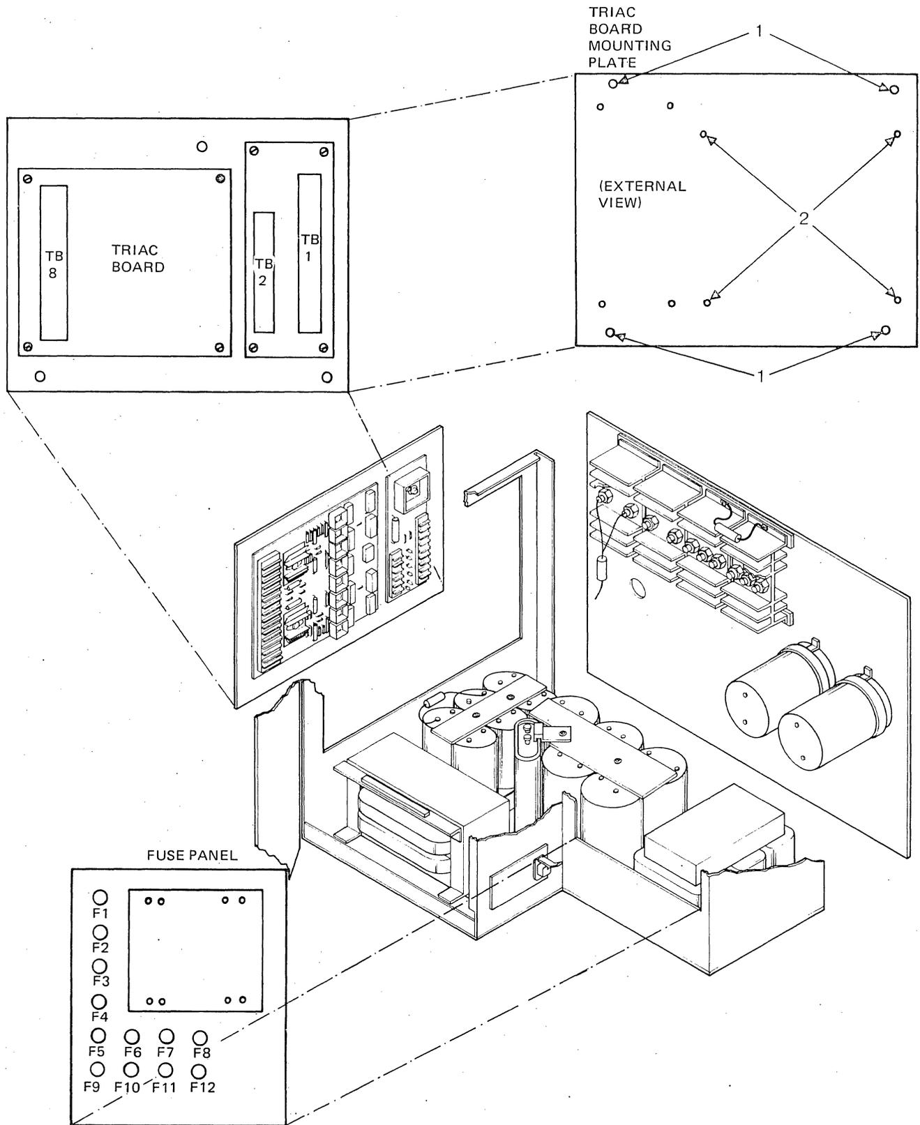
Figure 3-26. TRIAC Board and Fuse Panel
