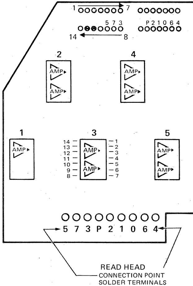
Figure 3-21. R/W Head Amplifier Card
