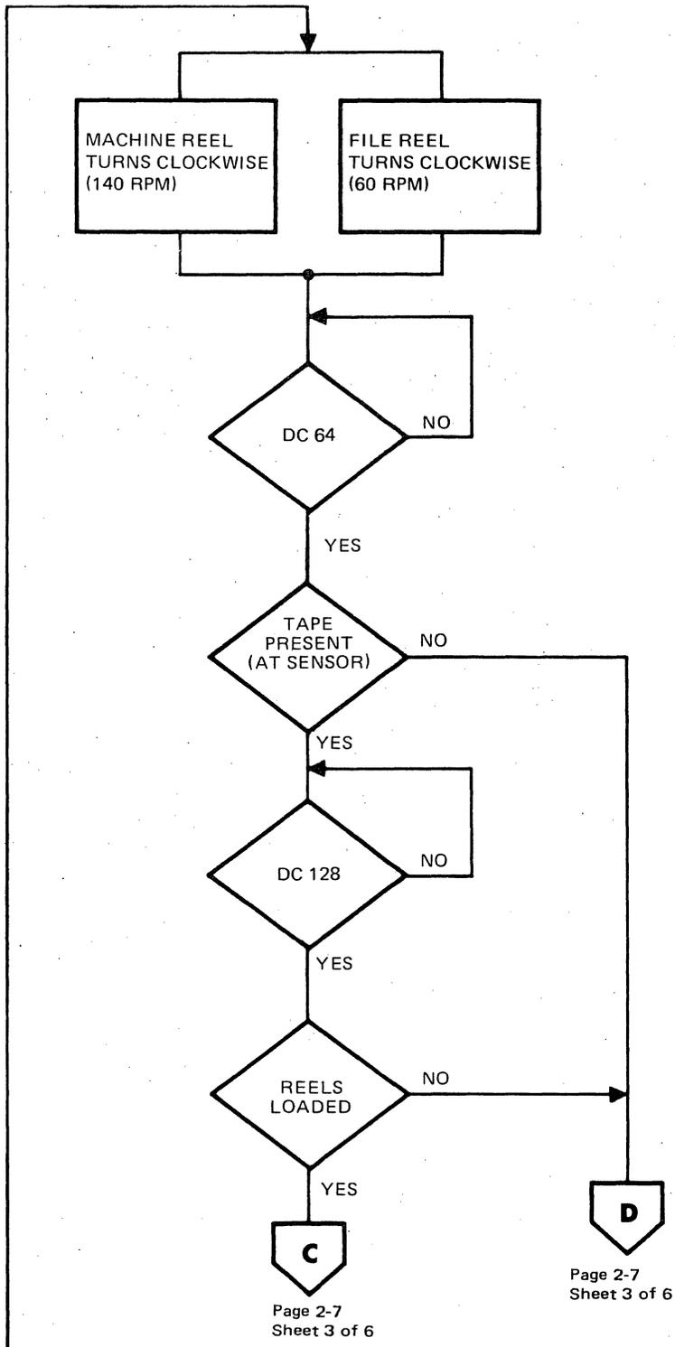
Figure 2-3. Thread/Load Flow Chart (Sheet 2 of 6)
