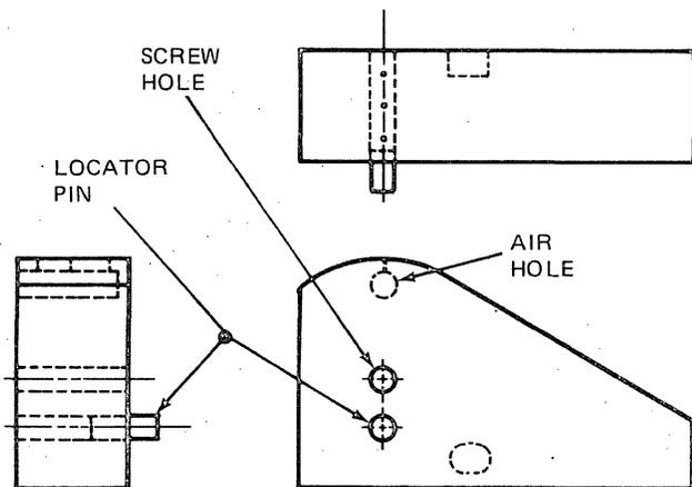
Figure 4-18. Right Guide Assembly PE Only
