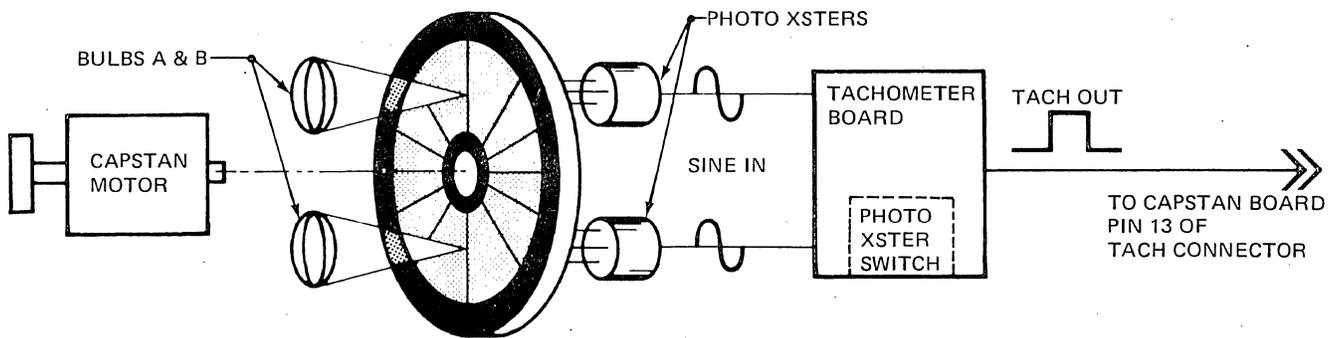
Figure 3-14. Digital Tachometer Configuration
