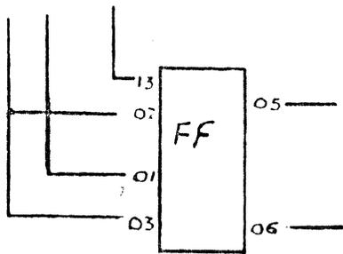
GND on pin 13 resets Latch
