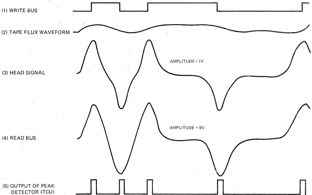
Figure 4-14. NRZI Read Signal Waveforms
