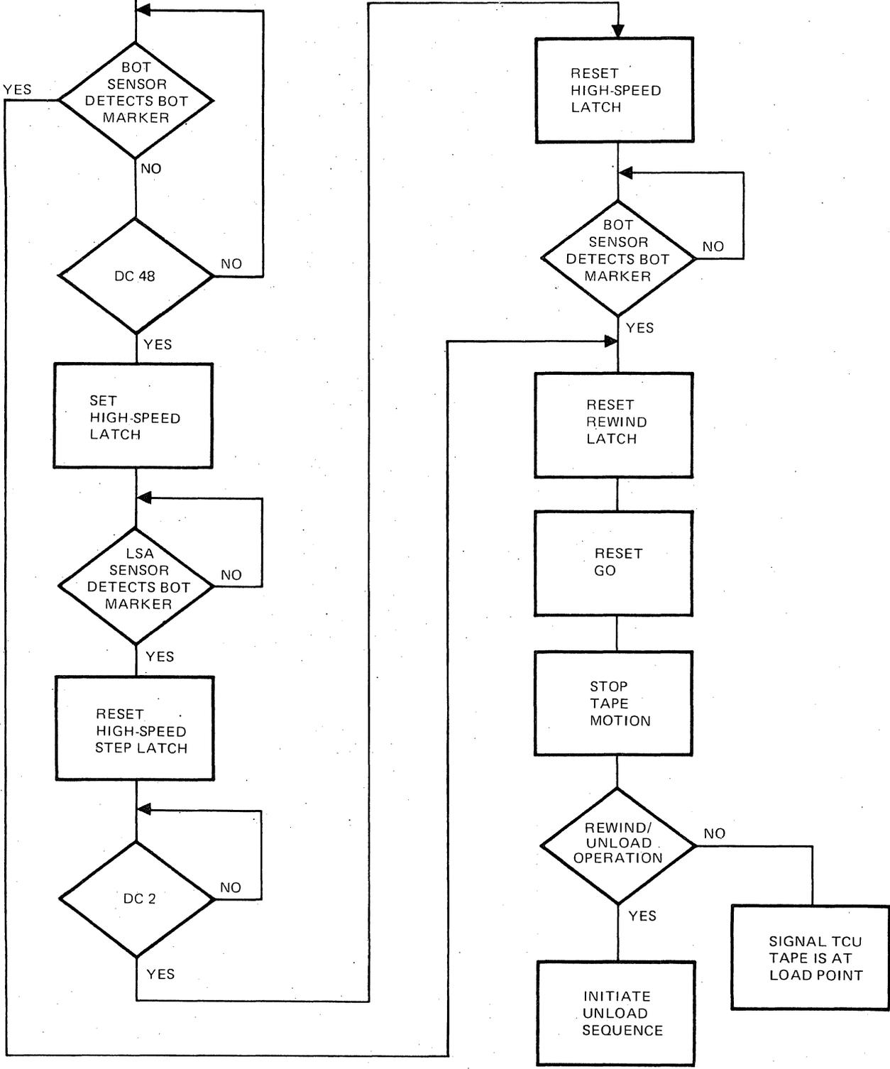
Figure 2-7. Rewind Operation Flow Chart (Sheet 2 of 2)
