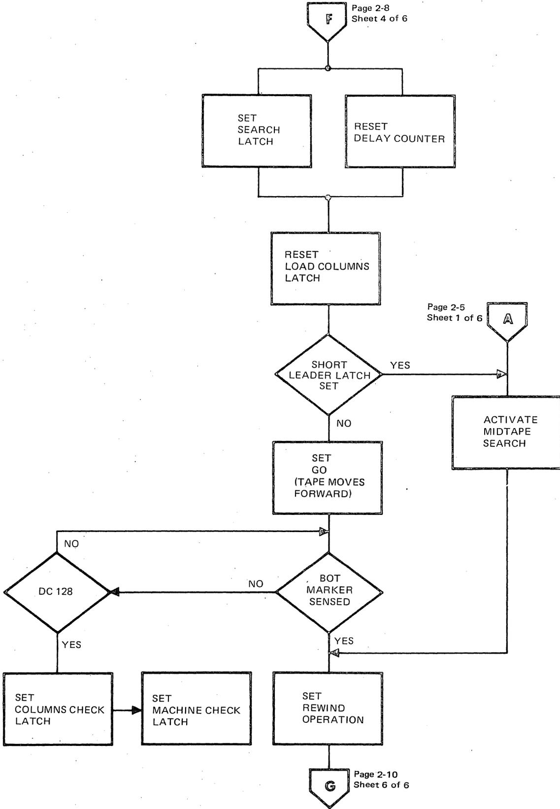
Figure 2-3. Thread/Load Flow Chart (Sheet 5 of 6)
