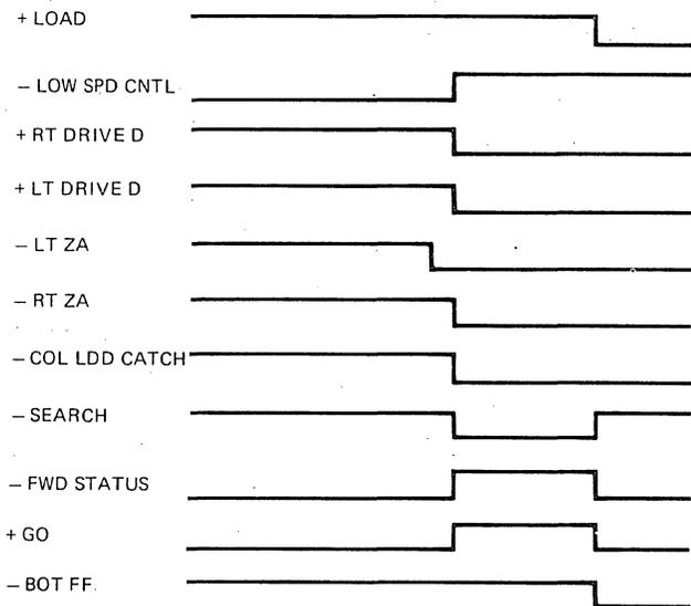
Figure 2-5. Columns Load Sequence Timing Chart
