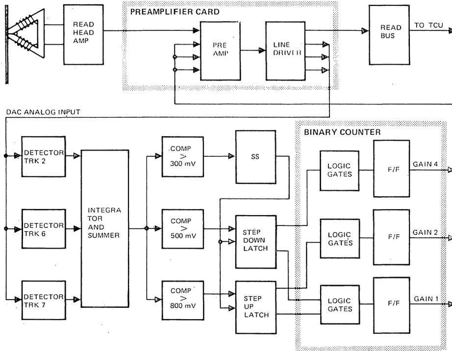
Figure 3-22. DAC Operational Block Diagram
