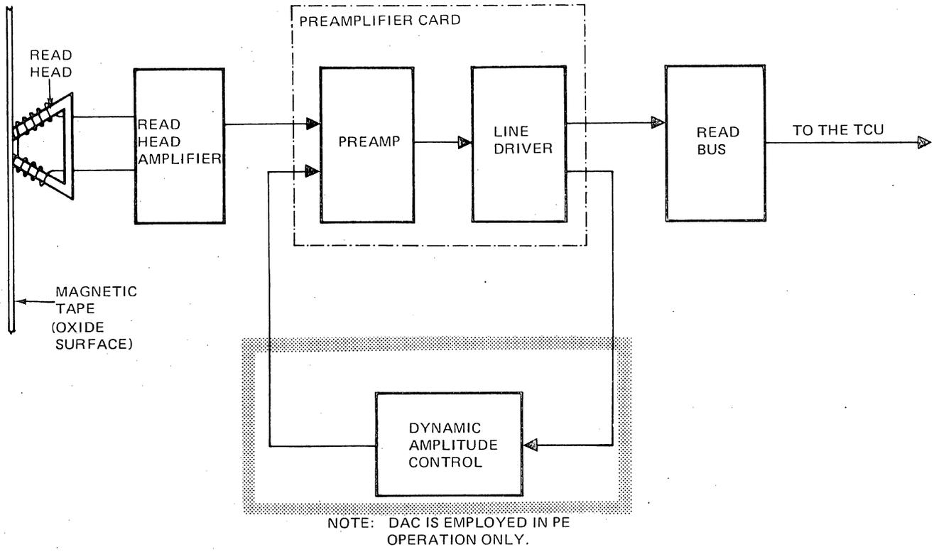
Figure 3-20. Read Circuit Simplified
