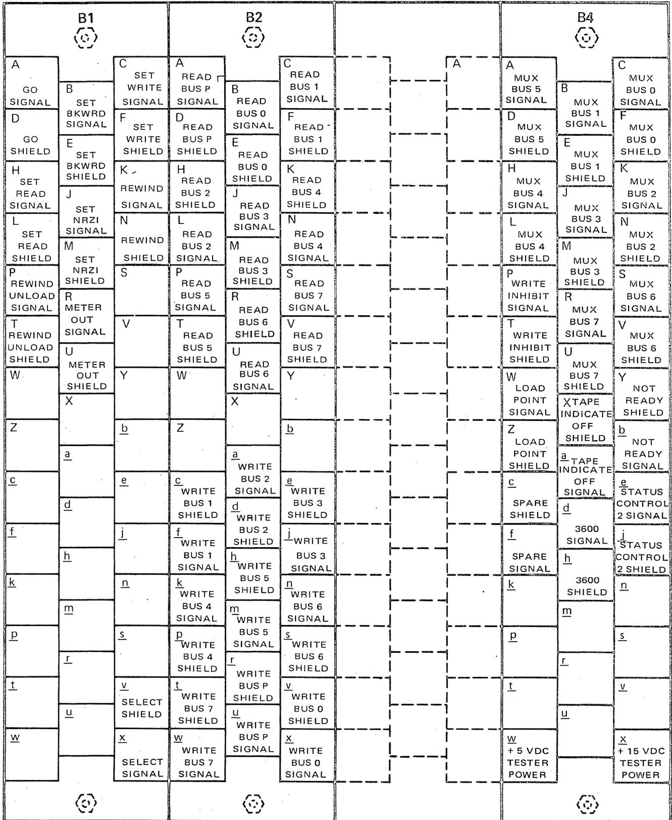
Figure 3-24. Tape Unit I/O Connector (Connector Side)
