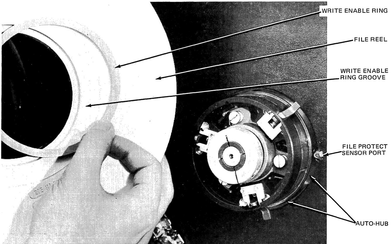
Figure 2-6. Write Enable Ring and File Protect Mechanism
