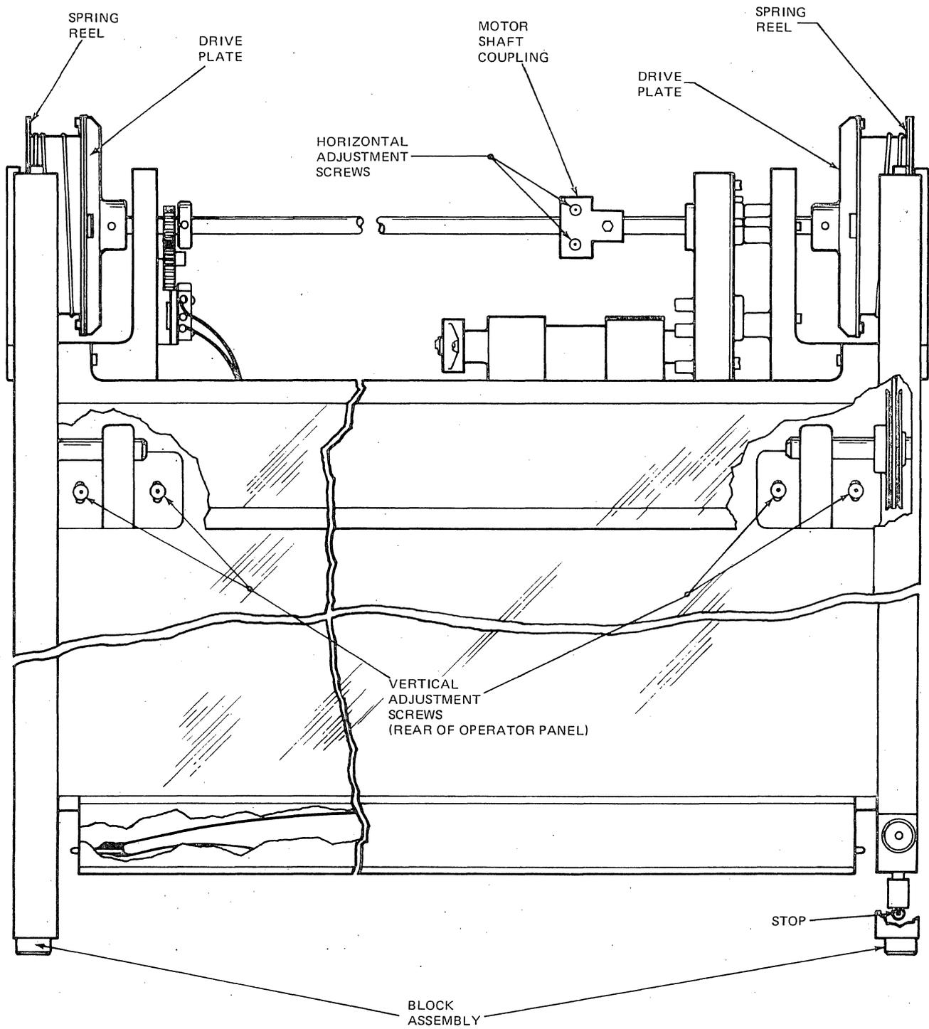
Figure 4-29. Power Window Adjustments
