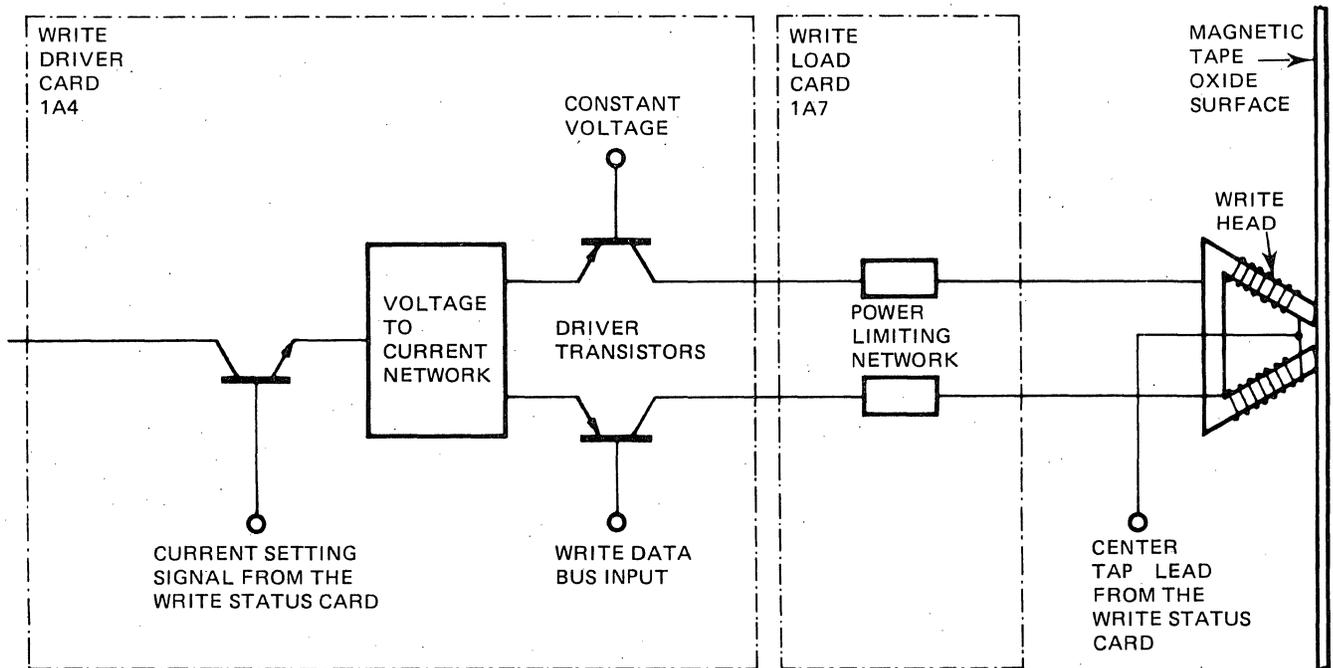
Figure 3-19. Write Driver Simplified
