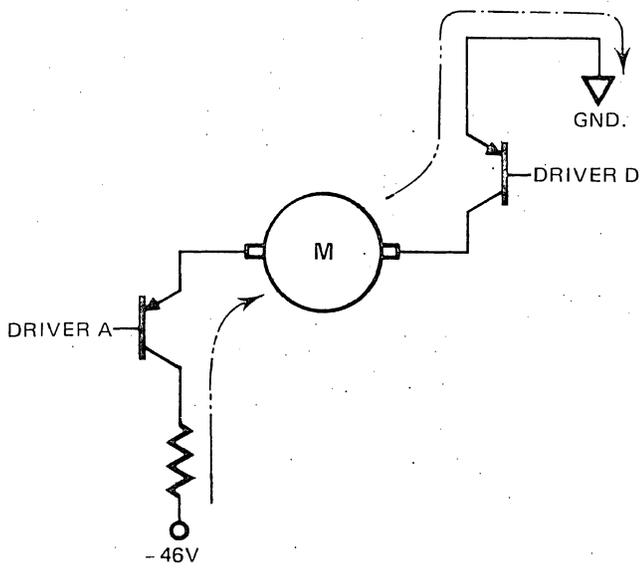
Figure 3-9. Capstan Motor Current Path (Forward Motion)
