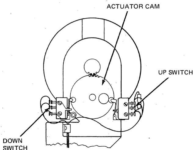
Figure 4-28. Power Window Switches
