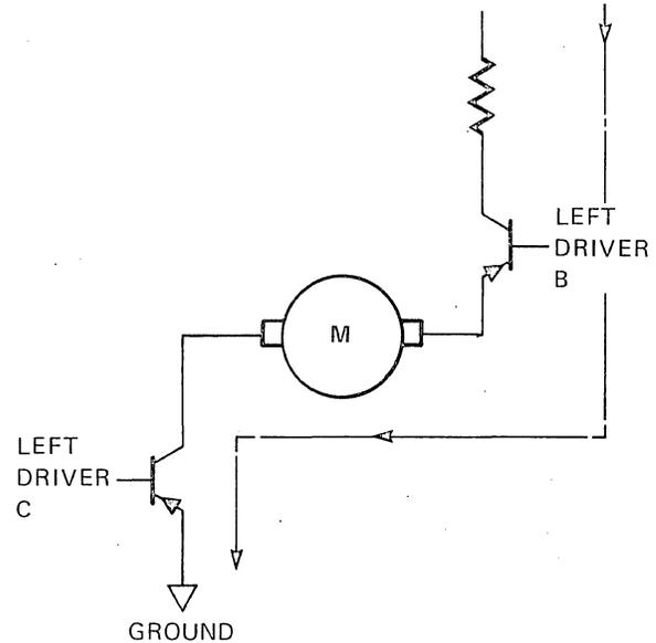
Figure 3-4. Machine Reel Current Path—Forward Motion Left Zone C Violation
