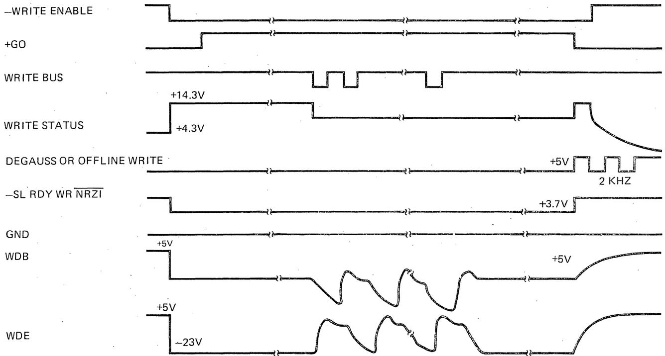
Figure 4-16. Phase Encoded, Write Operation
