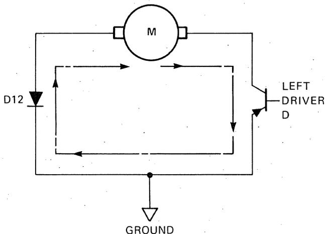
Figure 3-6. Dynamic Brake Current Path (CW Rotation)
