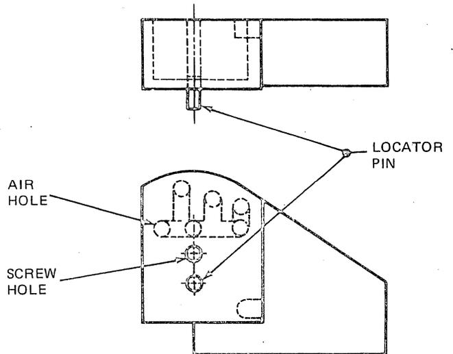
Figure 4-19. Right Guide Assembly 3470 DD Only
