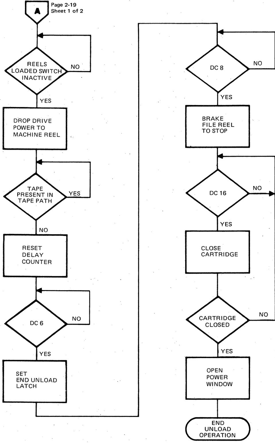
Figure 2-10. Unload Operation Flow Chart (Sheet 2 of 2)
