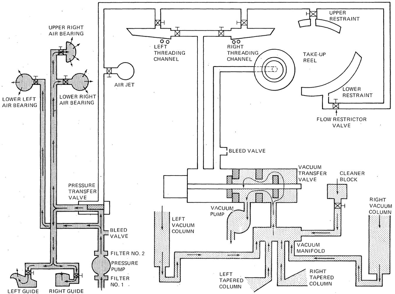
Figure 3-30. Pneumatics, Running Mode
