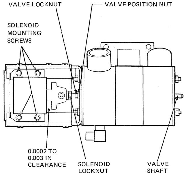
Figure 4-27. Vacuum Transfer Valve
