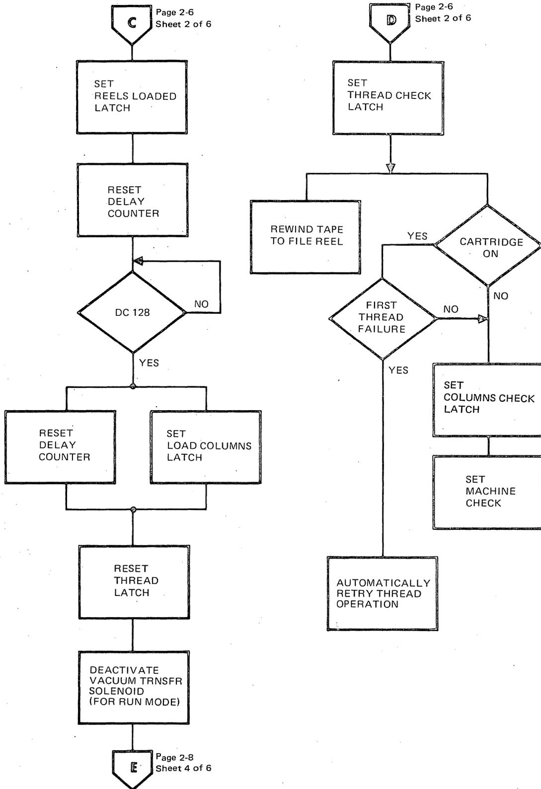
Figure 2-3. Thread/Load Flow Chart (Sheet 3 of 6)
