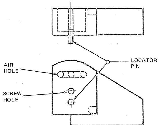
Figure 4-20. Right Guide Assembly (all DD except 3470)
