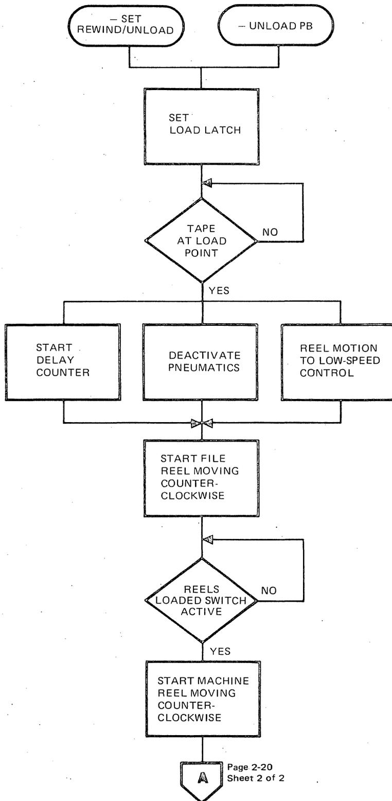
Figure 2-10. Unload Operation Flow Chart (Sheet 1 of 2)
