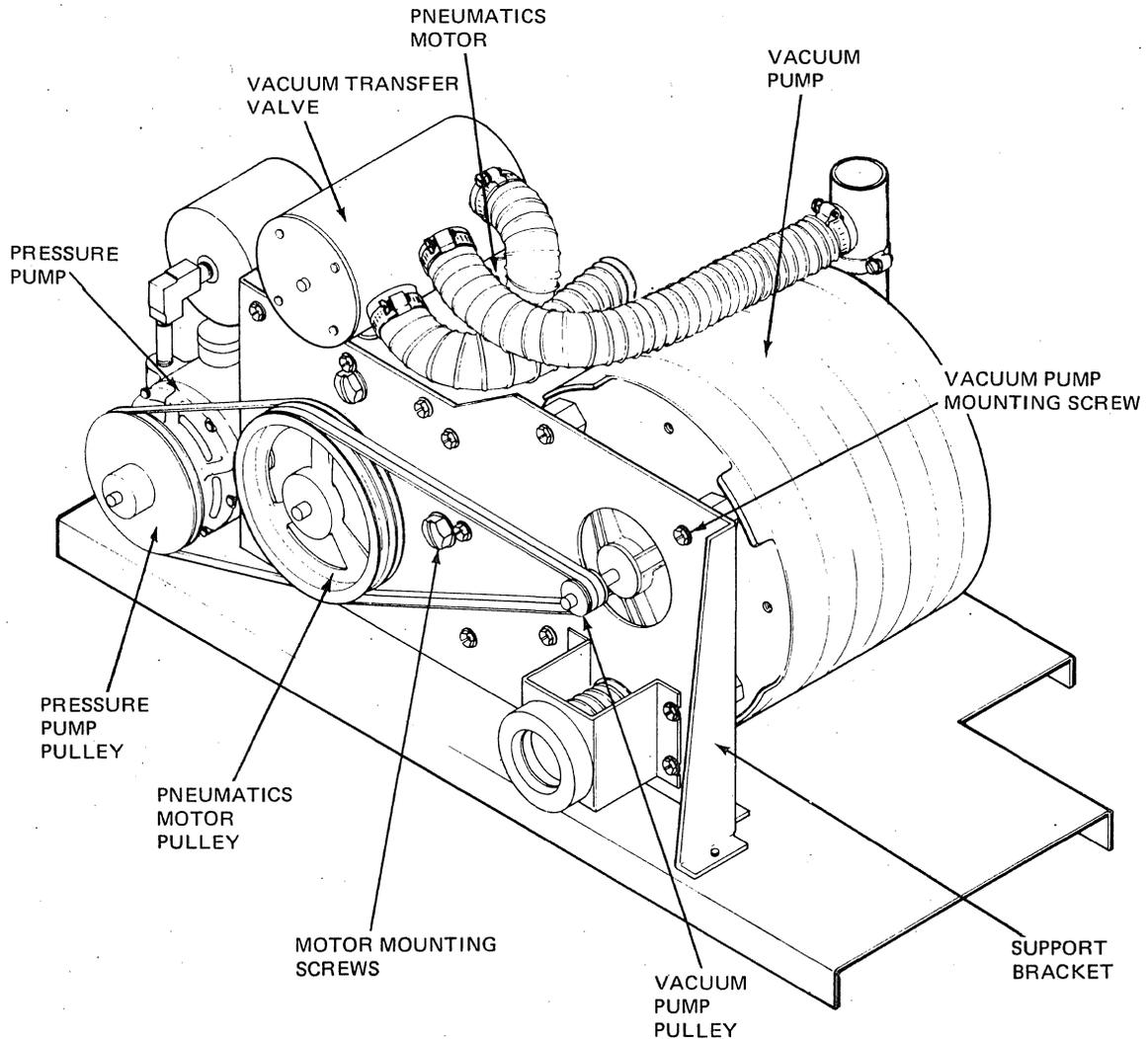
Figure 4-30. Pneumatic Supply Assembly
