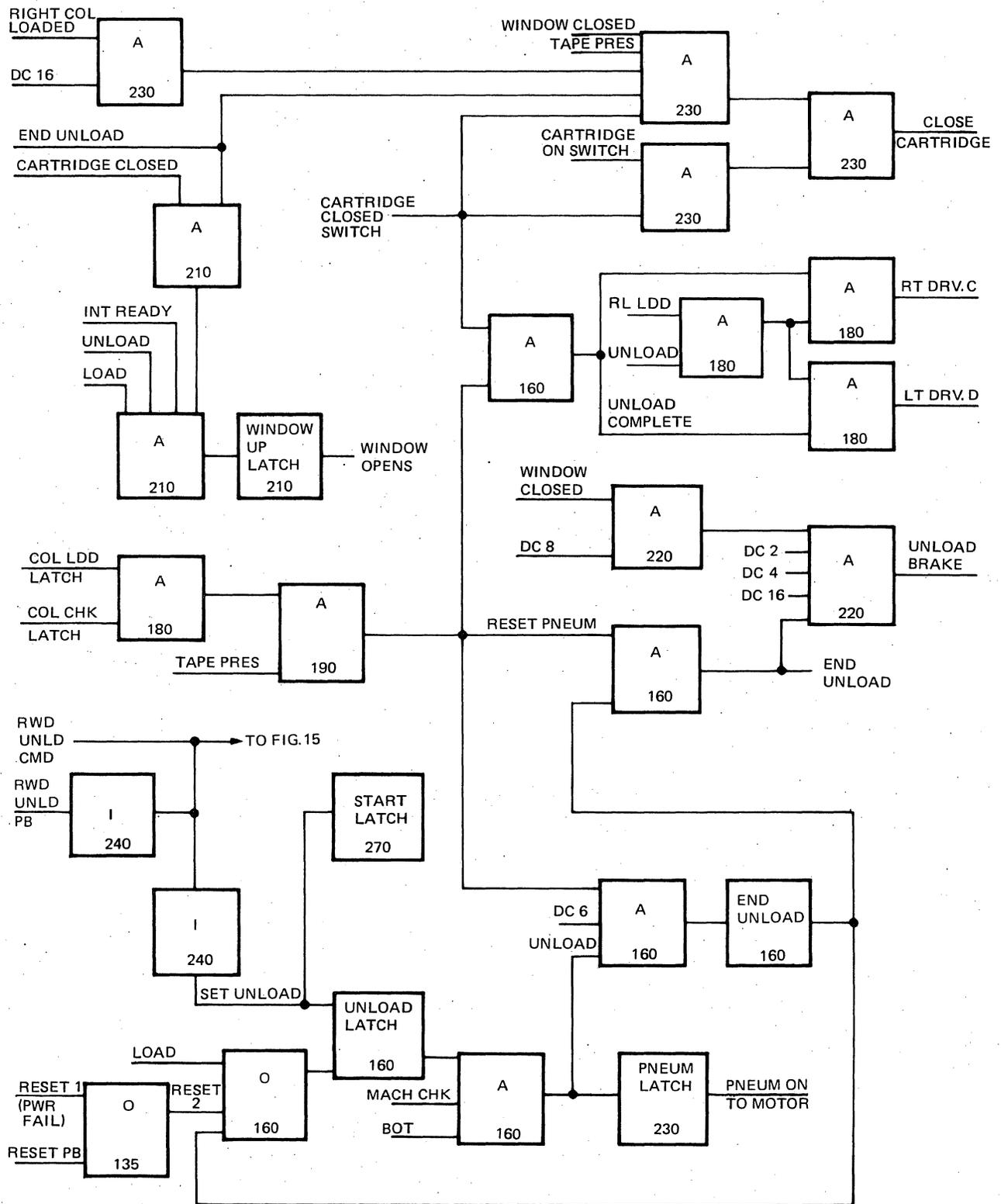
Figure 2-12. Unload Operation Simplified Logic
