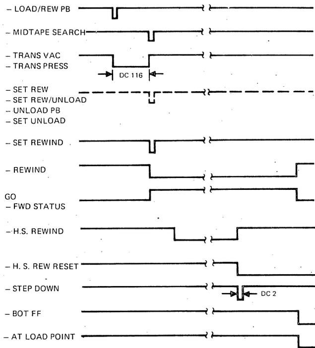
Figure 2-8. Rewind Operation Timing
