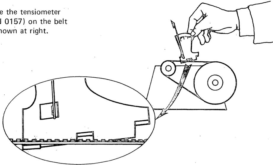
2. With the forefinger on the spring tip, pull the spring in the direction shown at right.
