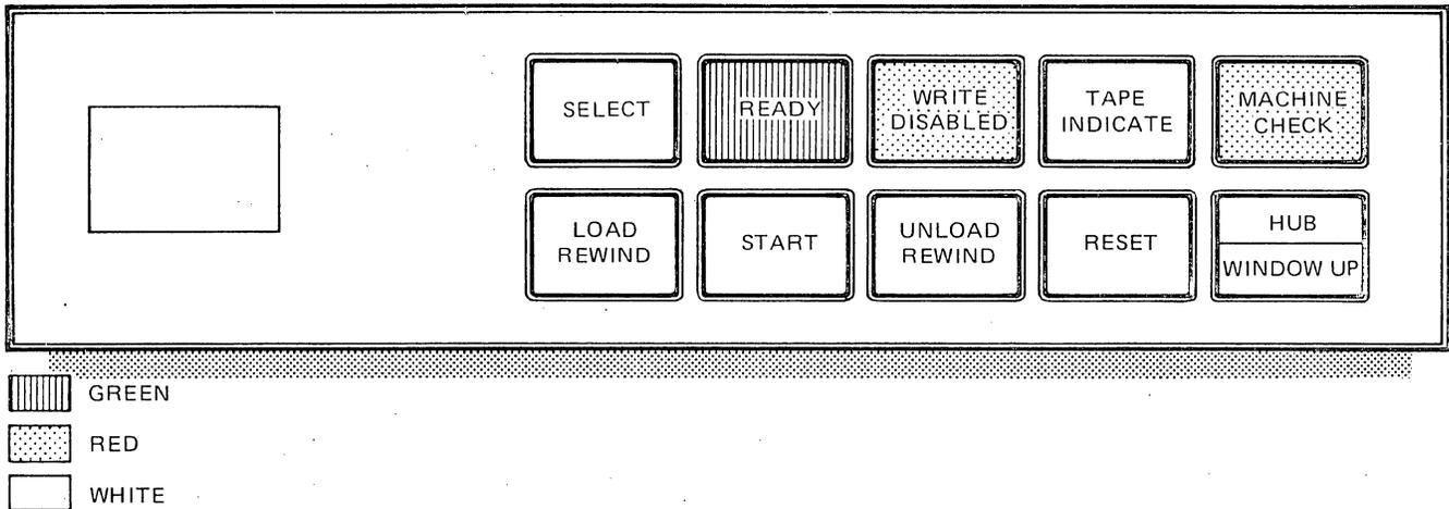
Figure 1-6. Tape Unit Operator Panel
