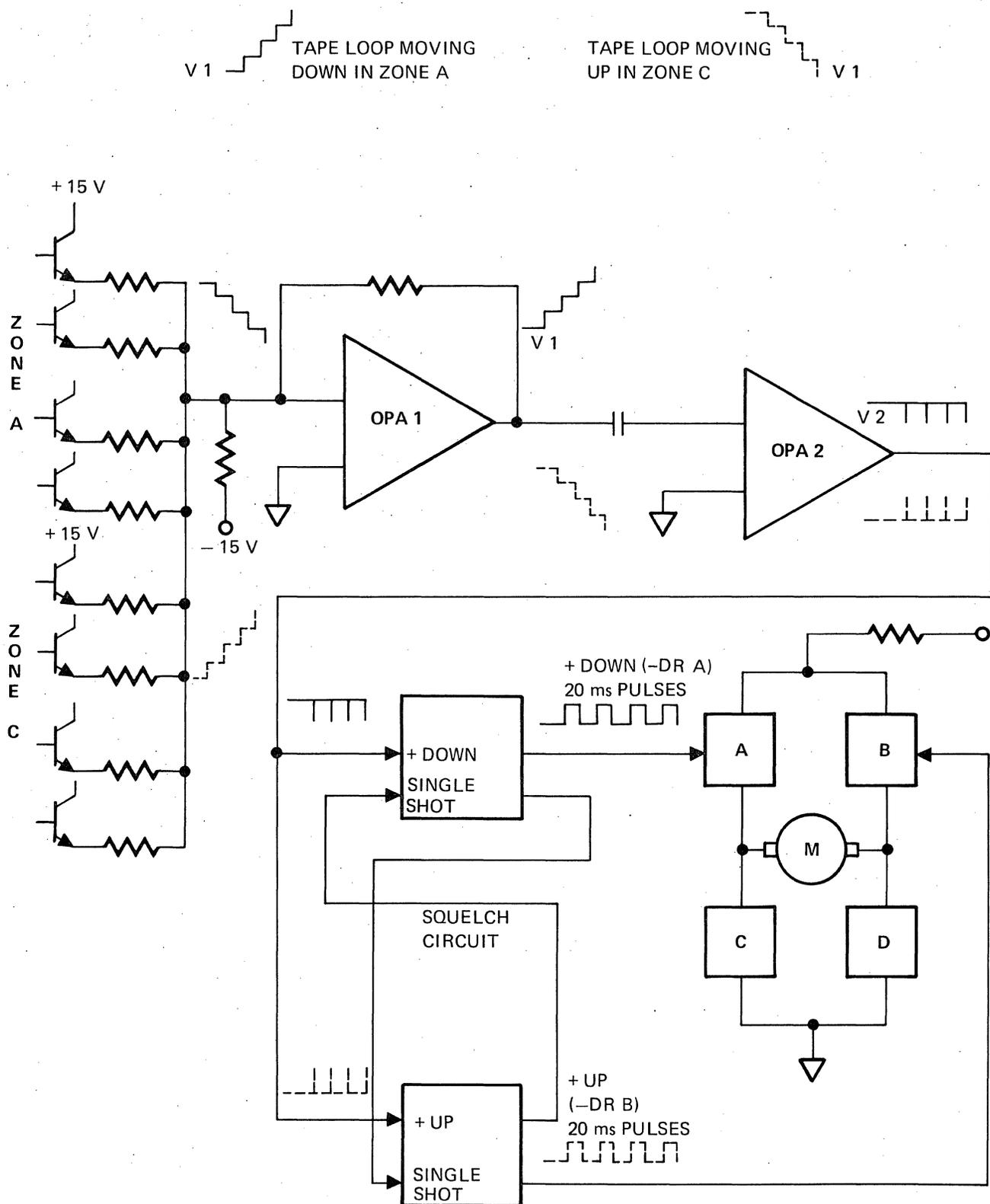
Figure 3-7. Velocity Feedback Control
