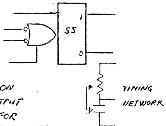
A MINUS SHIFT ON INPUT CAUSES OUTPUT TO GO NEG (AND) FOR DURATION OF SS TIMEOUT THEN RETURNS POSITIVE
