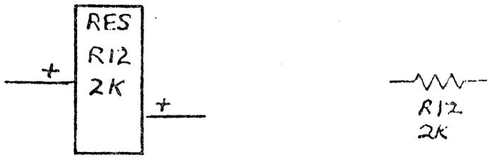
NOTE: Line from lower half of Block means Non-Inversion of input.
