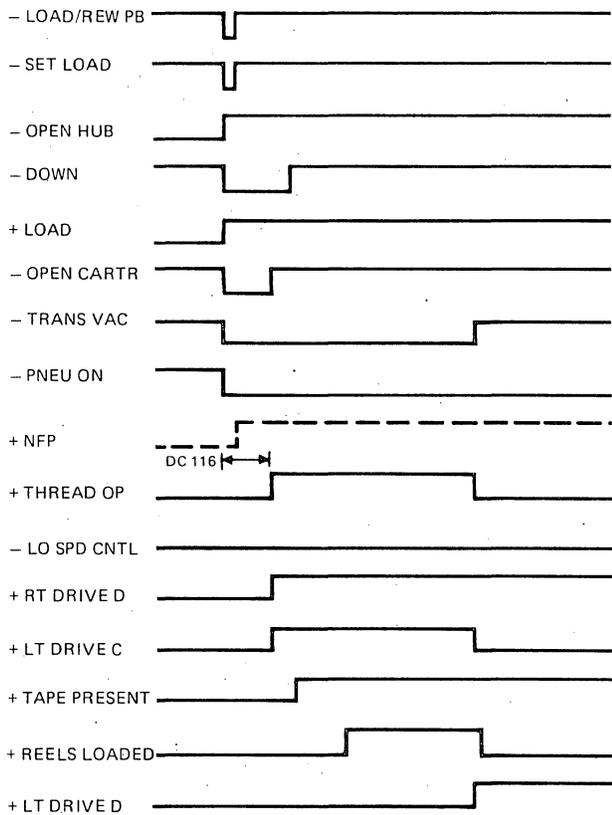
Figure 2-4. Thread Sequence Timing Chart
