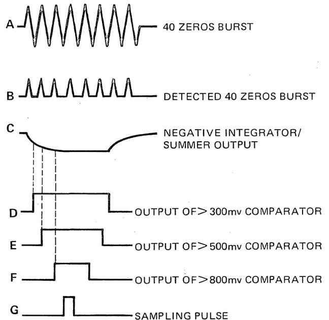
Figure 3-23. DAC Operation Waveforms
