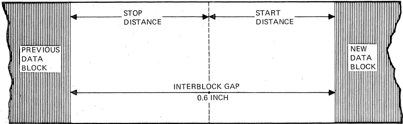
Figure 3-16. Interblock Gap Diagram
