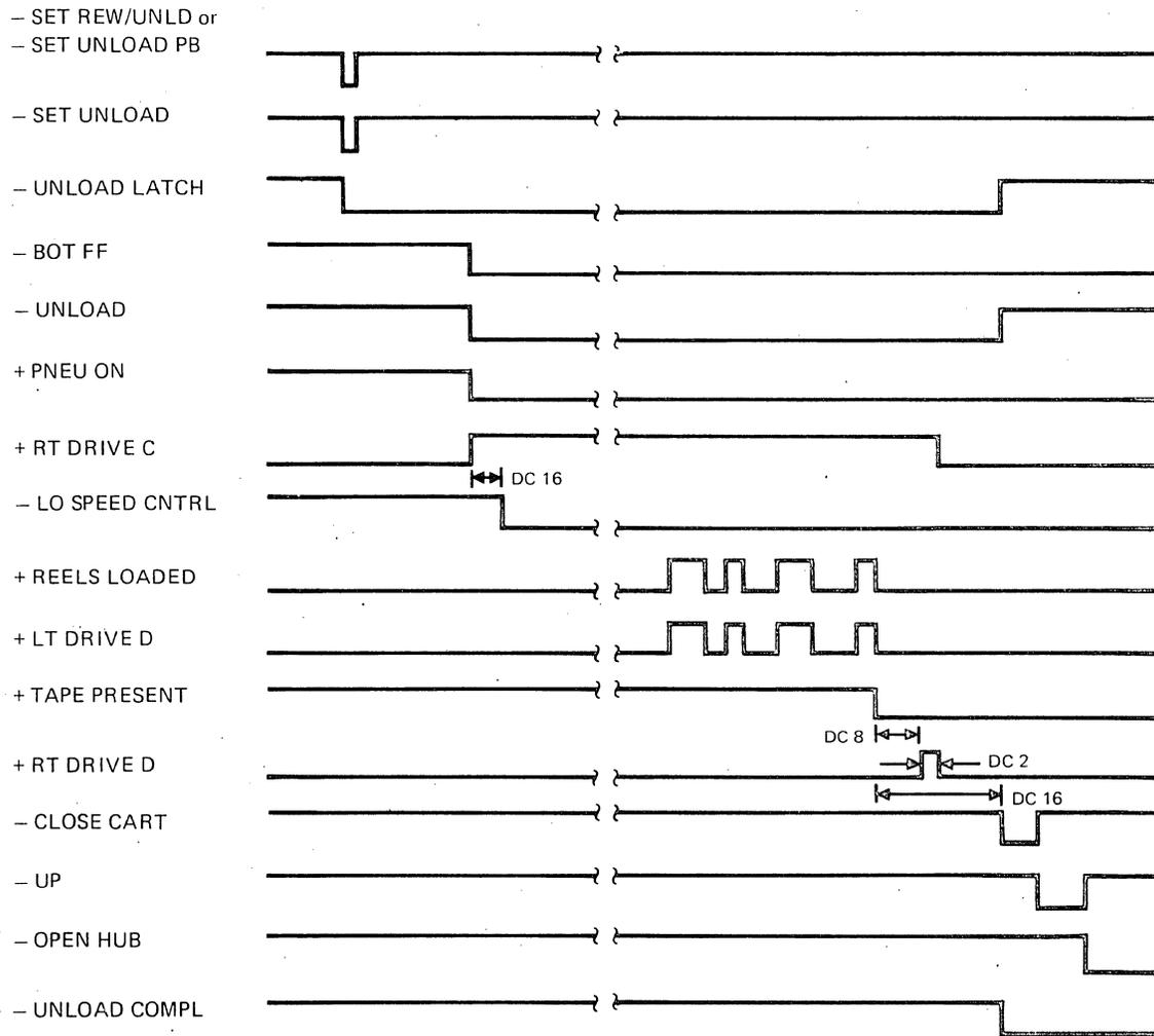
Figure 2-11. Unload Operation Timing
