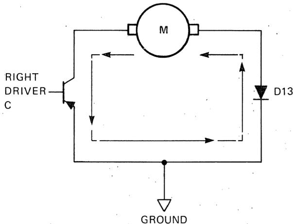
Figure 3-5. Dynamic Brake Current Path (CCW Rotation)
