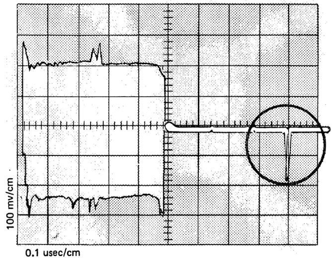
Figure 4-9. Erase Head Polarity Pulse
