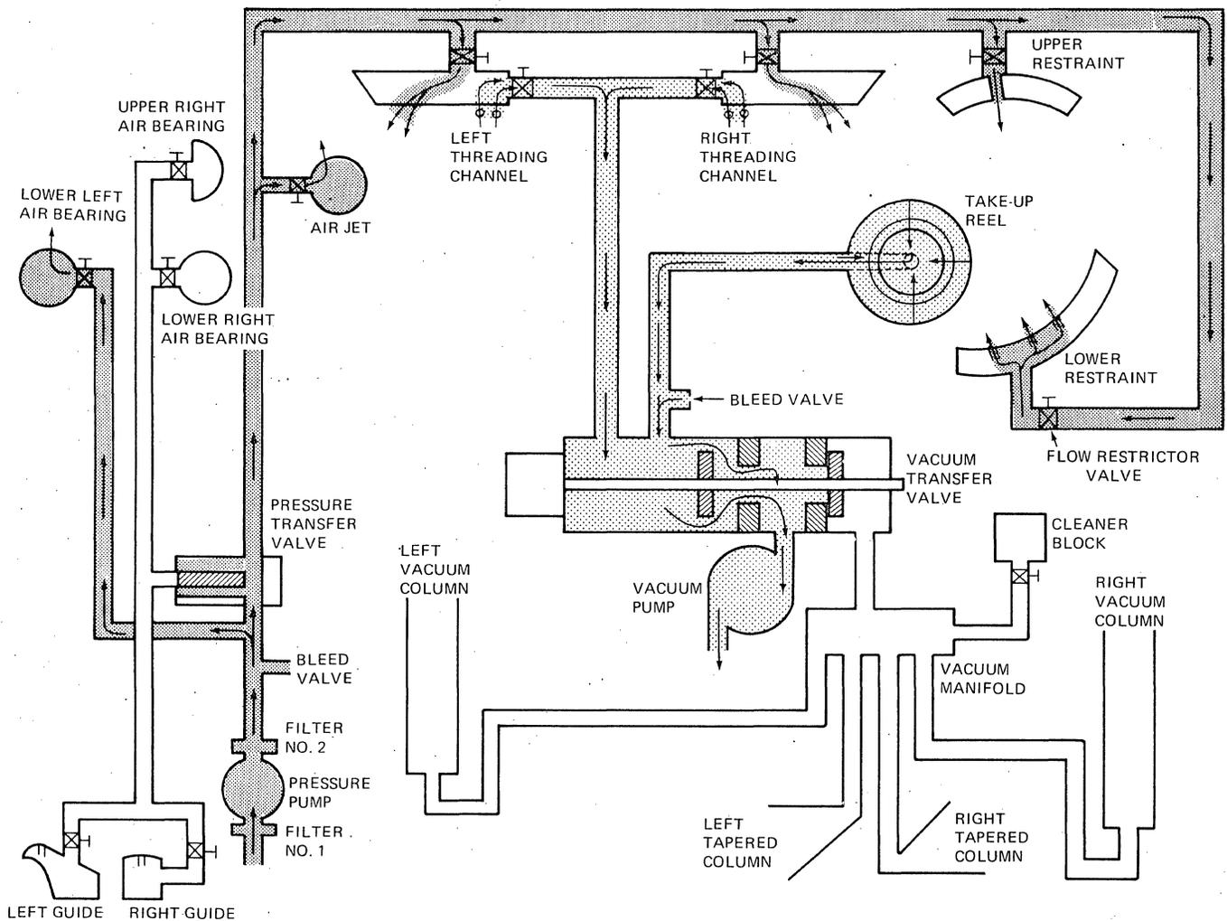
Figure 3-29. Pneumatics, Threading Mode
