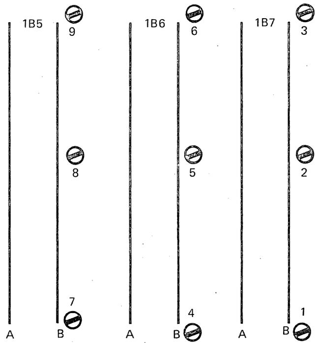
Figure 4-25. NRZI Write Amplitude Adjustment Potentiometers by Track Location
