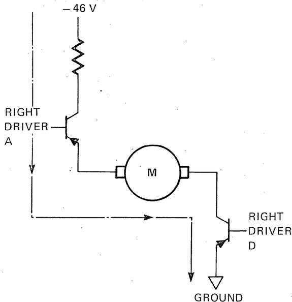
Figure 3-3. File Reel Current Path—Forward Motion Right Zone A Violation
