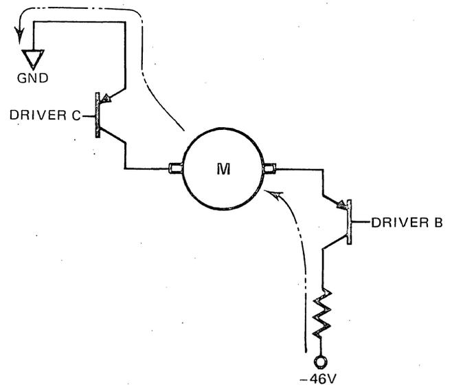
Figure 3-10. Capstan Motor Current Path (Backward Motion)
