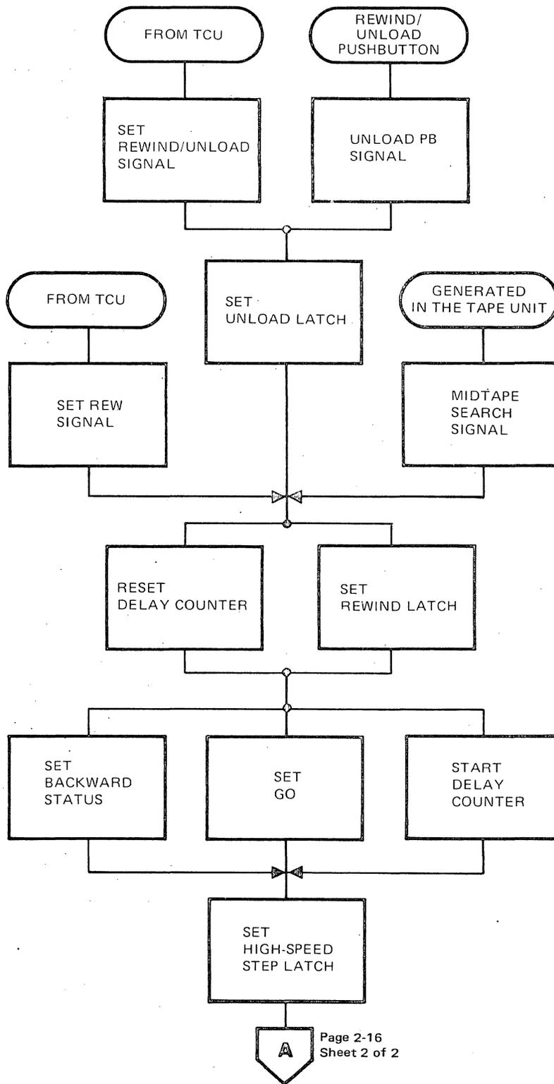
Figure 2-7. Rewind Operation Flow Chart (Sheet 1 of 2)
