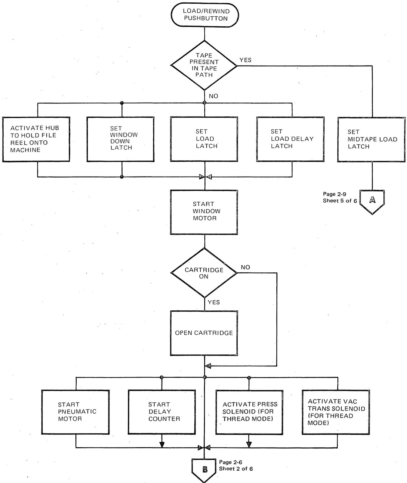
Figure 2-3. Thread/Load Flow Chart (Sheet 1 of 6)
