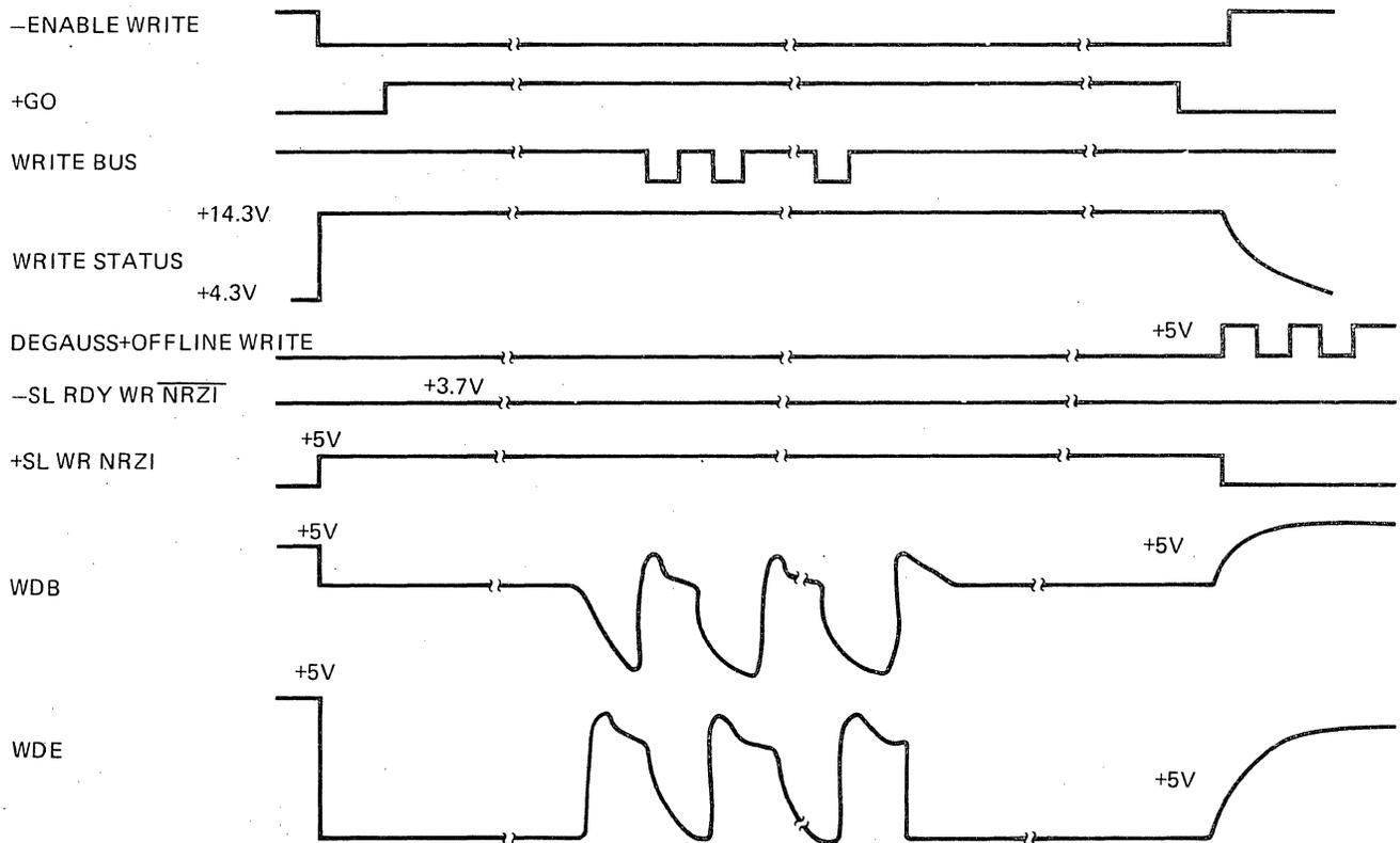
Figure 4-17. NRZI, Write Operation
