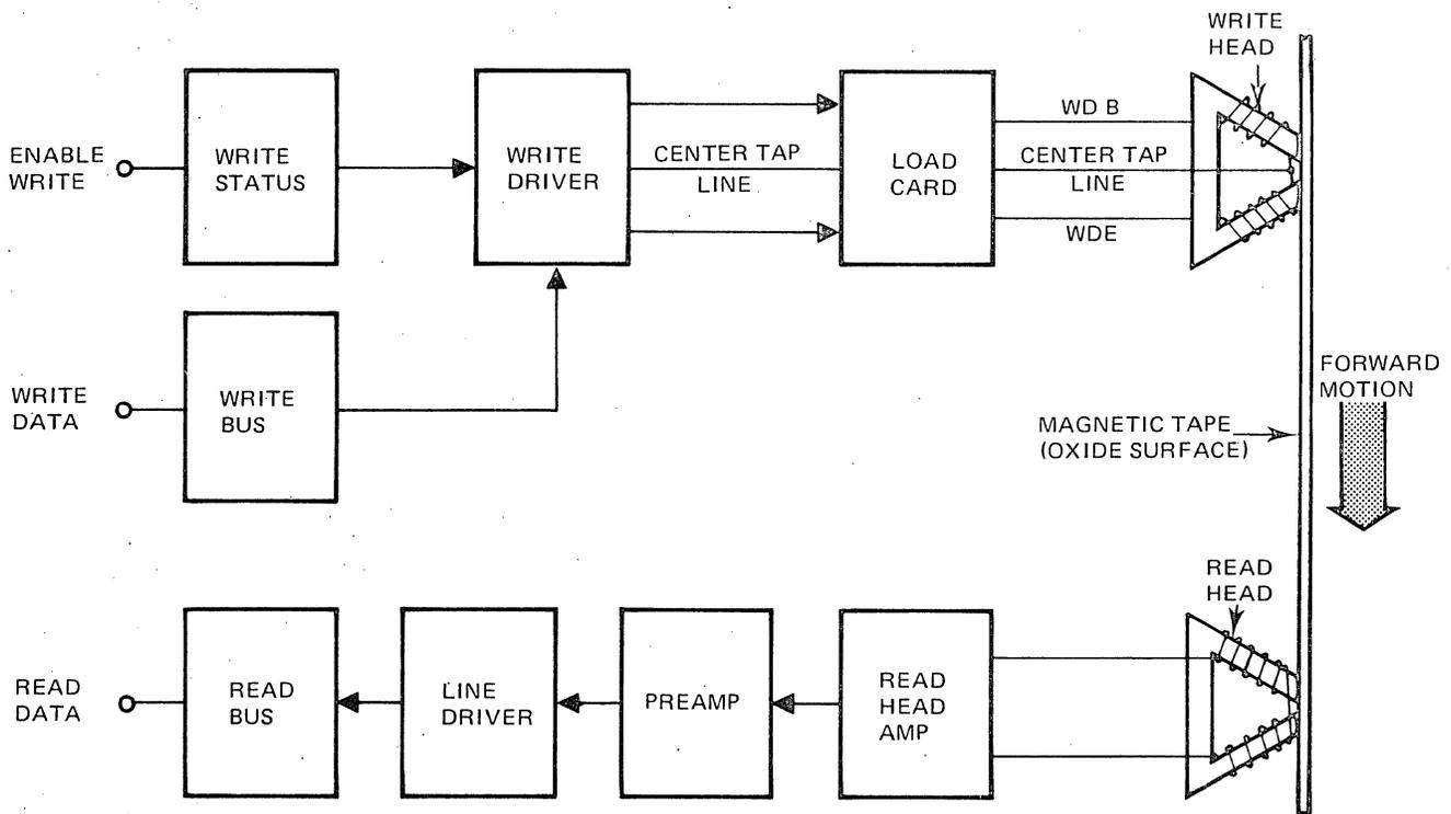
Figure 3-18. Read/Write Block Diagram
