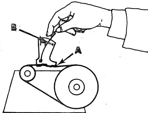
3. When the right hand tab of the Tensiometer just touches the top of the belt (A), read the belt tension (on the left edge of the spring) in pounds on the scale (B).
