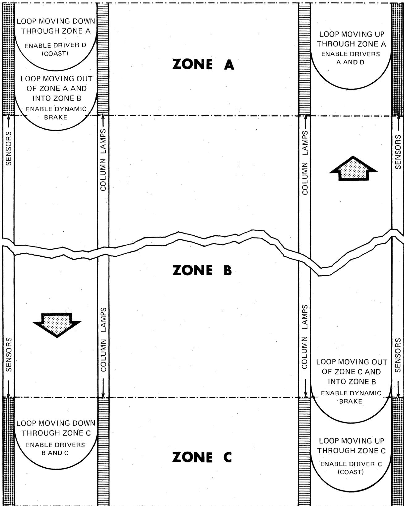
Figure 3-2. Column Sensors and Zones
