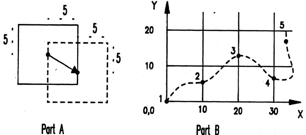
The five points collected in part B are numbered in order. The set increment distance equals 10.
