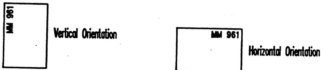
On the 961, the tablet's orientation is vertical on power-up or Reset. Send an ASCII b to set the orientation to horizontal; send an ASCII c to re-orient the tablet vertically.
