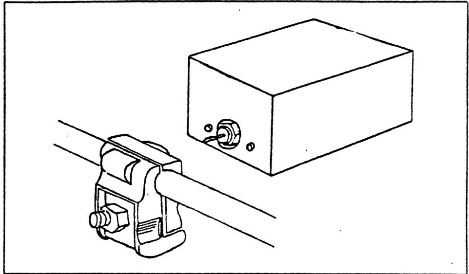
8. Carefully insert the stinger housing, on the transceiver box, into the hole in the tap block. Screw the transceiver into the tap block until the O-ring is seated. Do not overtighten the transceiver.
