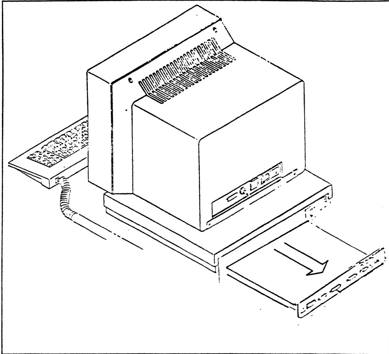
Figure 3-3 *Removing Rear Panel Assembly from Chassis*
