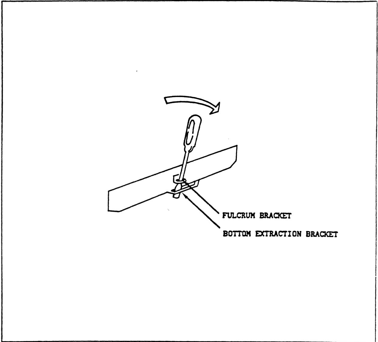
Figure 3-2 *Releasing Backplane Connectors*
