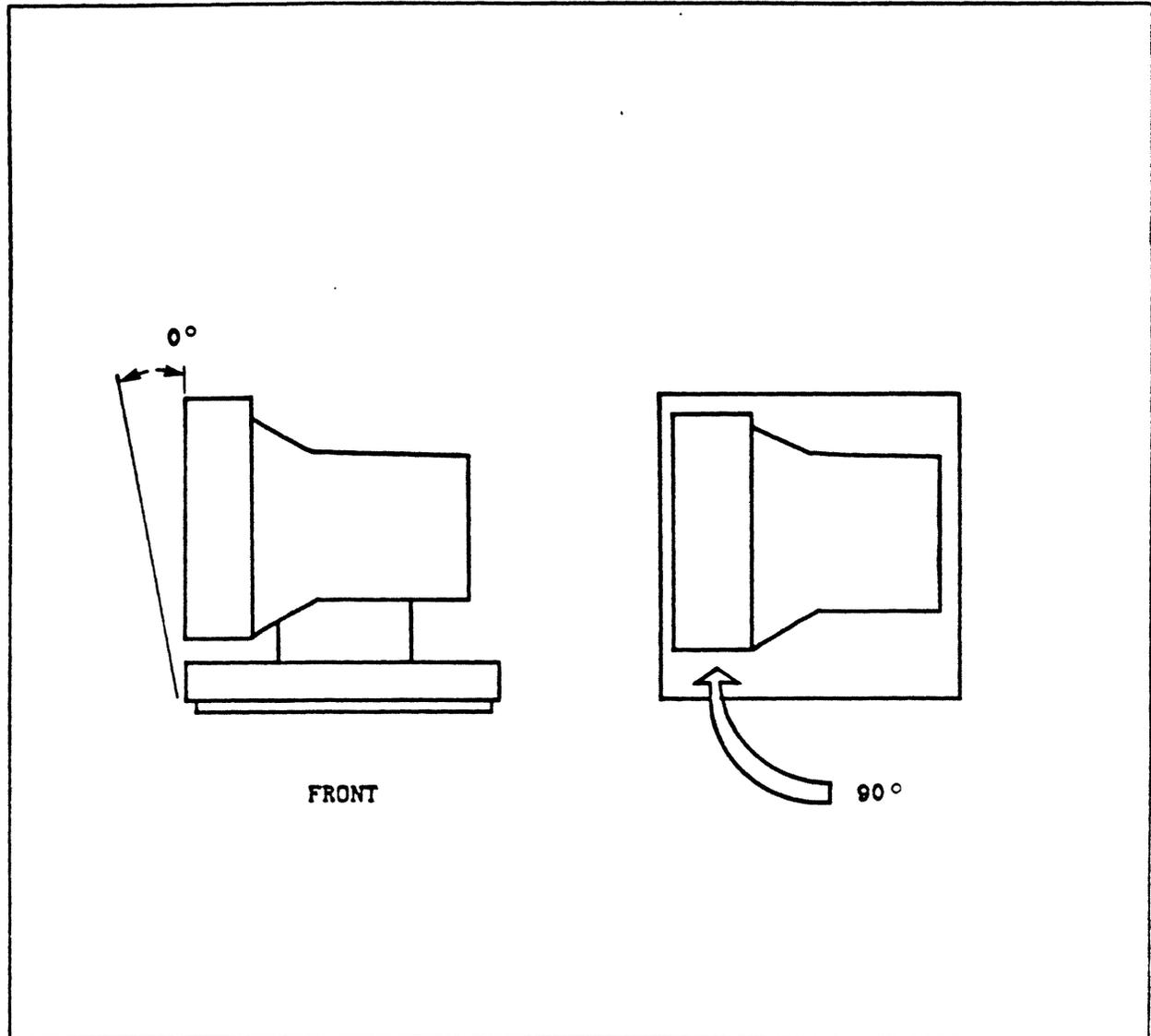
Figure 3-5 *Positioning Monitor for Removal*
