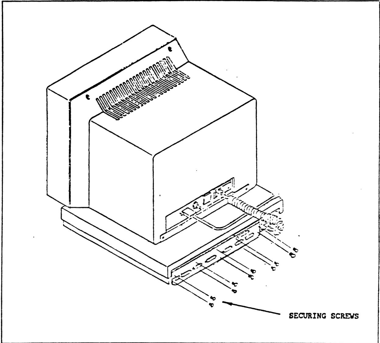
Figure 3-1 *Rear Panel Securing Screws*
