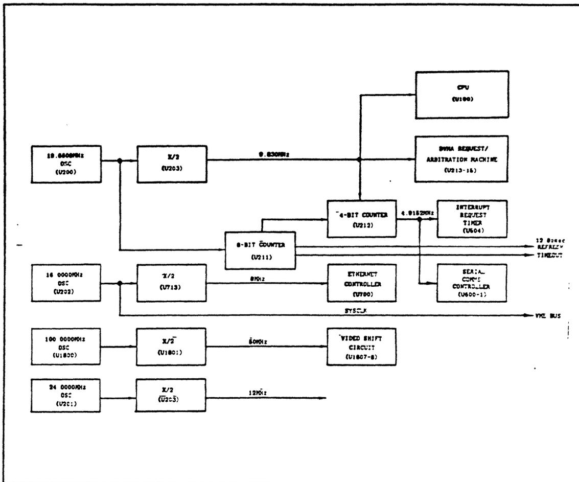
Figure 1-4 Clock Circuits
