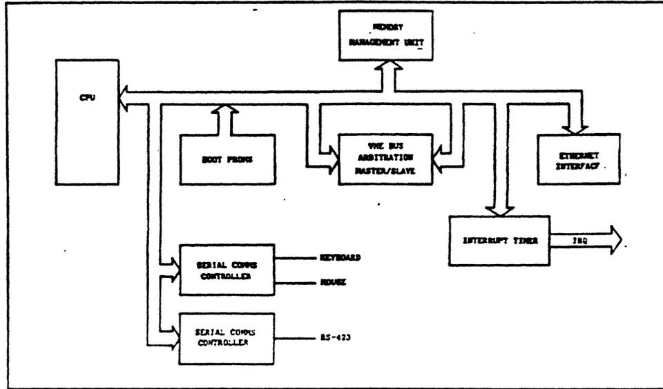
Figure 1-7 I/O Data Bus
