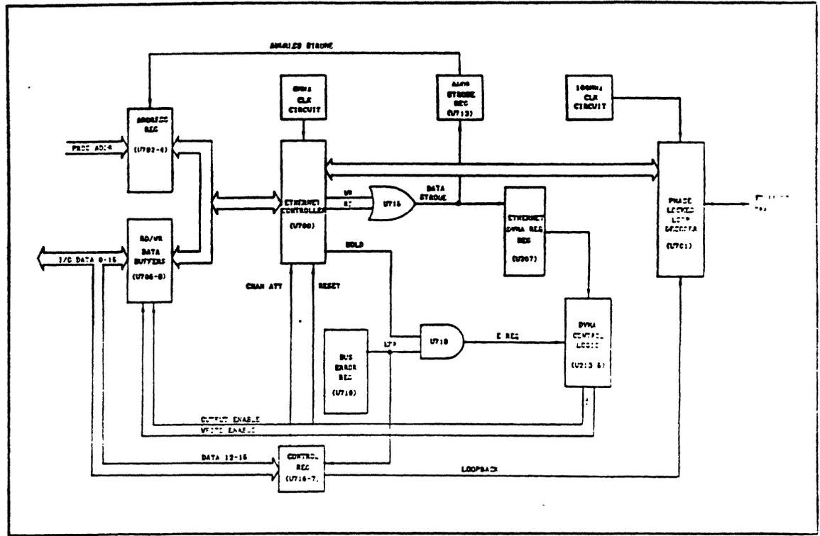
Figure 1-15 Ethernet Interface logic
