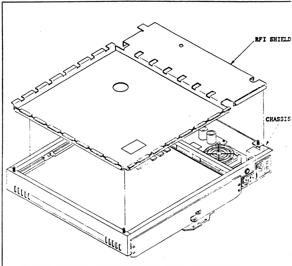
Figure 3-7 *RFI Shield Removal*
