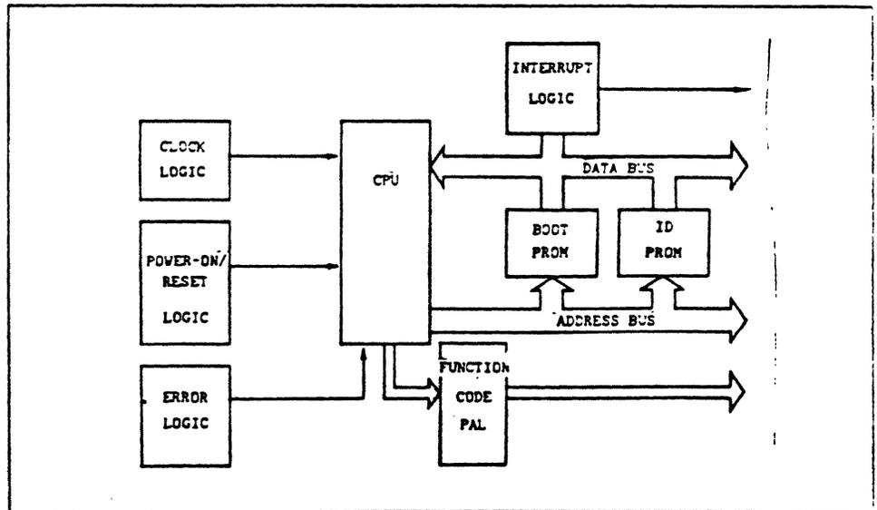
Figure 1-2 CPU Logic
