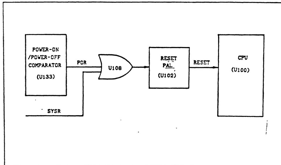
Figure 1-3 Power-on/Reset Logic
