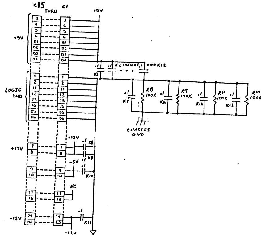
P1 MULTIBUS CONNECTIONS - 15 SLOT
