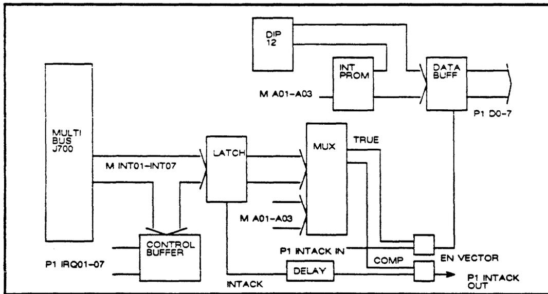
FIGURE 7C-5: INTERRUPT LOGIC
