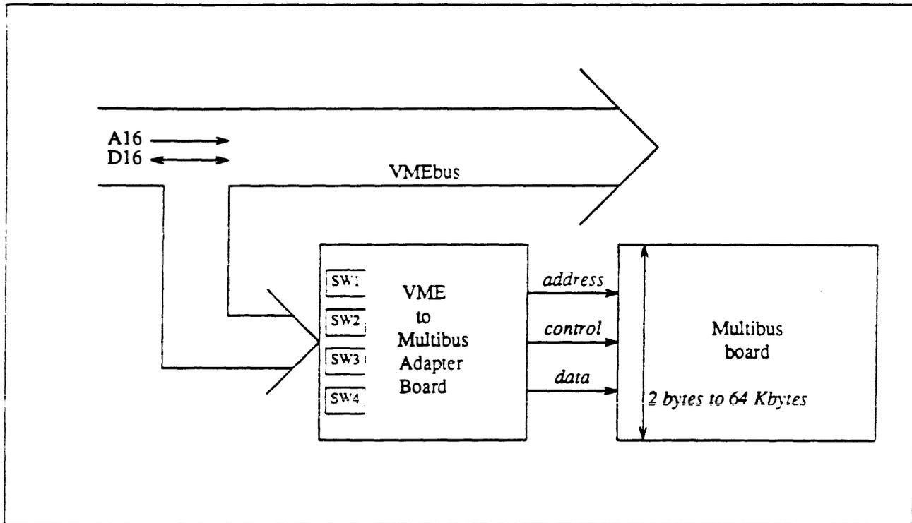
The size of the block of addresses can be any power of 2 between 2 to the 1st power and 2 to the 16th power (2 bytes to 64 Kbytes). The starting address of the block can be any address which is a multiple of the size of the block. Another way of saying this is that any VME address bit between A1 and A15 can either be ignored or compared against a switch section.
