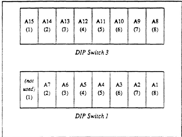
A switch section ON causes a match when the corresponding VME address bit is 0.
