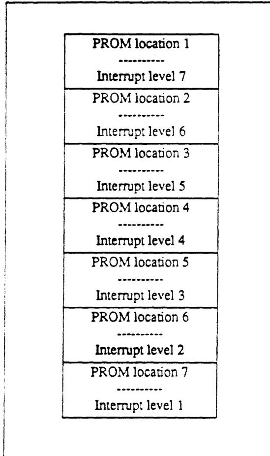
If the switch is used to set the interrupt vector, the Interrupt Vector PROM must NOT be installed in its socket. If the PROM is used to set the interrupt vector, all the switch sections in DIP 12 must be set to OFF.
