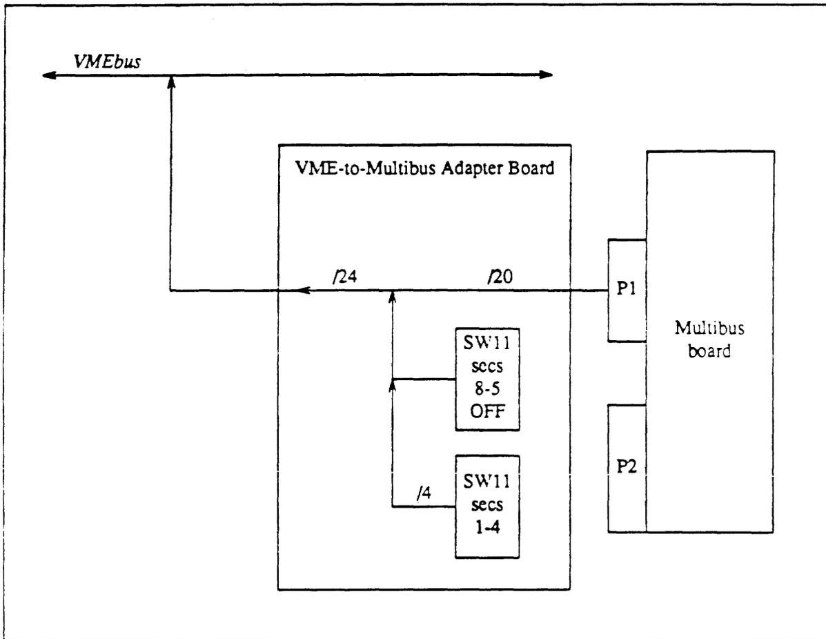
In this case, sections 5-8 of DIP switch 11 must be set OFF, to isolate the Multibus P2 connector, and the necessary four high-order address bits must be set into sections 1-4 of DIP switch 11.
