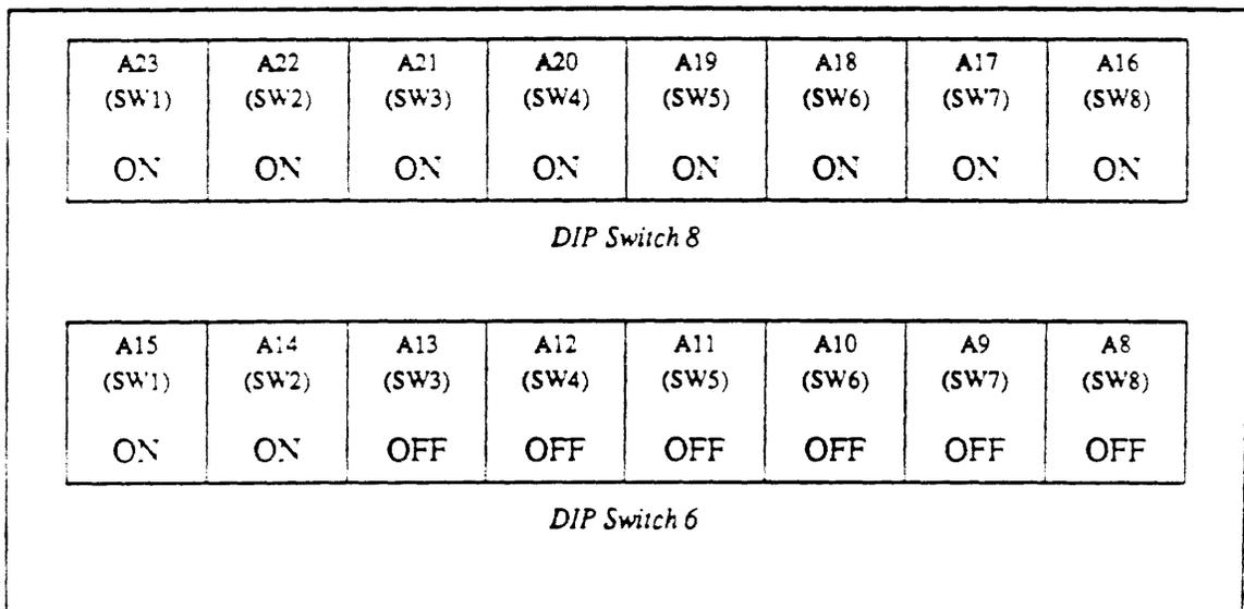
Here's the switch section settings for the various block sizes available in the Multibus memory space.
