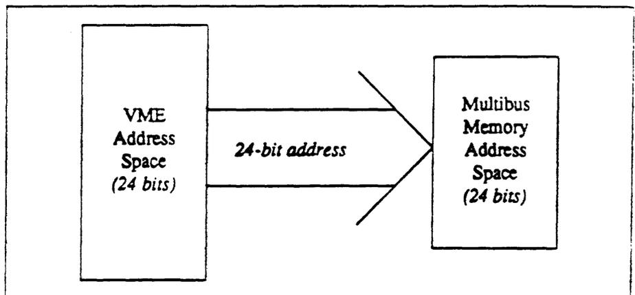
This addressing function is controlled by the DIP switches (DIPs 5, 6, 7, 8) which set up in two 8-bit equal-to-comparators (U201, U202). If the comparators
