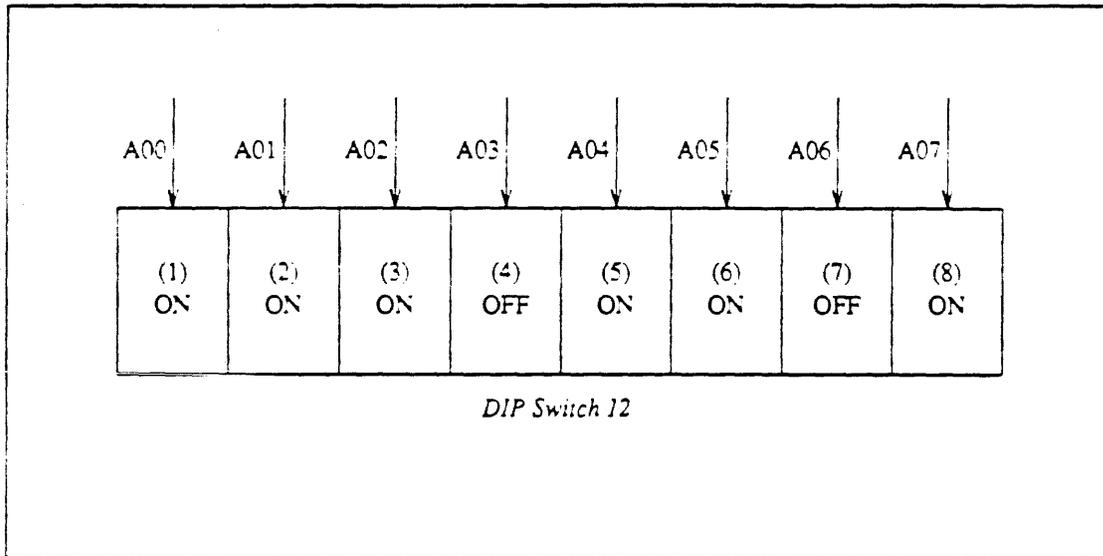
**NOTE** The VME interrupt vector number is the 68000 vector address divided by 4. Thus VME vector 0x48 causes the 68000 to fetch its interrupt vector from memory location  $0x48 * 4 = 0x120$ .
