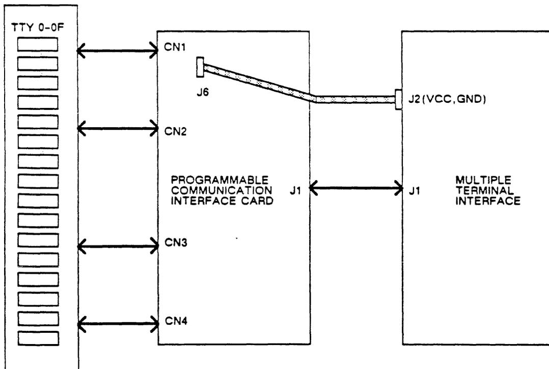
FIGURE 7C-14: PROGRAMMABLE COMMUNICATION INTERFACE (SECOND ALM BOARD)
