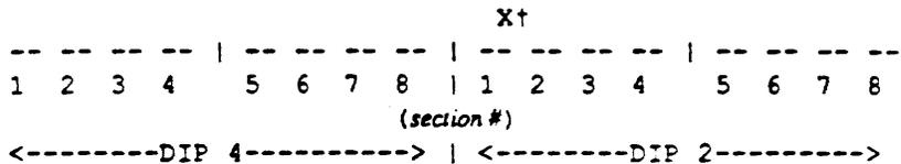
†Remember, address bit A0 is not set into this DIP switch.
