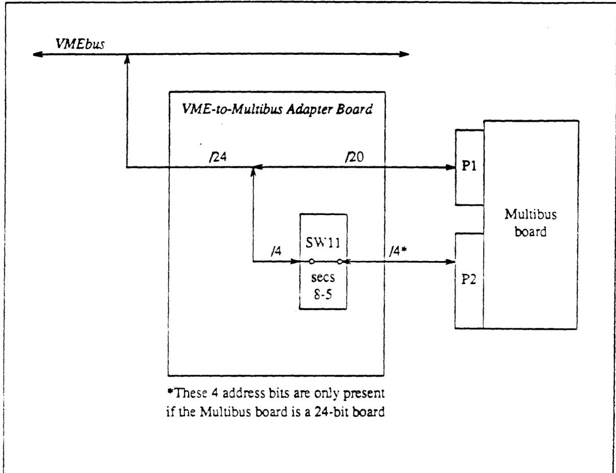
DMA Transfer Address—DIP Switch 11, Sections 1-4
