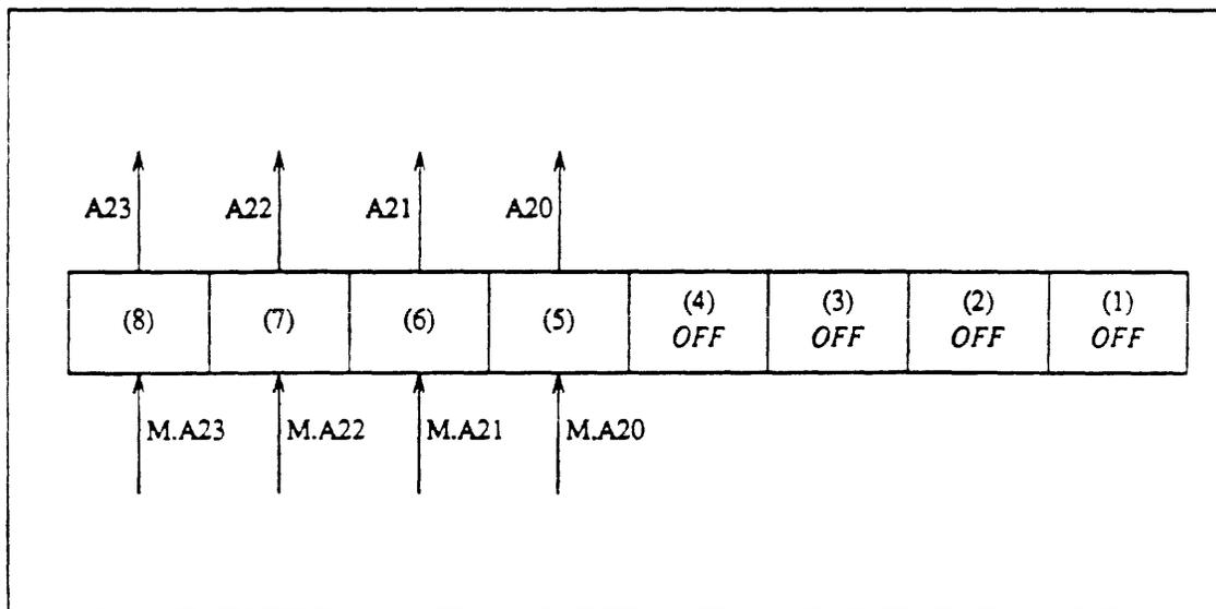
†Since the Multibus address lines use negative logic, a switch section must be set ON to provide a logic 1 to the VMEbus and OFF to provide a logic 0.
