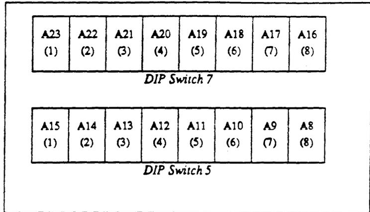
A switch section ON causes a match when the corresponding VME address bit is 0.
