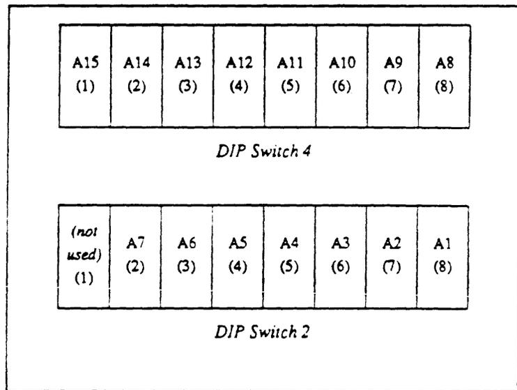
There is a separate switch section for each address bit from A1 to A15. If the switch section is ON, that address bit is compared against the corresponding base address switch section. If the address bit matches the switch section setting, the adapter board responds. If the switch section is OFF, that bit is ignored by the adapter board, and is simply passed through to the Multibus board.
