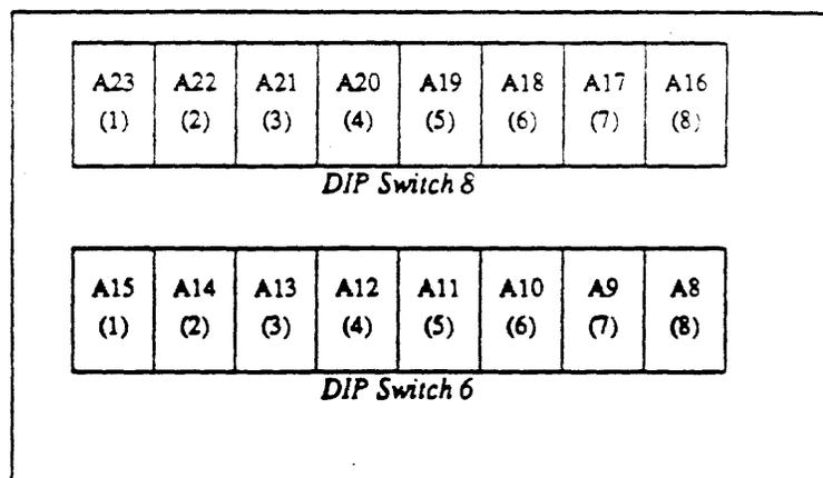
There is a separate switch section for each address bit from A8 to A23.
