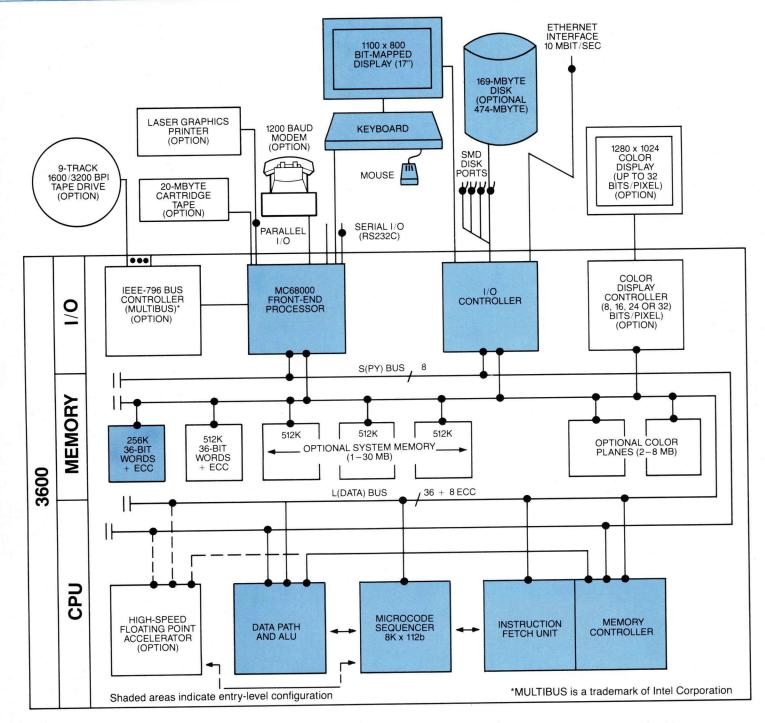
The 3600 Symbol Processor consists of three major subsystems as shown on the simplified diagram above.
