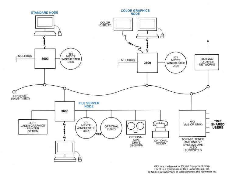
The Symbolics Network System enables Symbolics computers to share resources and exchange information comprehensively with each other and with standard time-shared computer systems. Communication and access are supported via an industry-standard 10 Mbit/sec Ethernet local network. High-level user services, including generic file-system access, file transfer, electronic mail, remote
