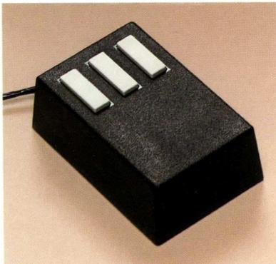
The mouse is a hand-held device that transmits any change in its X or Y position as it is moved over a smooth surface. This movement information updates the position of a cursor on the display, providing immediate visual feedback. The mouse has three buttons that the user can press to give commands as an alternative to typing on the keyboard.
