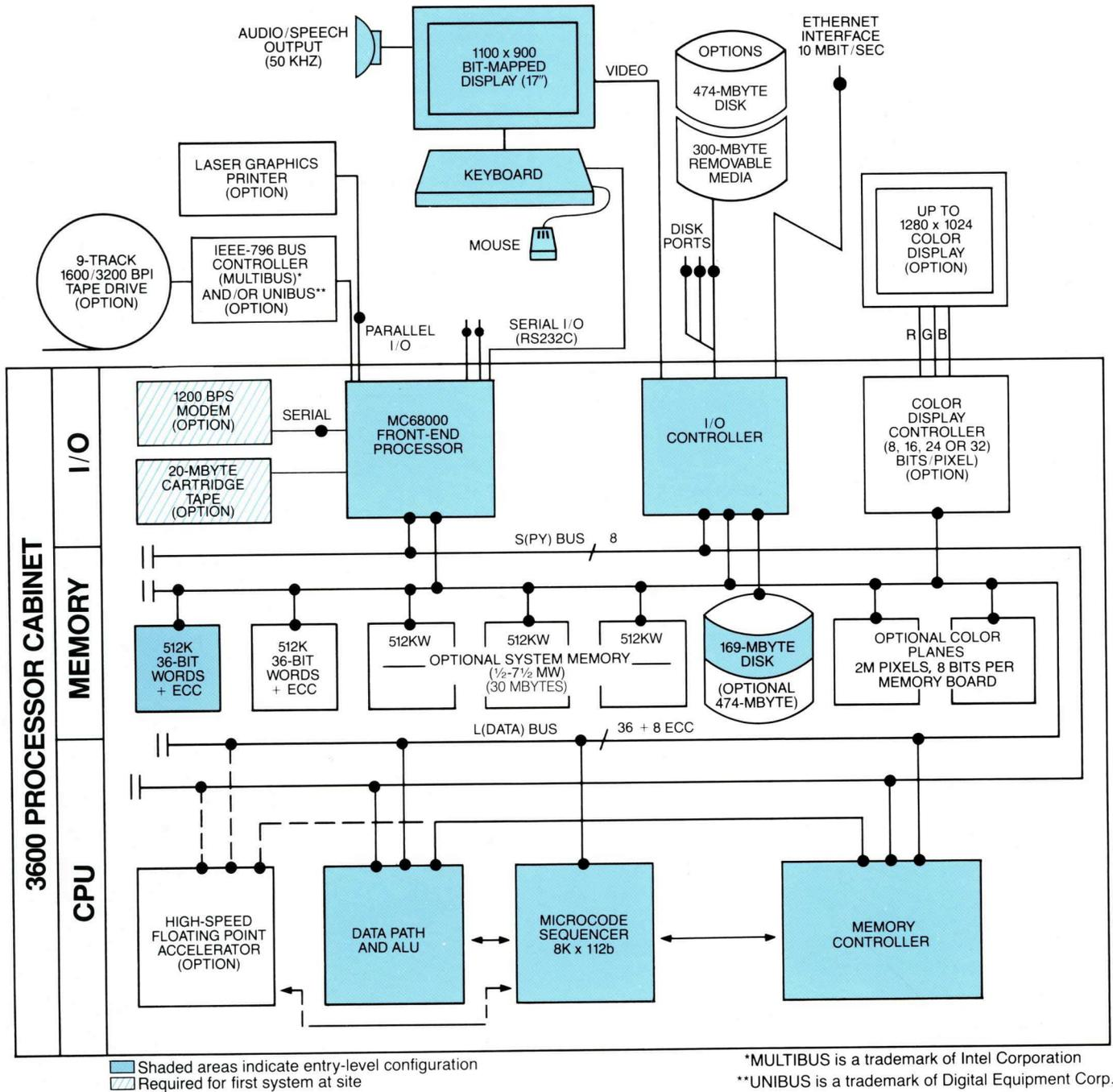
The 3600 Symbol Processor consists of three major subsystems as shown on the simplified diagram above.
