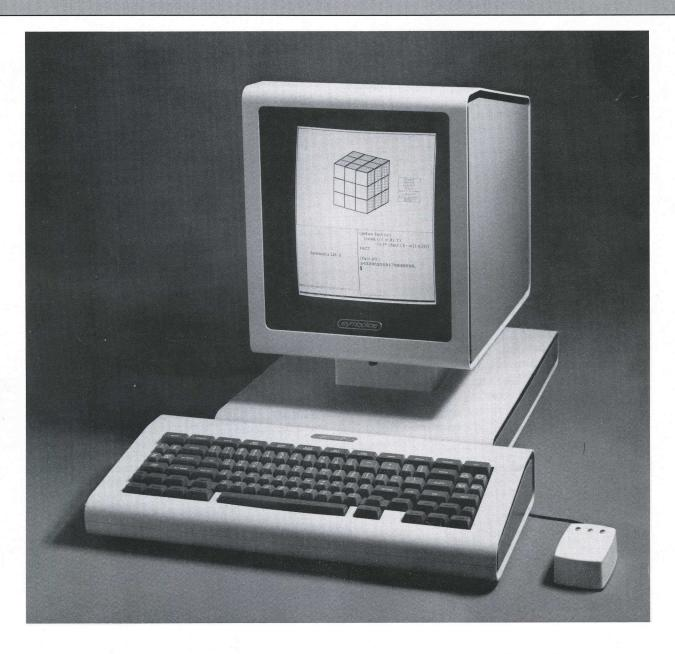
A standard LM-2 symbol processing system consists of a micro-coded 32-bit CPU, 1 Megabyte of main memory, 80 Megabyte fast disk, high resolution B/W graphics display, keyboard, "mouse," Chaosnet local network interface and ZetaLisp programming environment with real-time editor, mail-reader, window system, interpreter, compiler, debugger, local file
