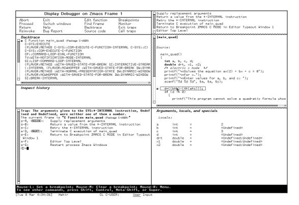
Figure 71. A C Program in the Display Debugger
