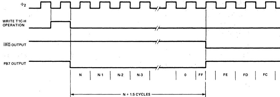
Figure 18. Timer 1 and Timer 2 One-Shot Mode Timing
