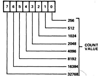
WRITE – 8 BITS LOADED INTO T1 HIGH-ORDER LATCHES. UNLIKE REG 4 OPERATION NO LATCH-TO-COUNTER TRANSFERS TAKE PLACE.
