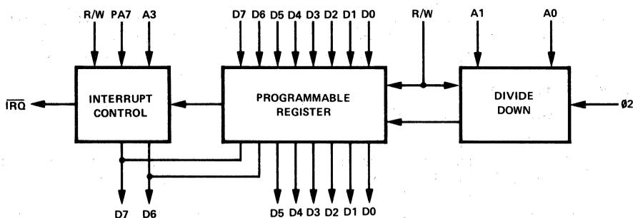
Thus, to arrive at the total elapsed time, merely do a two's complement add to the original time written into the timer. Again, assume time written as 00110100 (=52). With a divide by 8, total time to interrupt is  $(52 \times 8) + 1 = 417T$ . Total elapsed time would be  $416T + 28T = 444T$ , assuming the value read after interrupt was 11100100.
