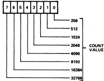
WRITE – 8 BITS LOADED INTO T1 HIGH-ORDER LATCHES. ALSO, AT THIS TIME BOTH HIGH AND LOW-ORDER LATCHES TRANSFERRED INTO T1 COUNTER. T1 INTERRUPT FLAG ALSO IS RESET.
