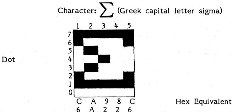
Each byte corresponds to a single column, with each bit corresponding to a single dot.
