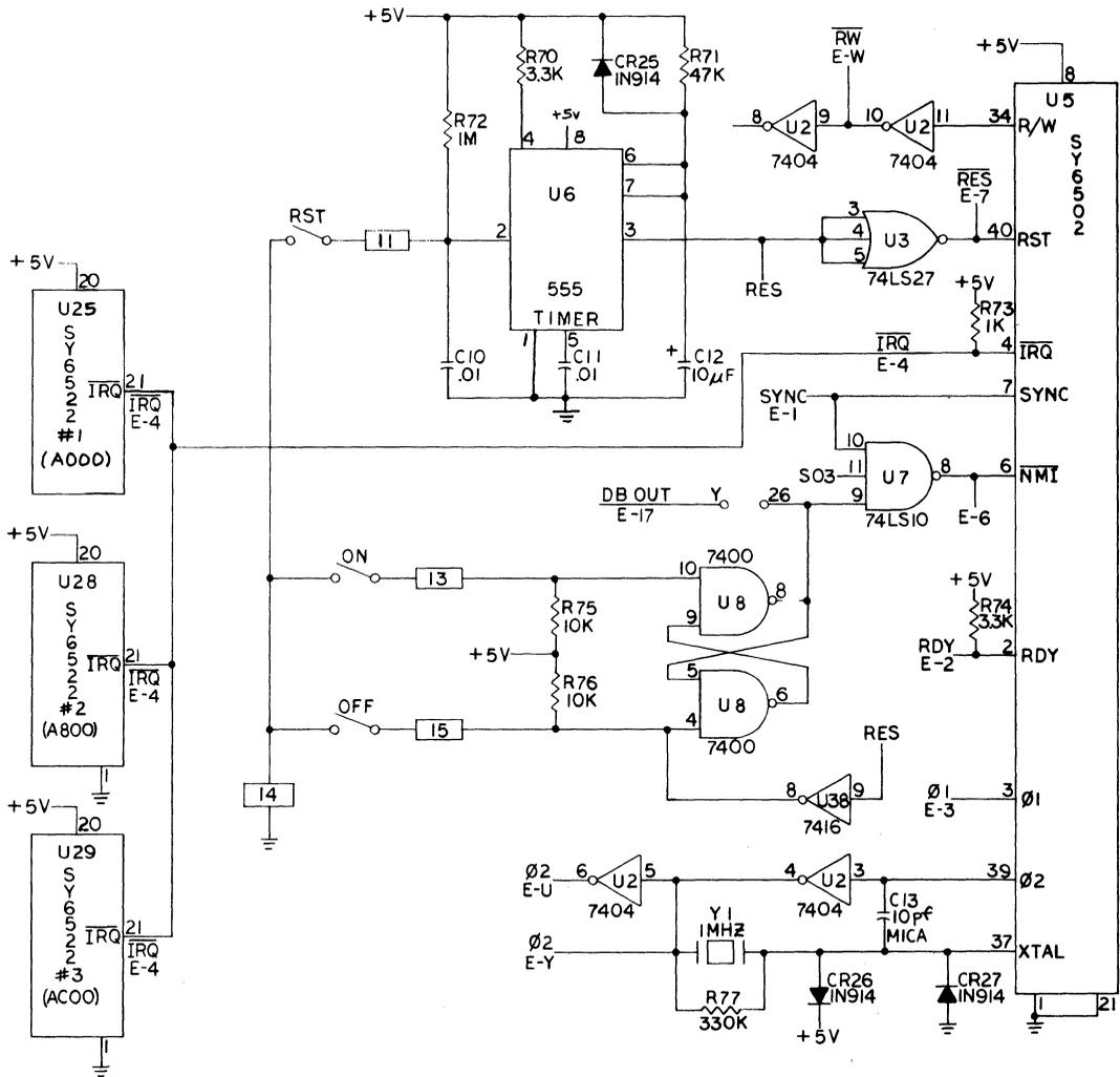
Figure 4-7. CONTROL SECTION SCHEMATIC
