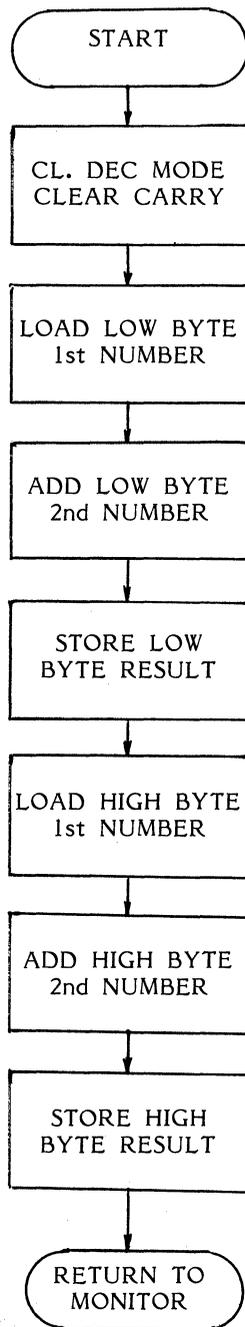
Figure 6-2. DOUBLE-PRECISION ADDITION FLOWCHART
