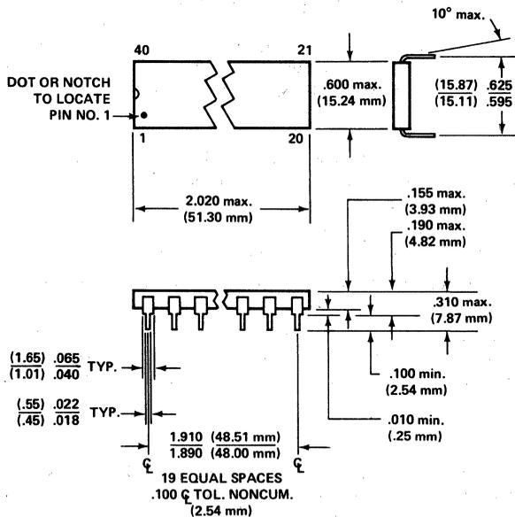
NOTE: Pin No. 1 is in lower left corner when symbolization is in normal orientation
