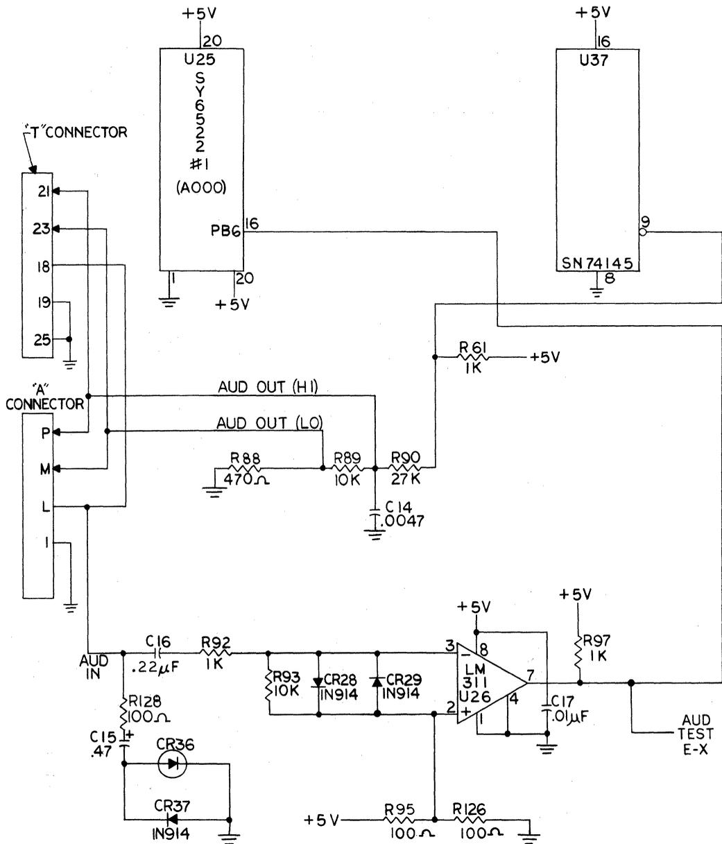
Figure 4-3. AUDIO CASSETTE INTERFACE SCHEMATIC
