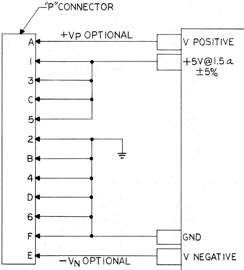
Figure 3-2. POWER SUPPLY CONNECTIONS
