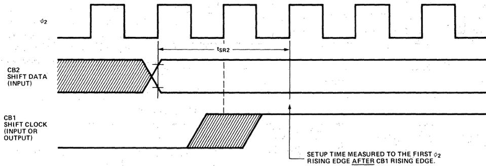
**Figure 5g. Timing for Shift In with Internal or External Shift Clocking**
