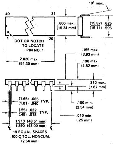
NOTE: Pin No. 1 is in lower left corner when symbolization is in normal orientation
