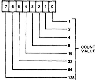
WRITE – 8 BITS LOADED INTO T1 LOW-ORDER LATCHES. THIS OPERATION IS NO DIFFERENT THAT A WRITE INTO REG 4.
