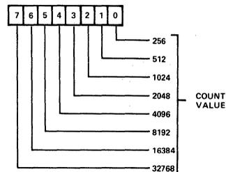
WRITE – 8 BITS LOADED INTO T2 HIGH-ORDER COUNTER. ALSO, LOW-ORDER LATCHES TRANSFERRED TO LOW-ORDER COUNTER. IN ADDITION, T2 INTERRUPT FLAG IS RESET.
