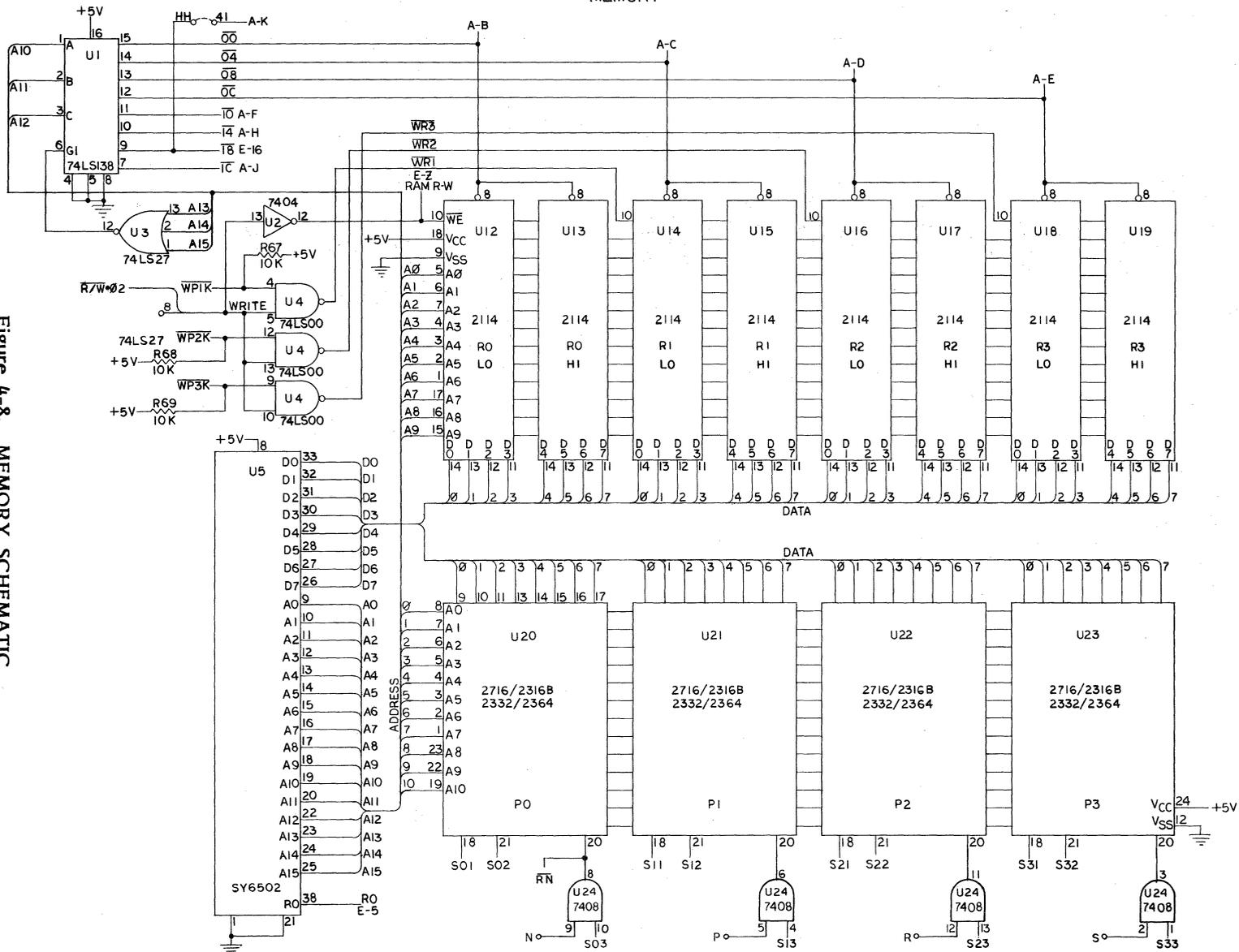
Figure 4-8. MEMORY SCHEMATIC
