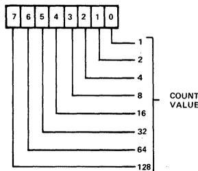
WRITE – 8 BITS LOADED INTO T2 LOW-ORDER LATCHES.
