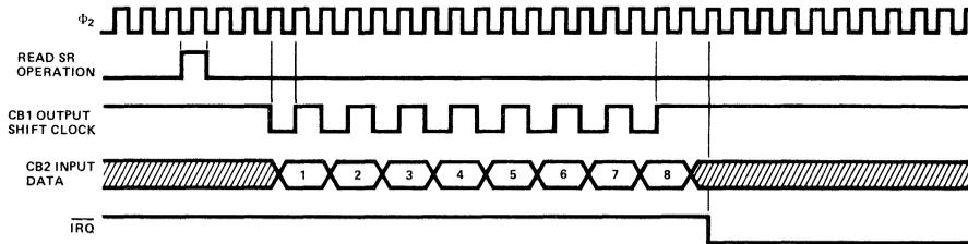
**Shift in Under Control of External CB1 Clock (011)**
