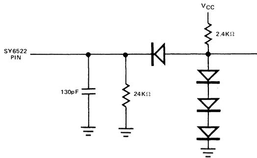
**Figure 2. Test Load (for all Dynamic Parameters)**
