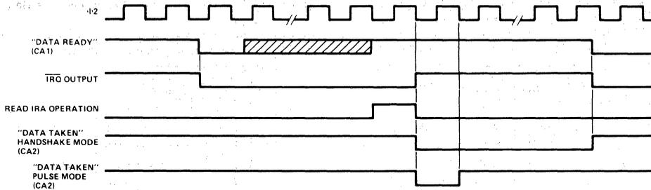
Figure 12. Read Handshake Timing (Port A, Only)
