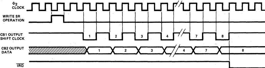
**Shift Out Under Control of External CB1 Clock (111)**
