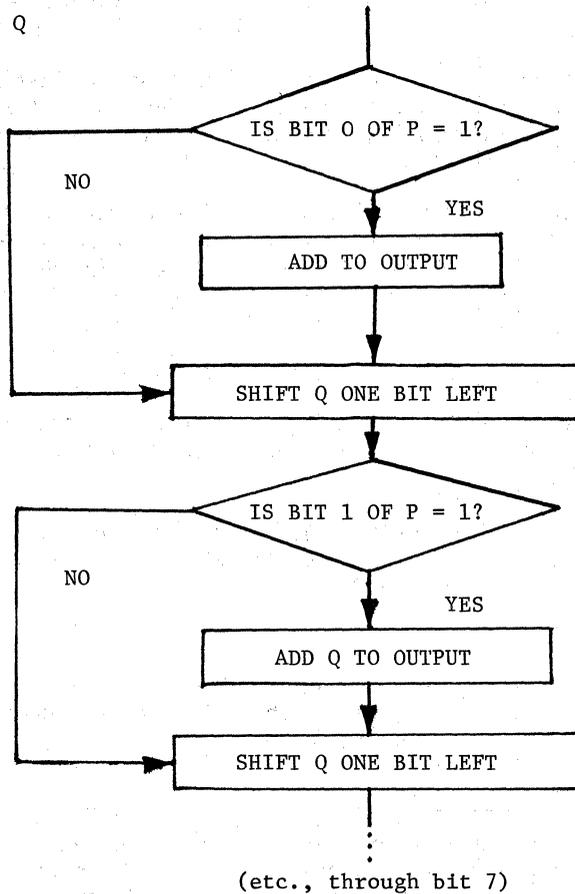
Figure 6-7. DETAILED MULTIPLICATION FLOWCHART
