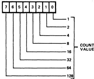
WRITE – 8 BITS LOADED INTO T1 LOW-ORDER LATCHES. LATCH CONTENTS ARE TRANSFERRED INTO LOW-ORDER COUNTER AT THE TIME THE HIGH-ORDER COUNTER IS LOADED (REG 5).
