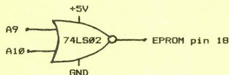
EPROM pin 18 (chip enable) must be disconnected from ground. I connected wires to A9 and A10 at pins 19 and 22 of the SYM ROM sockets.
