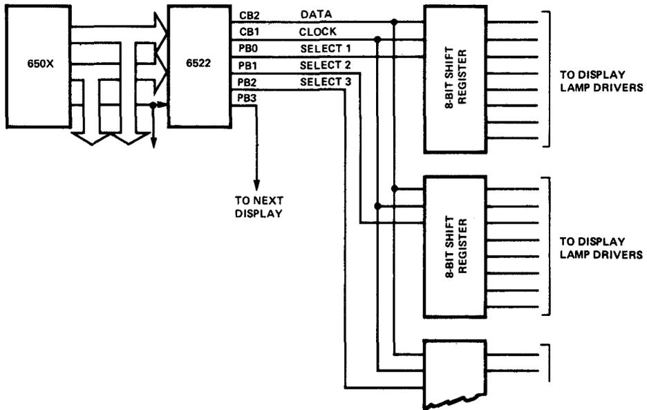
Remote input devices can be serviced in much the same manner by shifting data into the Shift Register under control of a peripheral port output as shown in Figure 21. Each set of input switches can be polled by first selecting the set to be polled and then triggering the shifting operation with a Shift Register read operation. A shift register interrupt can be used to cause the processor to read the resulting input information after shifting is complete.
