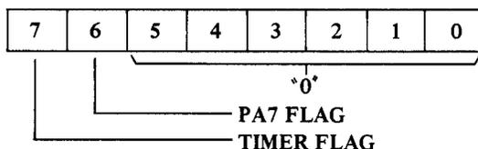
The PA7 flag is cleared when the Interrupt Flag Register is read. The timer flag is cleared when the timer register is either written or read.
