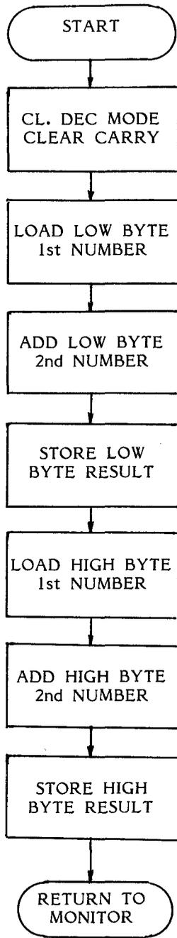
Figure 6-2. DOUBLE-PRECISION ADDITION FLOWCHART
