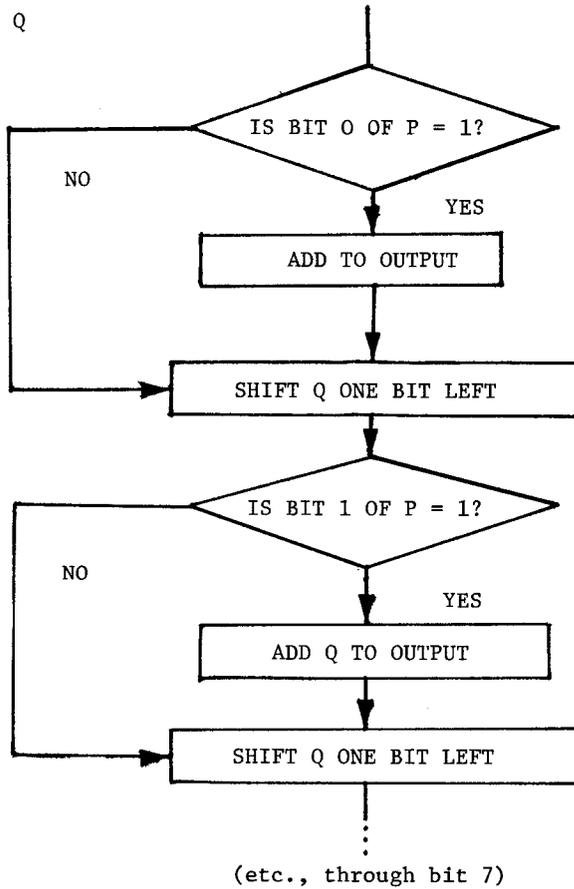
Figure 6-7. DETAILED MULTIPLICATION FLOWCHART
