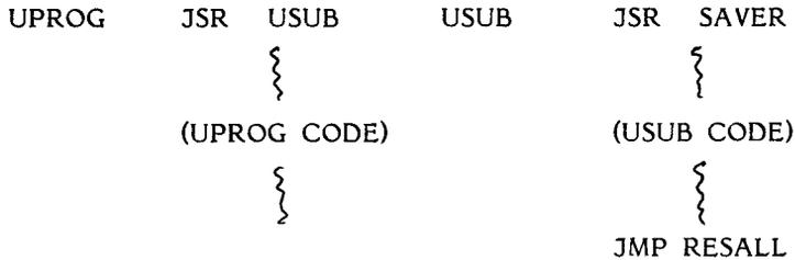
In this example, UPROG calls USUB. USUB calls SAVER, performs its function, and then jumps to RESALL. RESALL restores all registers and returns to UPROG. If RESXF or RESXAF were used instead of RESALL, UPROG would receive the F, or F and A registers as left by USUB.
