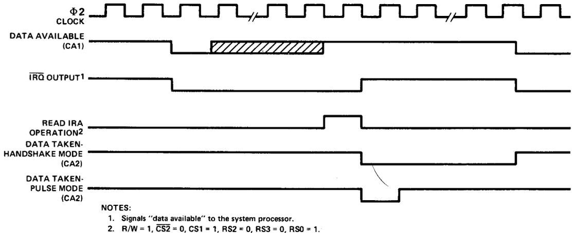
Figure 7. WRITE HANDSHAKE TIMING SEQUENCE
