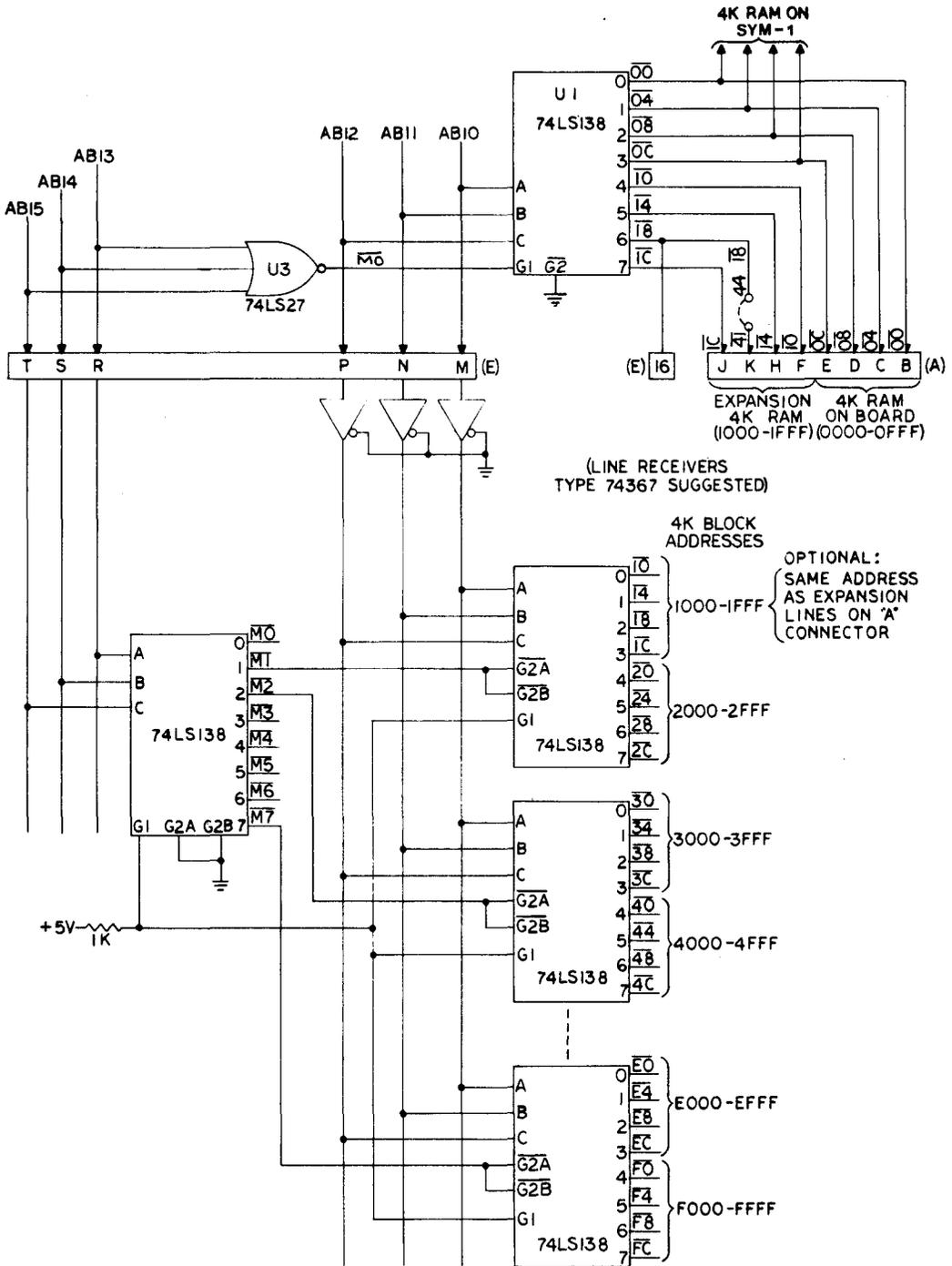
**Figure 8-2. MEMORY - I/O EXPANSION TO 65K**
