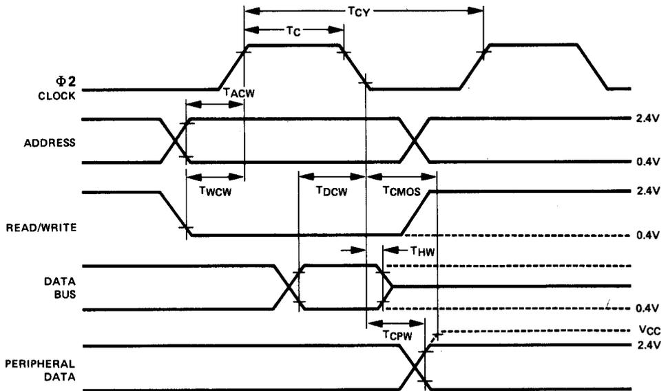
**Figure 4. I/O TIMING CHARACTERISTICS**
