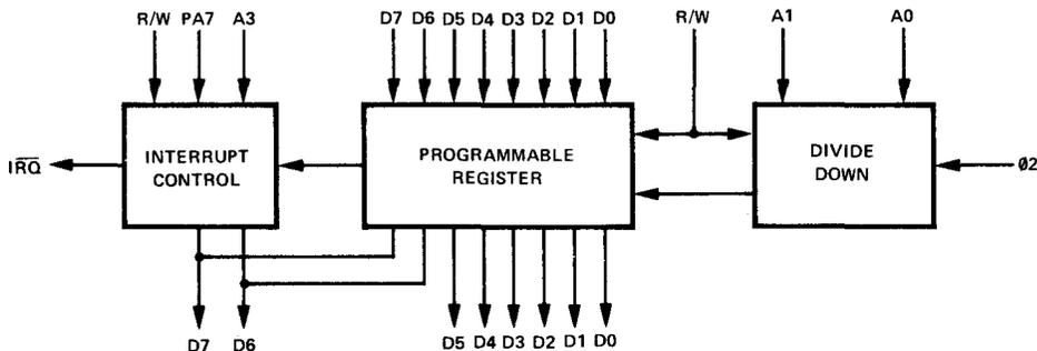
Thus, to arrive at the total elapsed time, merely do a two's complement add to the original time written into the timer. Again, assume time written as 00110100 (=52). With a divide by 8, total time to interrupt is  $(52 \times 8) + 1 = 417T$ . Total elapsed time would be  $416T + 28T = 444T$ , assuming the value read after interrupt was 11100100.
