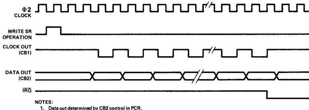
**Mode 111 - Shift out under Control of an External Pulse**
