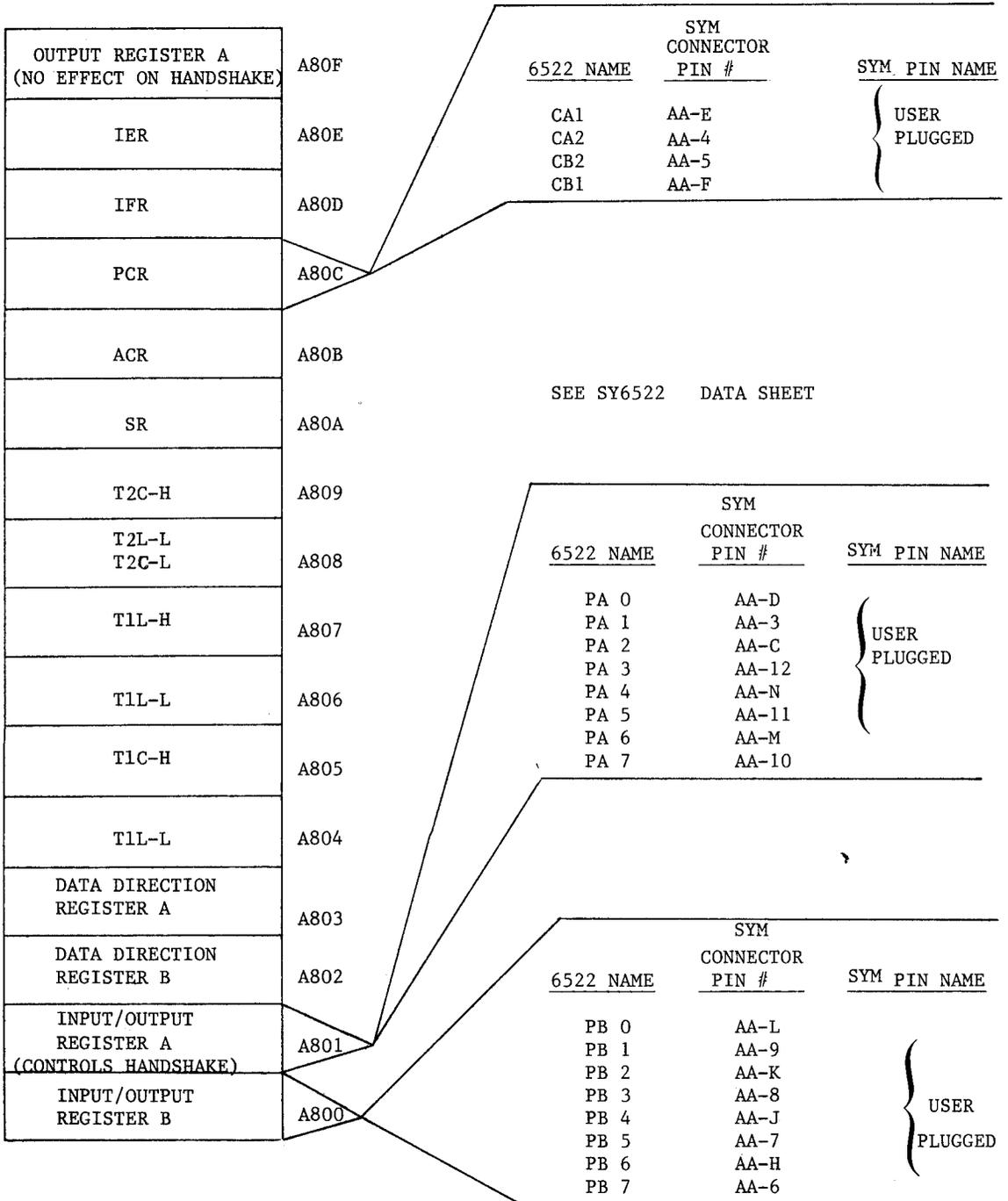
Figure 4-10. MEMORY MAP FOR SY6522 VIA #2 (DEVICE U28-USER SUPPLIED)
