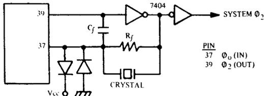
*SY6502 Series Mode Crystal Controlled Oscillator*
