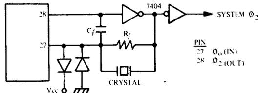
*SY6503,4,5,6 Series Mode Crystal Controlled Oscillator*
