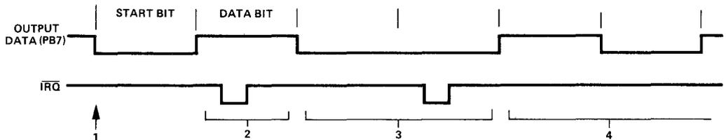
1. Load T into T1 counter and latch. Load T into T2 to trigger T1 latch reload.
