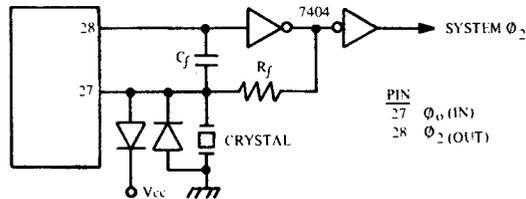
*SY6503,4,5,6 Parallel Mode Crystal Controlled Oscillator*
