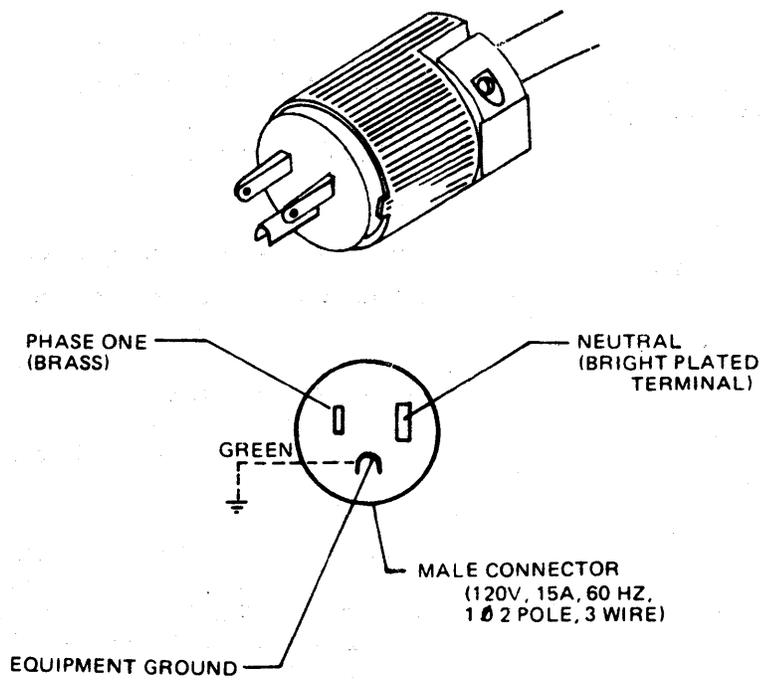
Figure 2-12. CDC 9762 60 Hz AC Power Connector
