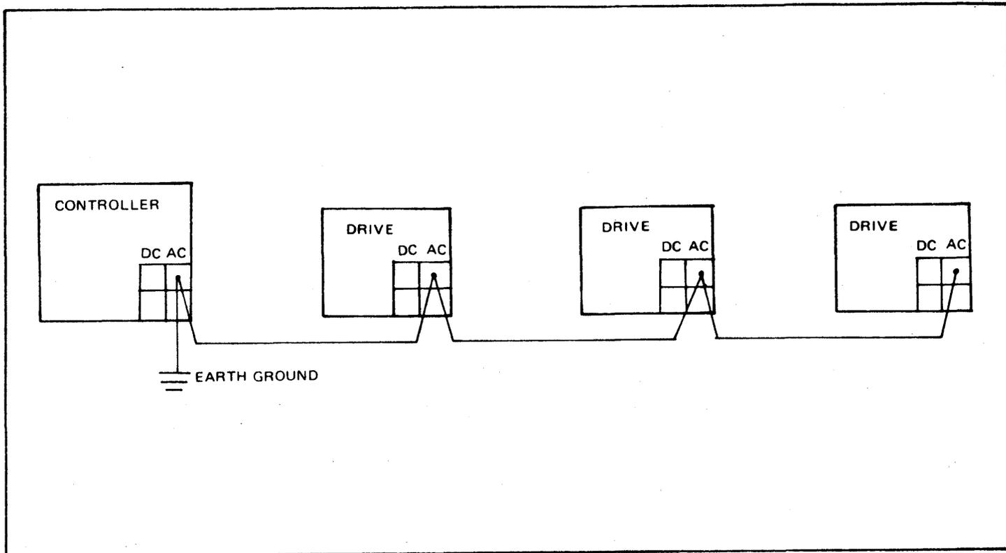
Figure 2-9. Daisy Chain Grounding System
