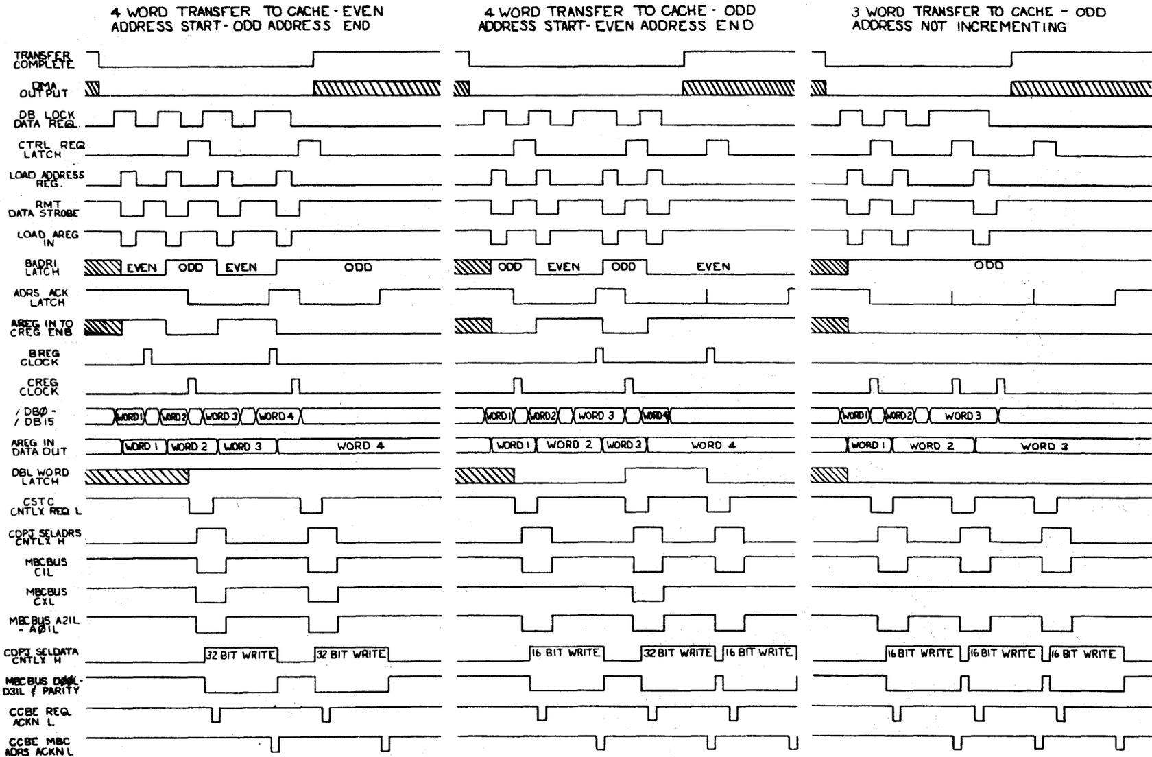
Figure 10-2. Timing Diagram, Cache - Write
