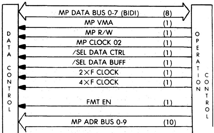
**Figure 5-14. OP Control - Data Control Interface**
