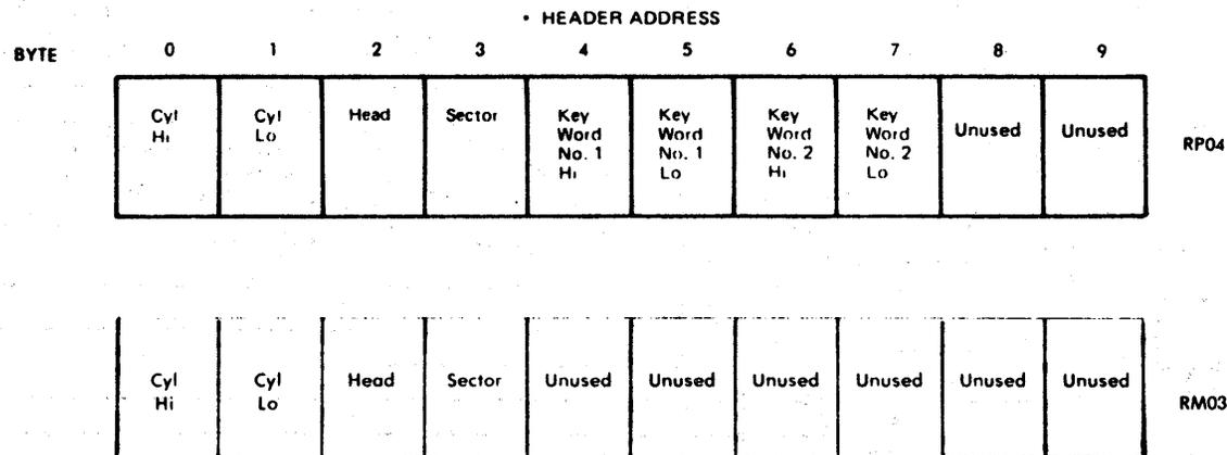
**NOTE:** All ten header address bytes are timed although only cylinder, head, and sector are read.
