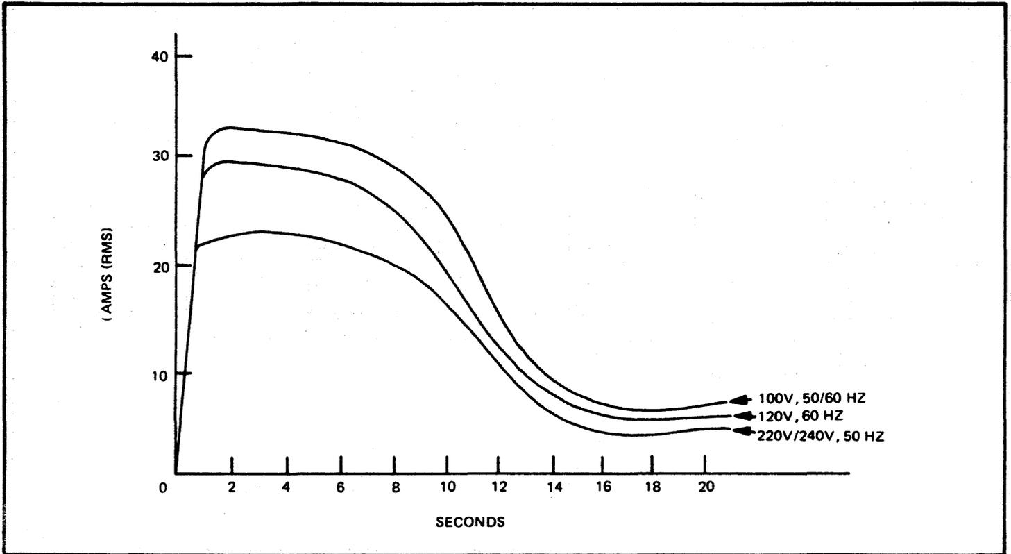
Figure 2-10. 9762 Line Current Versus Start-Up Time
