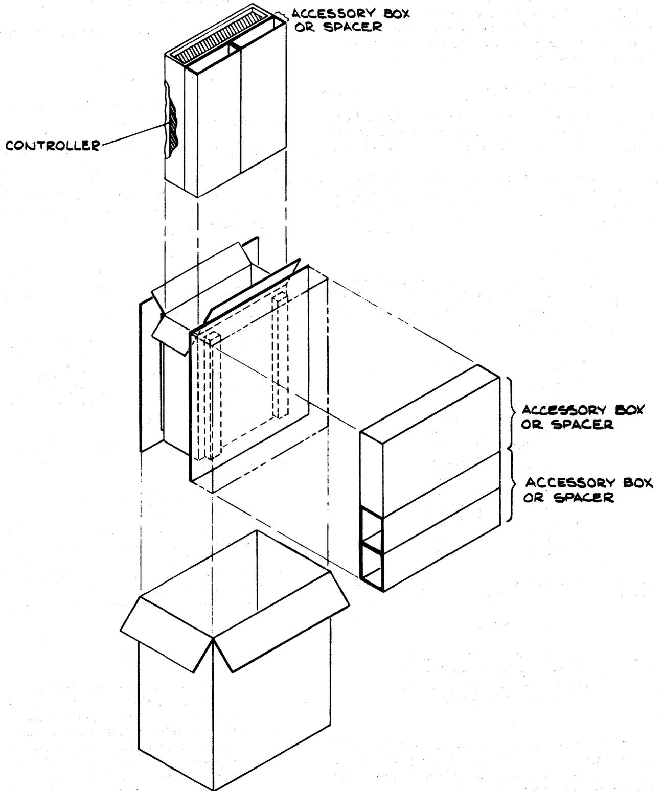
Figure 2-15. 9400 Controller Packing
