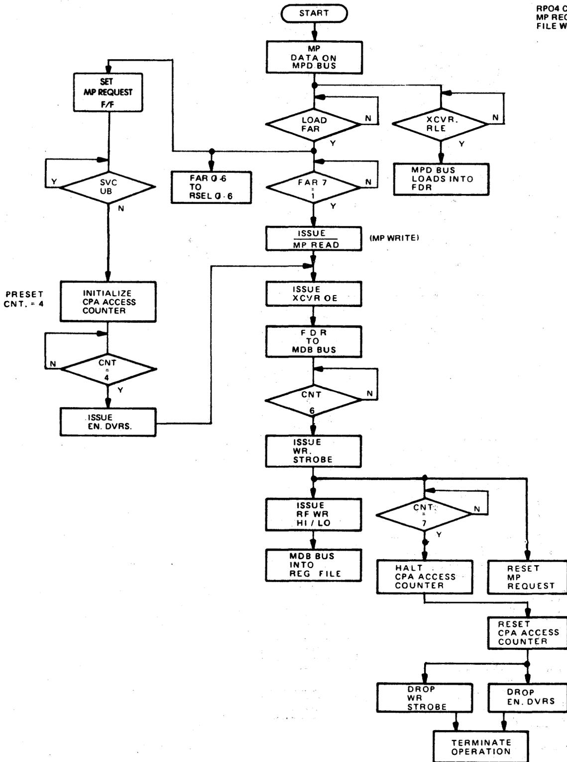
FIGURE 5-9. 9400 RPO4 CPA, MICROPROCESSOR REGISTER FILE WRITE FLOW CHART
