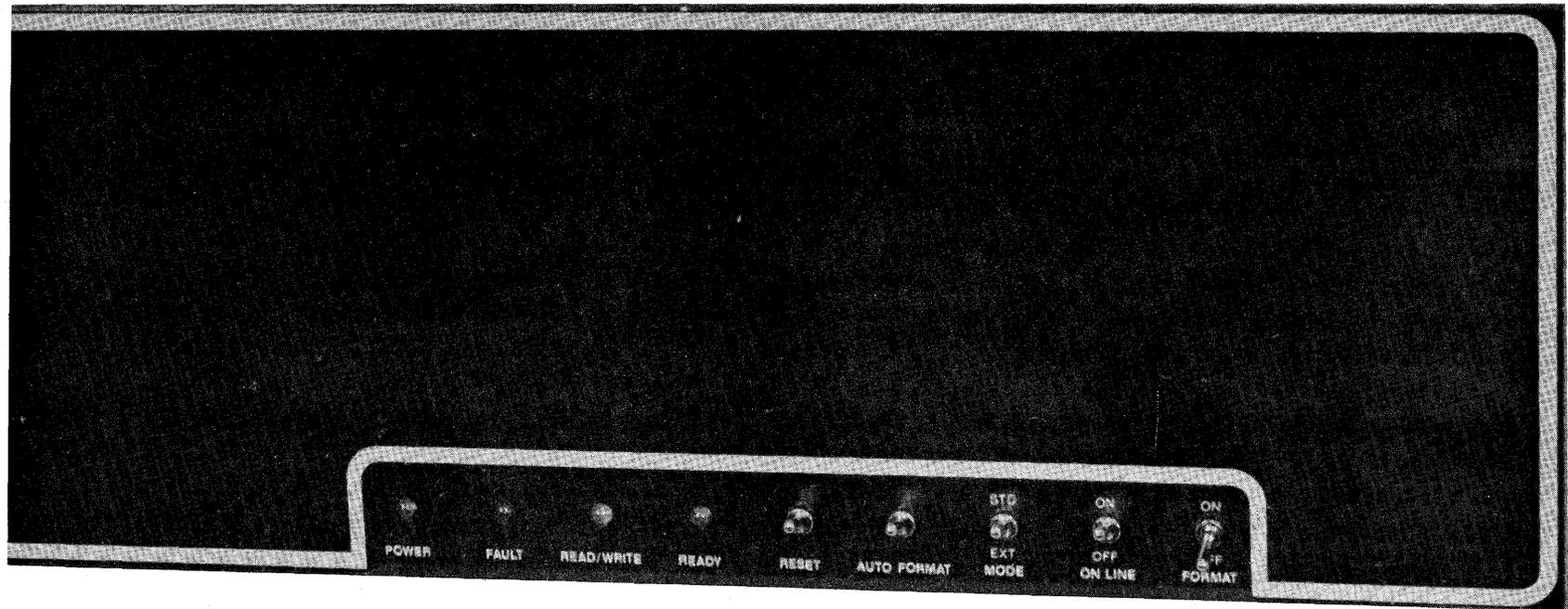
Figure 3-1. Series 9400 Disk Controller Controls and Indicators, Front Panel
