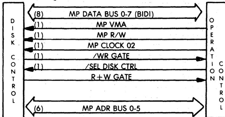
**Figure 5-15. Operation Control - Disk Control**
