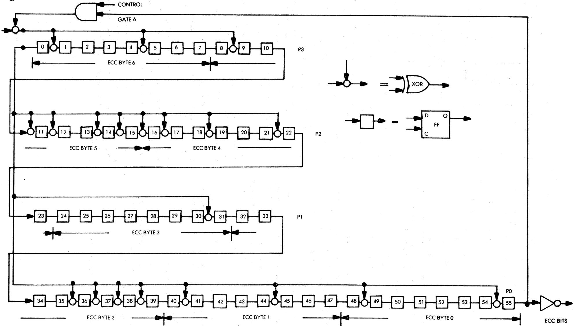
Figure 5-34. ECC Hardware During Write Operation
