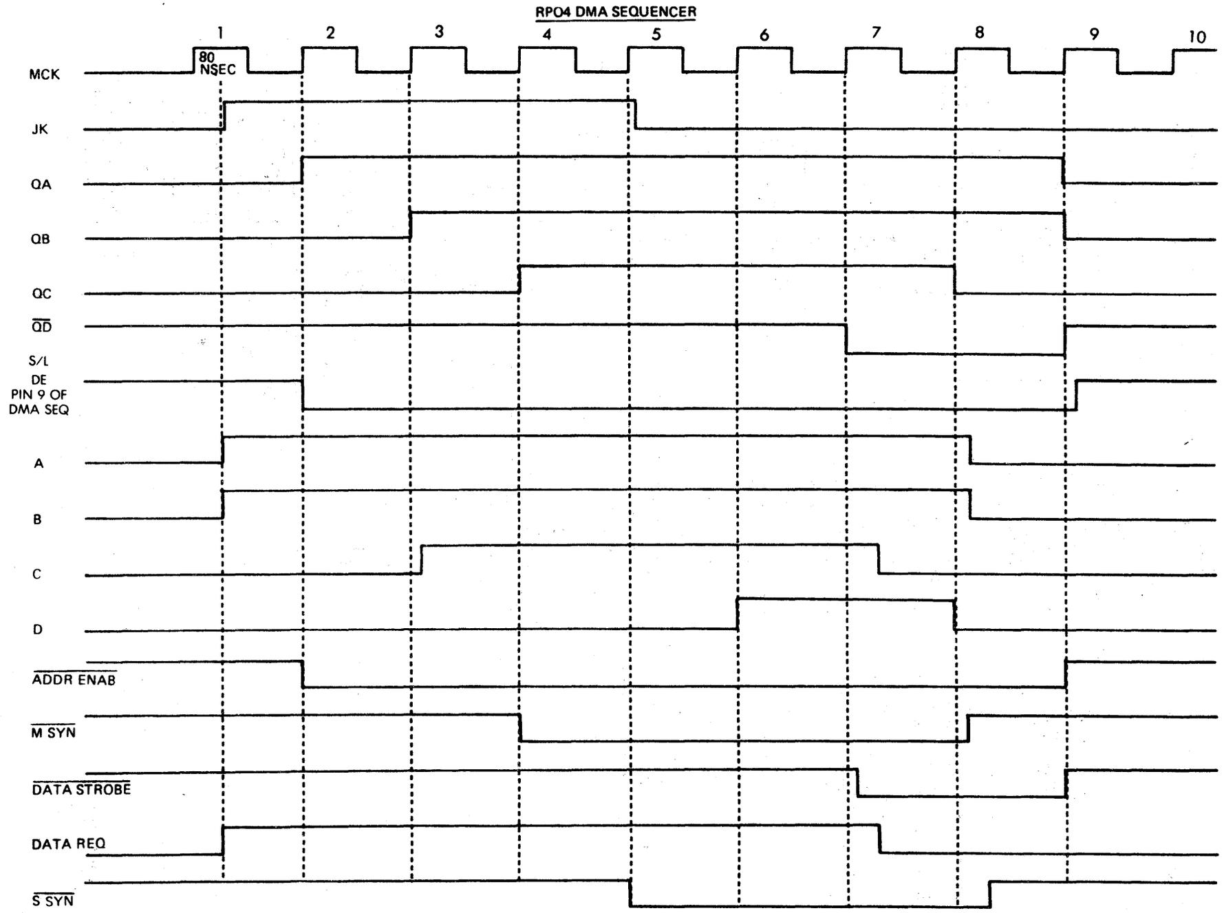
FIGURE 5-12. 9400 RP04 CPA, DIRECT MEMORY ACCESS SEQUENCER TIMING DIAGRAM
