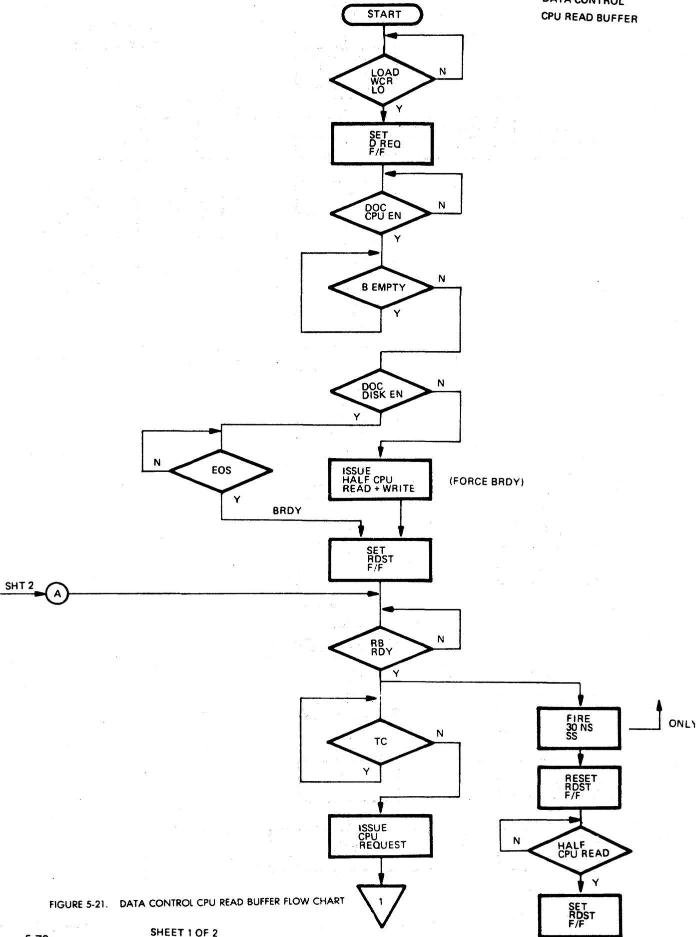
FIGURE 5-21. DATA CONTROL CPU READ BUFFER FLOW CHART
