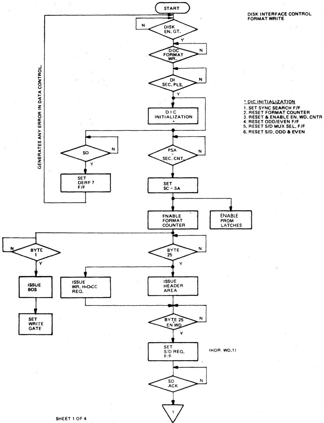
FIGURE 5-28. DISK INTERFACE CONTROL FORMAT WRITE FLOW CHART
