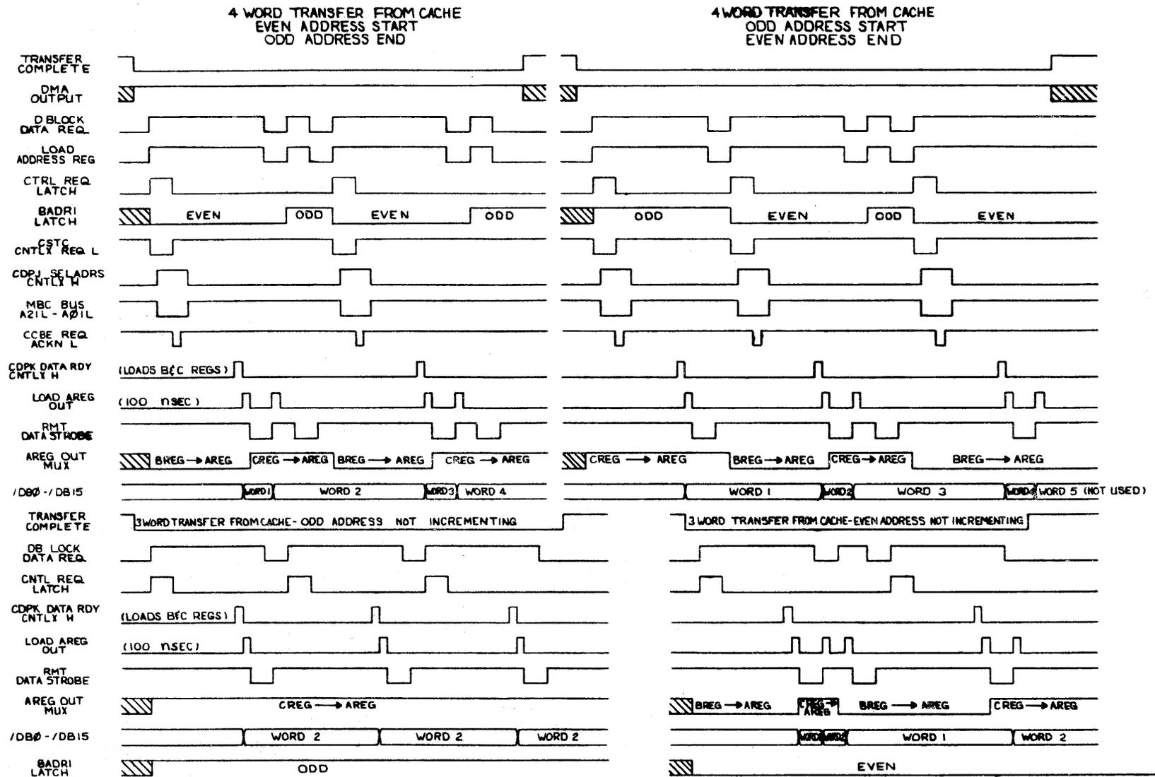
Figure 10-3. Timing Diagram, Cache - Read
