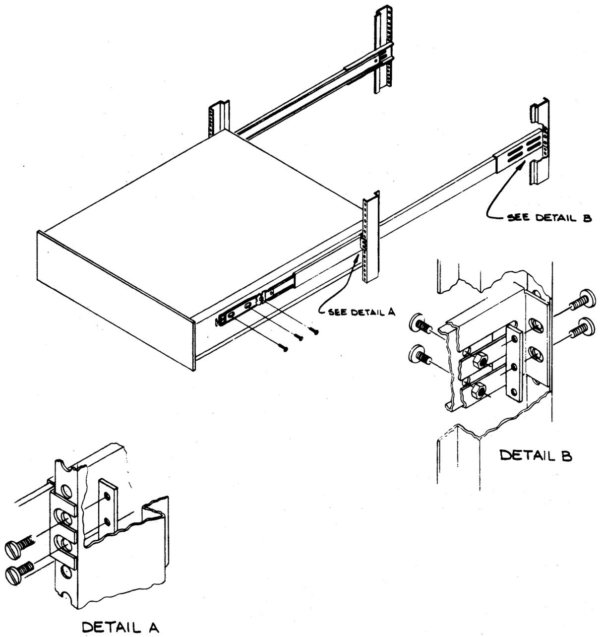
Figure 2-16. 9400 System Installation
