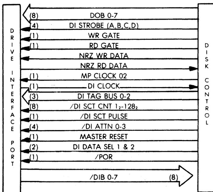
Figure 5-17. Disk Control - Drive Interface Port
