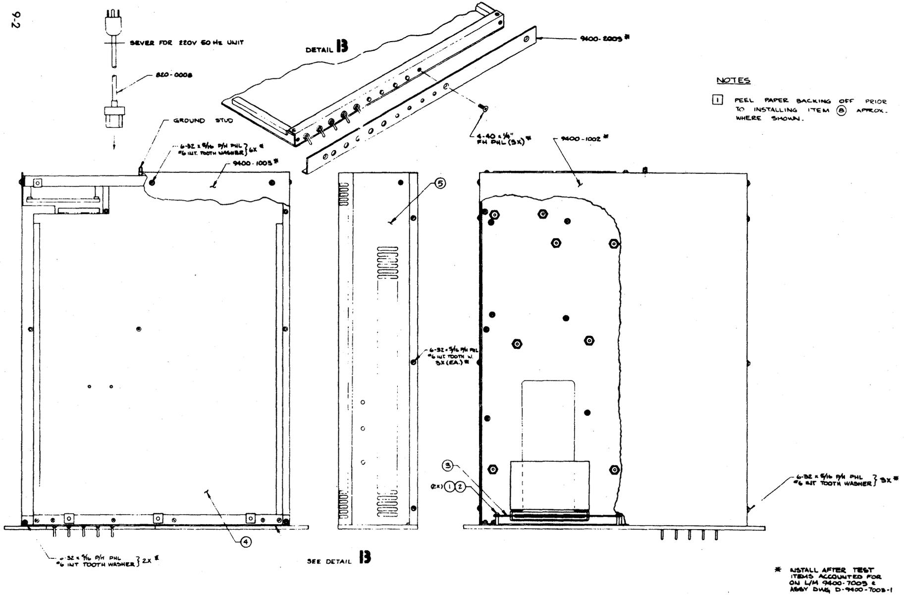
Figure 9-1. Mainframe and Basic Controller Assembly
