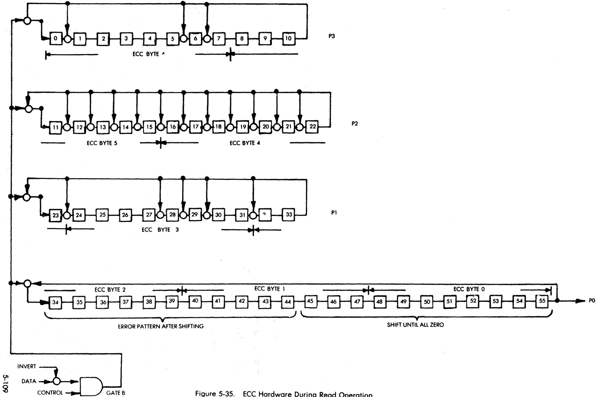
Figure 5-35. ECC Hardware During Read Operation
