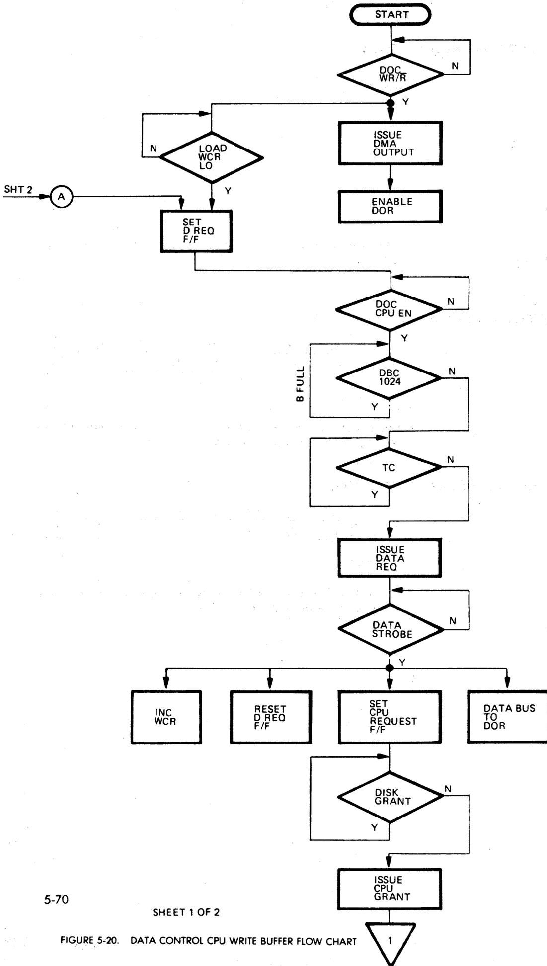
FIGURE 5-20. DATA CONTROL CPU WRITE BUFFER FLOW CHART
