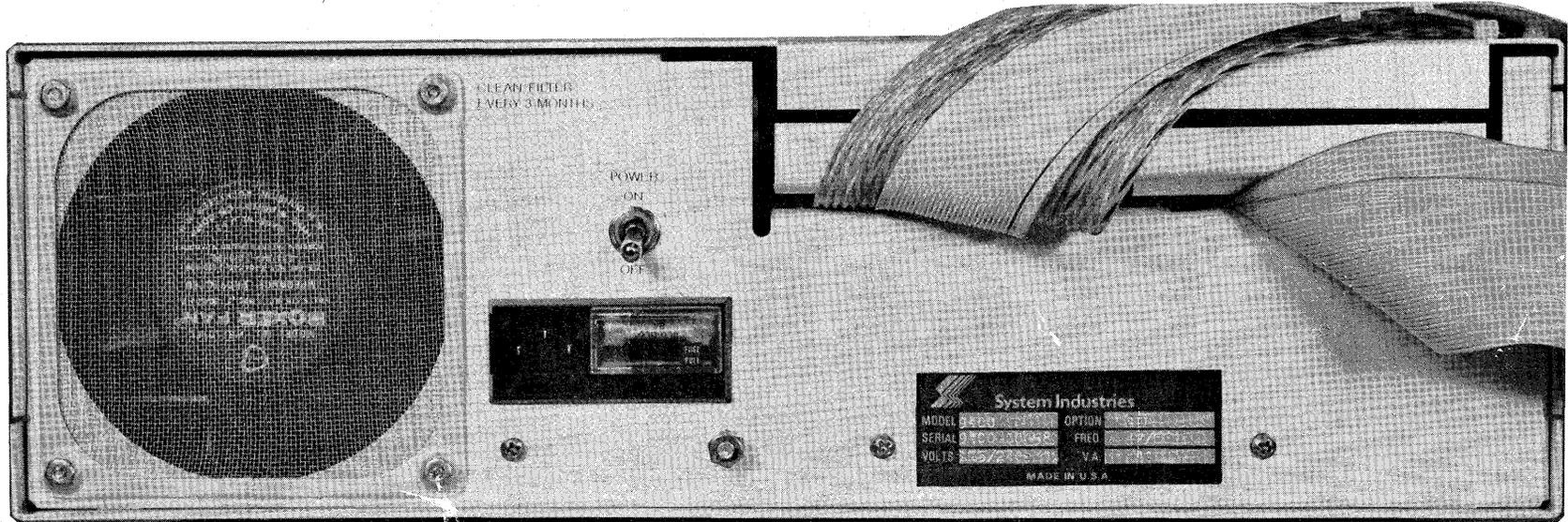
Figure 3-2. Series 9400 Disk Controller Controls and Indicators, Rear Panel
