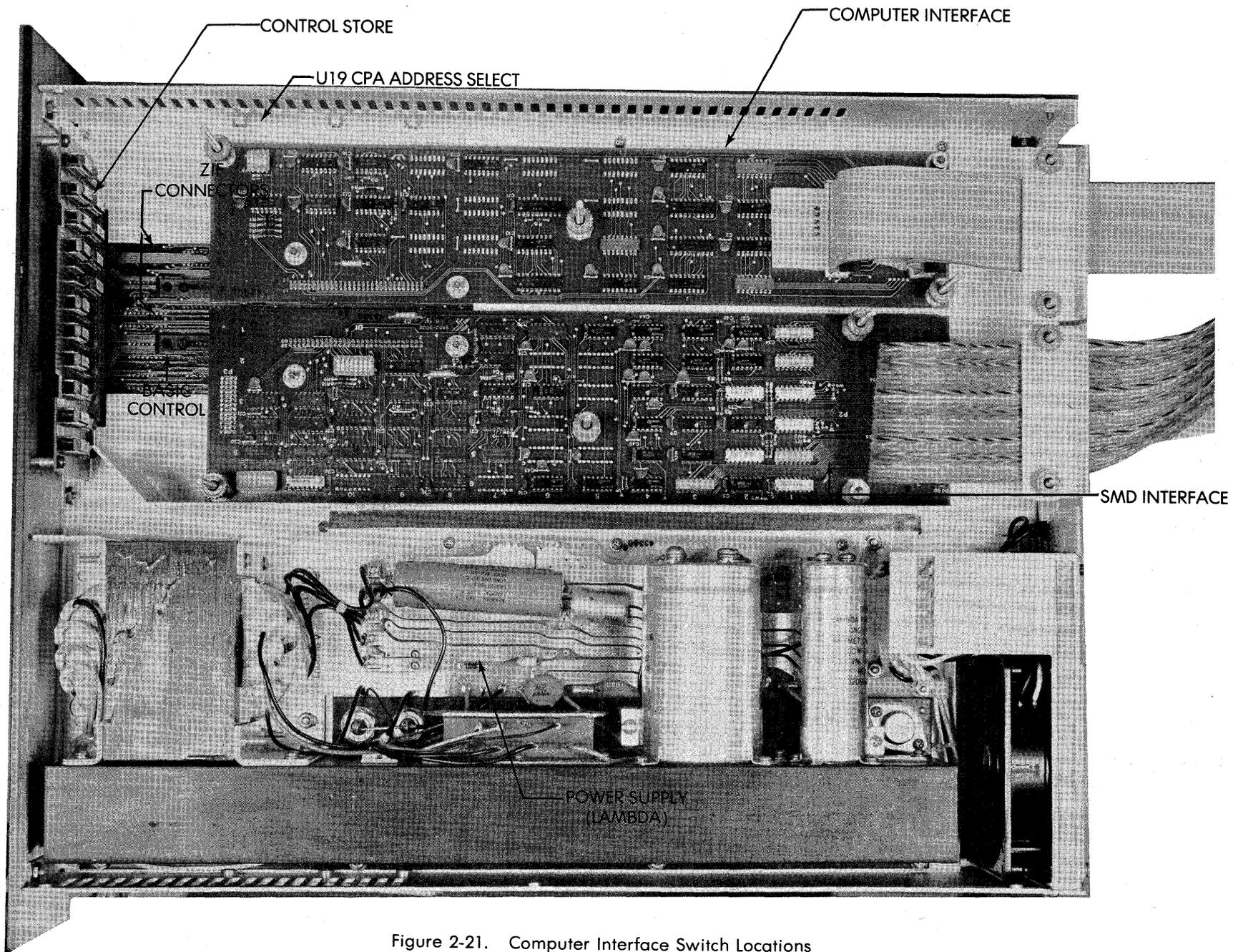
Figure 2-21. Computer Interface Switch Locations
