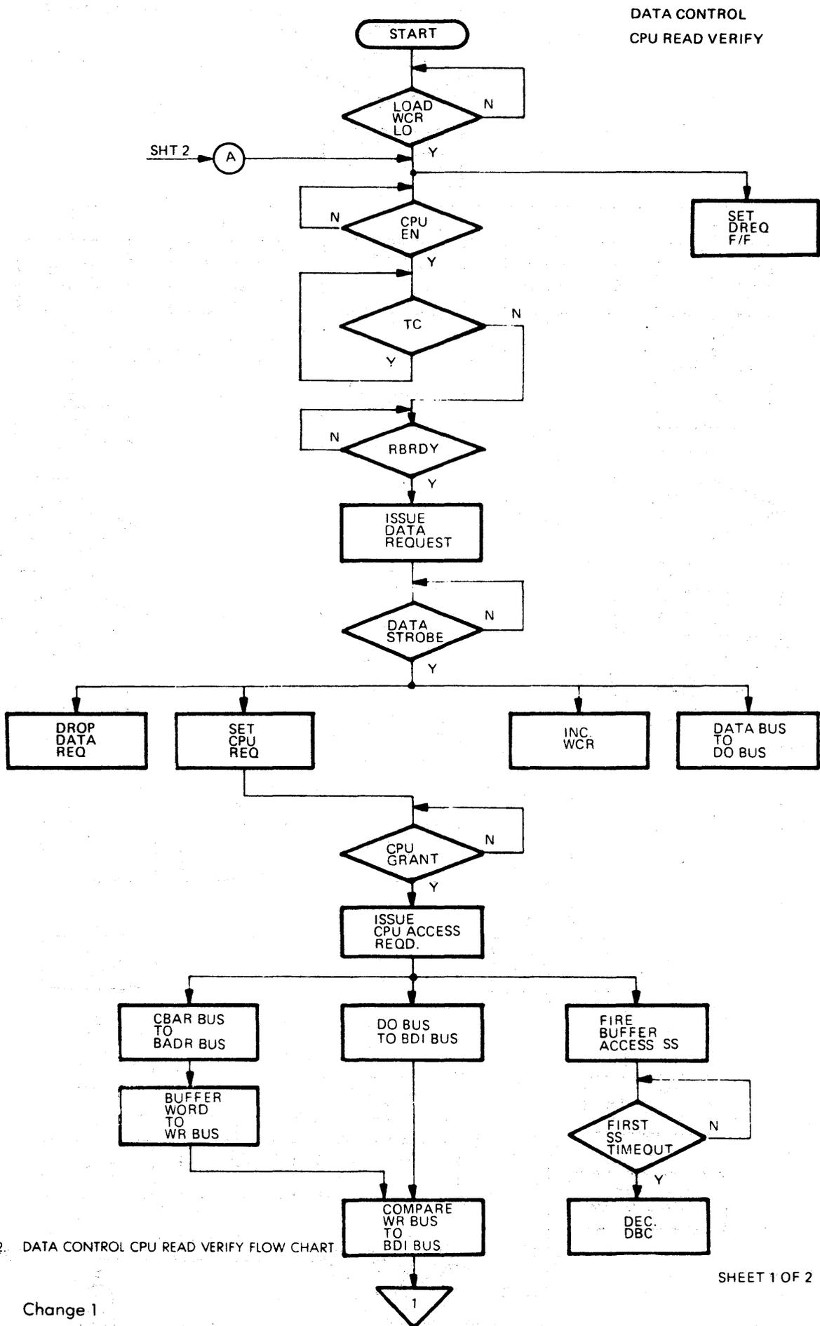
FIGURE 5-22. DATA CONTROL CPU READ VERIFY FLOW CHART
