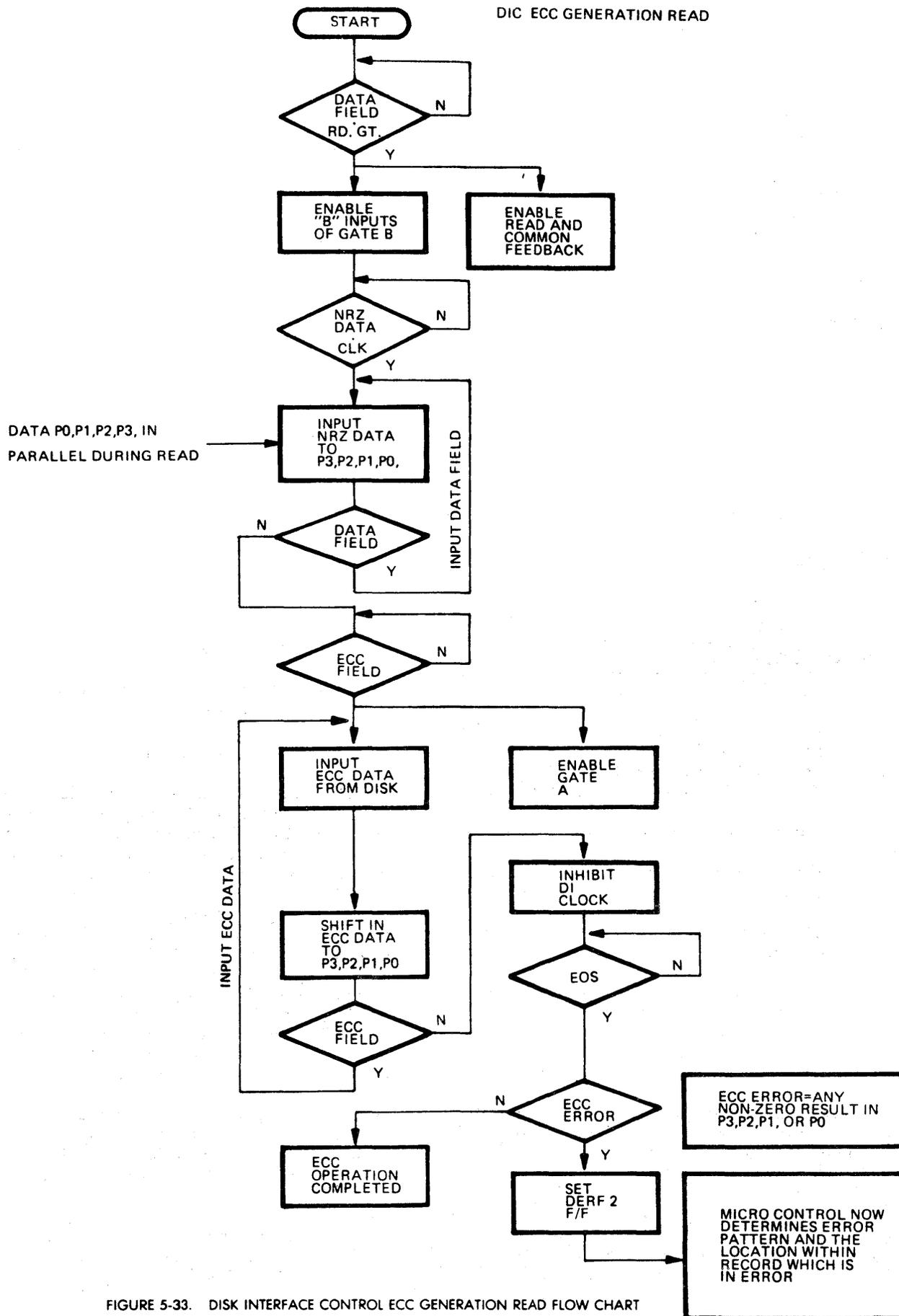
FIGURE 5-33. DISK INTERFACE CONTROL ECC GENERATION READ FLOW CHART
