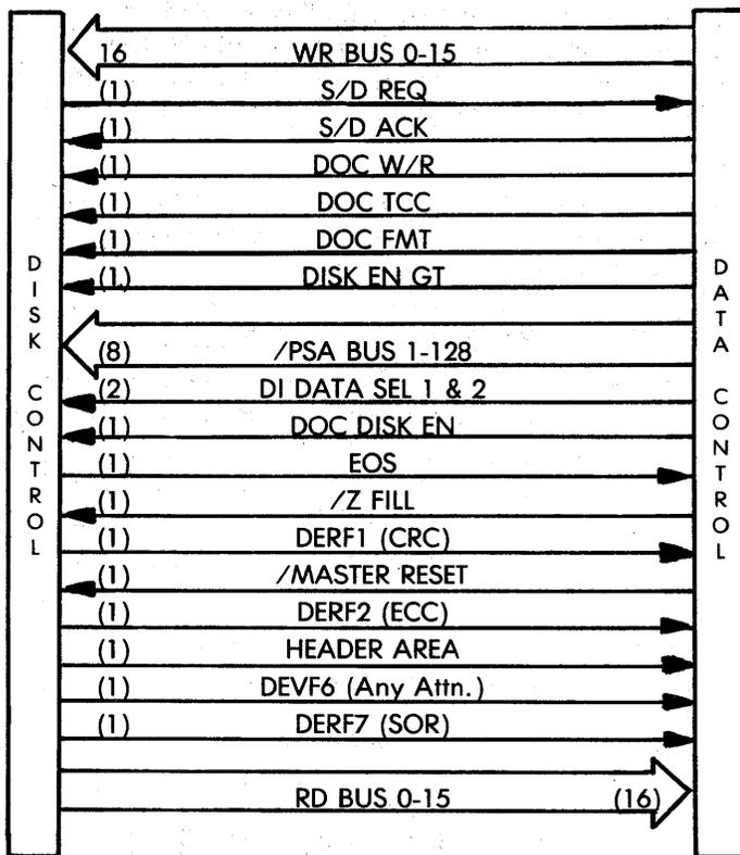
Figure 5-16. Data Control - Disk Control Interface
