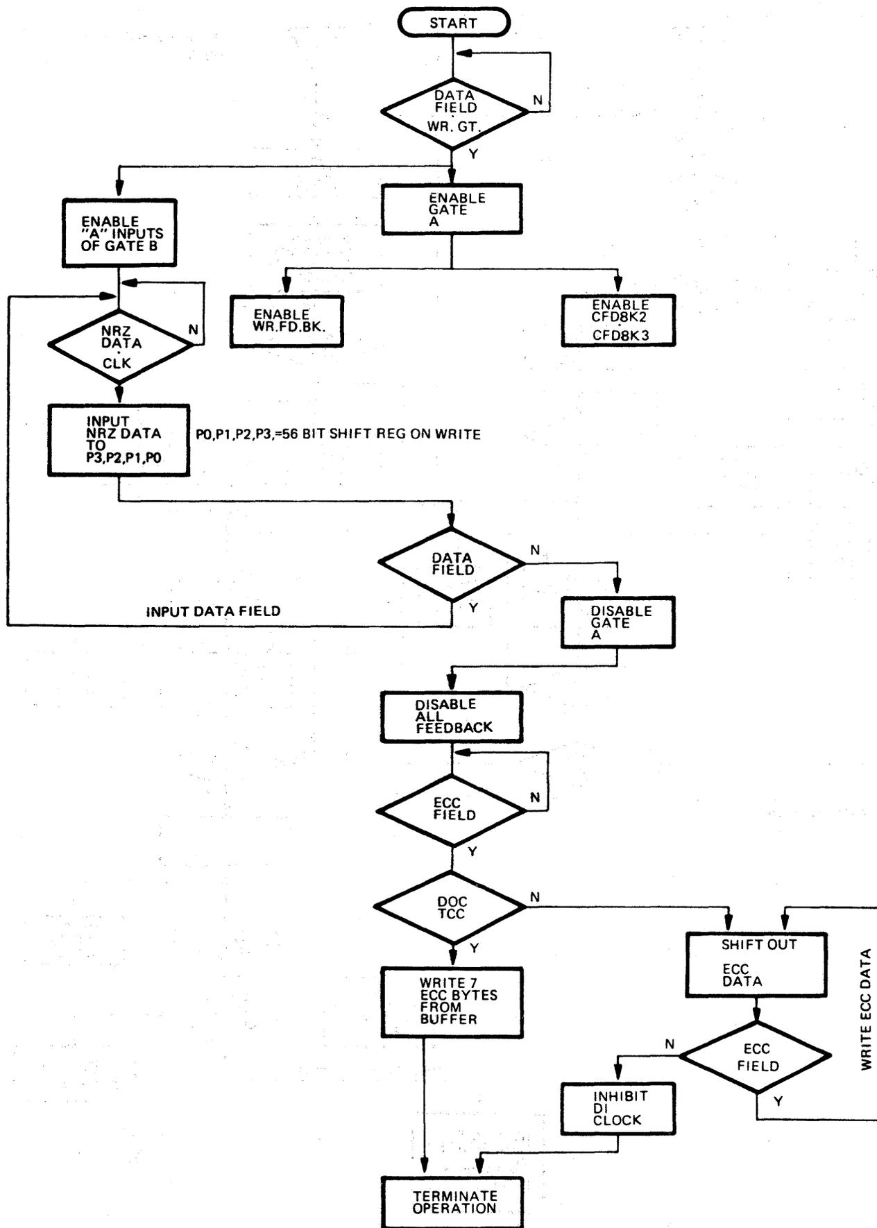
FIGURE 5-32. DISK INTERFACE CONTROL ECC GENERATION WRITE FLOW CHART
