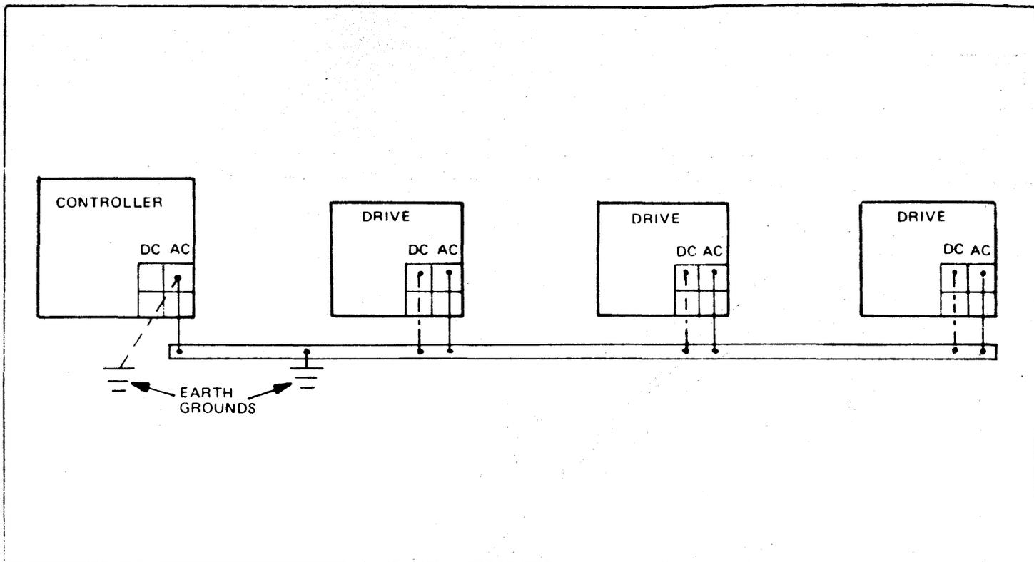
Figure 2-8. Floor Grid Grounding System
