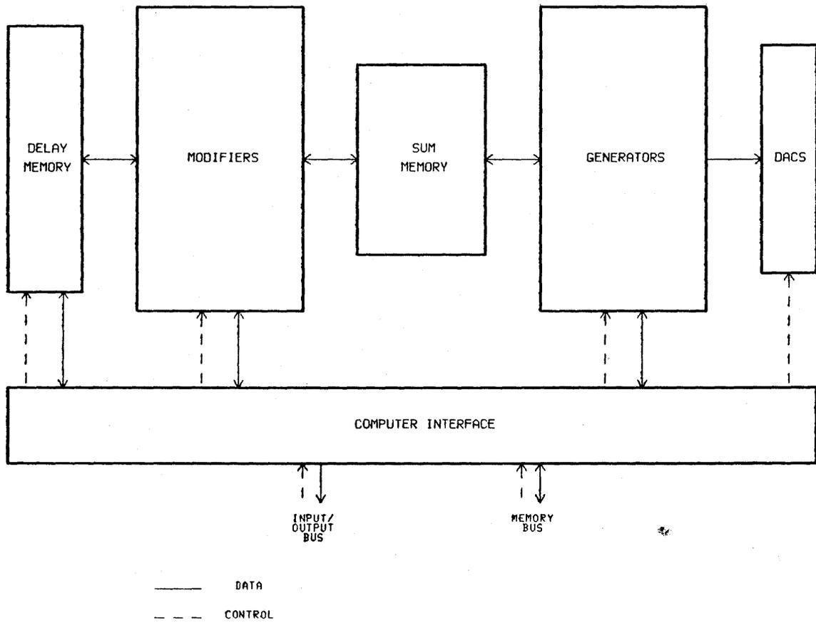
Fig. 1. Synthesizer Block Diagram
