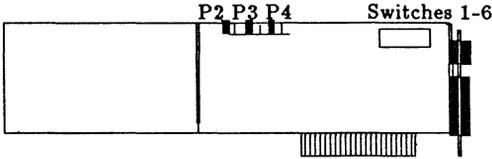
**II) Check JRAM-3 switches. SW1 and SW6 should be ON.** The six switches on the top right corner of the JRAM-3 board assign a unique set of bankswitching control addresses to the board for use by JETDRIVE, JSPOOL, multitasking software, and other packages using the Tall Tree Systems bankswitching standard. Every JRAM, JRAM-2, and JRAM-3 board in the computer must be identified by its own distinct addresses.
