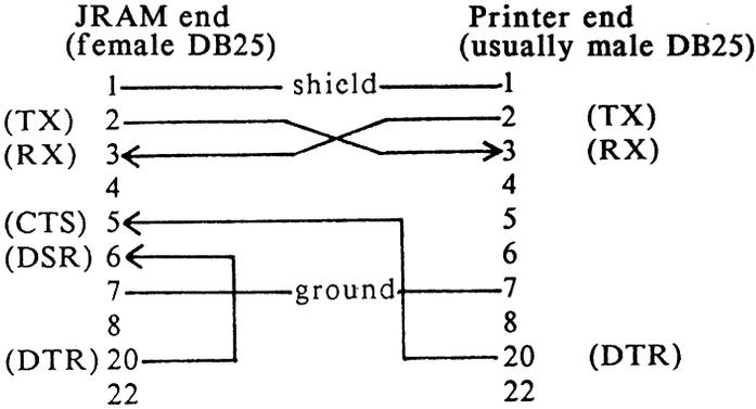
These "universal" cables ignore some ready lines used by some printers to signal specific problems such as "out of paper" or "buffer full". These signals are different for every printer that uses them. However, no software that we know of ever checks for these signals, so there is no point in designing printer-specific cables to transmit them.
