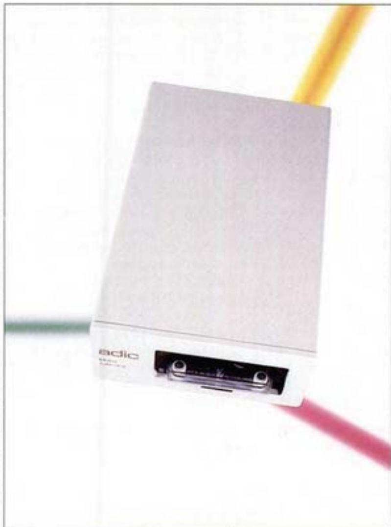
*The ADIC TD-440 is an external 3- by 6½- by 11-inch drive that connects to the host PC through an SCSI interface using an 8-bit interface expansion board. The unit thinks it's a disk drive—it uses familiar DOS commands like COPY and CHKDSK and needs no special software for daily backup.*
