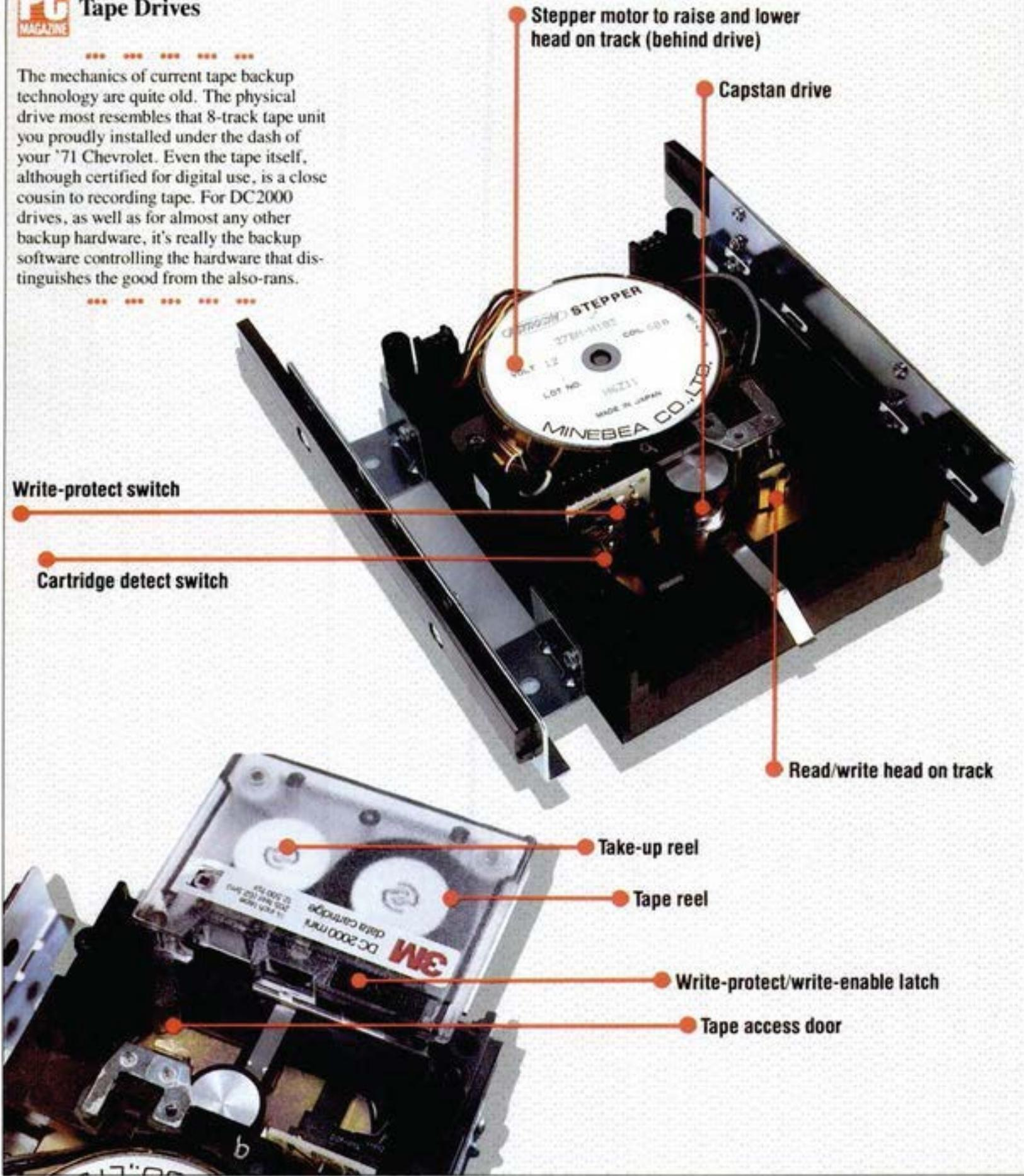
the manufacturers' own accounts, formatting the entire 40-megabyte tape capacity takes half an hour. Even that figure ignores such collateral matters as winding and re-winding the tape and indexing the read/write head.
