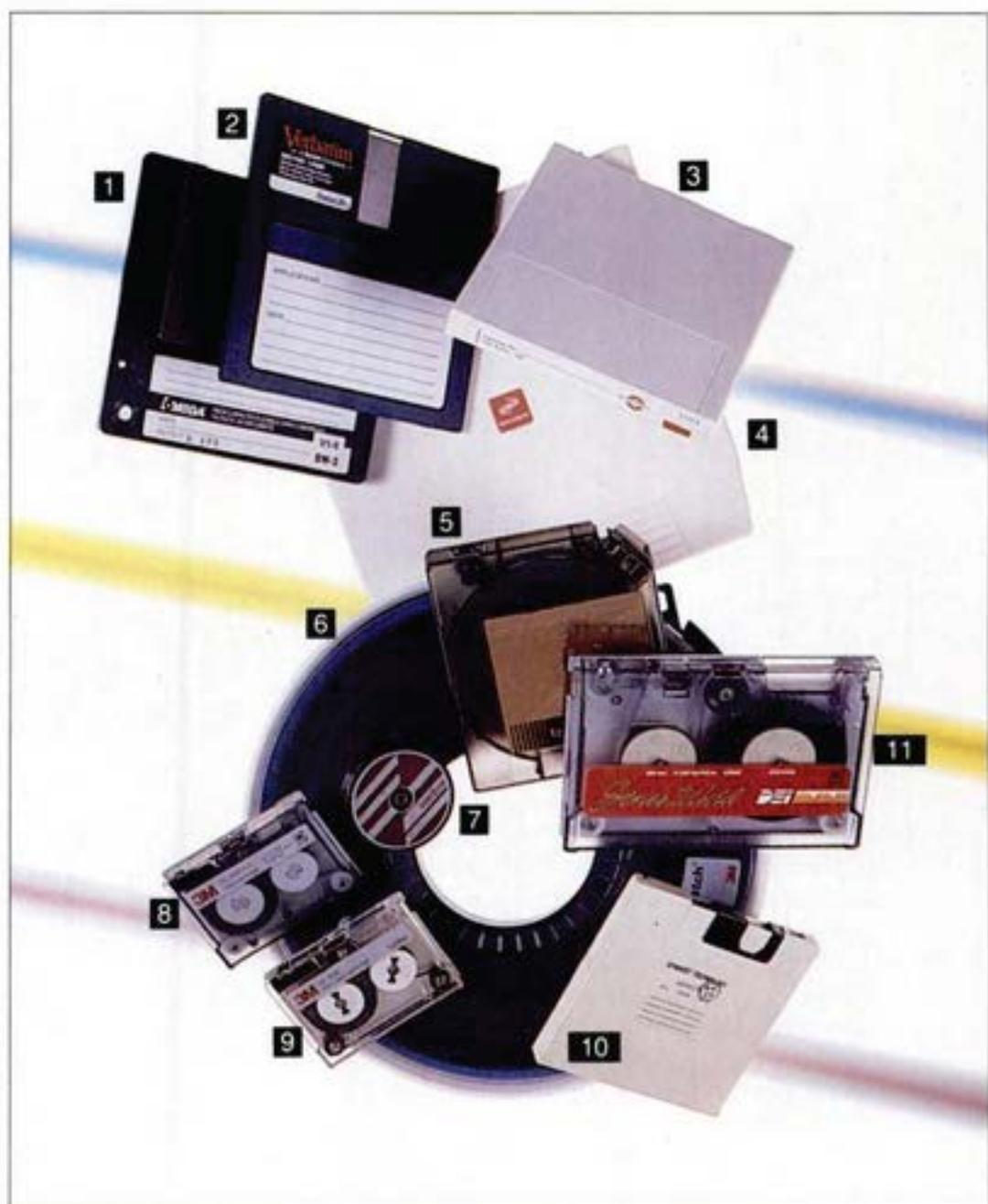
*In addition to DC2000 systems, the options for backing up your data include (1) Iomega's 5 1/4-inch Bernoulli cartridge, (2) Kodak's 12-megabyte cartridge, (3) a Dysan 5 1/4-inch removable Winchester cartridge, (4) Amcodyne's removable cartridge, (5) DEI's 3480 cartridge, (6) a nine-track open-reel tape, (7) Interdyne's spooled tape cartridge, (8 and 9) 3M's DC2000 and DC1000 cartridges, (10) IDE and Systen's removable cartridge, (11) DEI's DC600 cartridge.*
