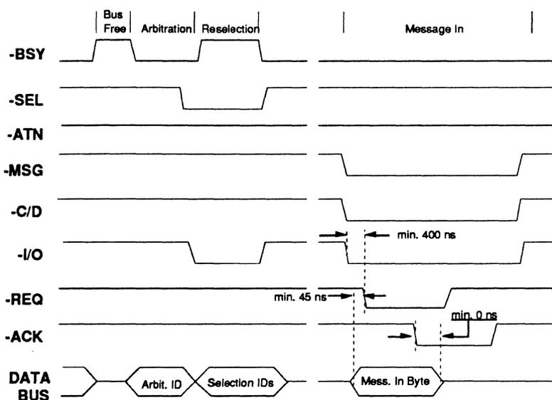
Figure 8.3 Arbitration, Reselection and Message In Phases
