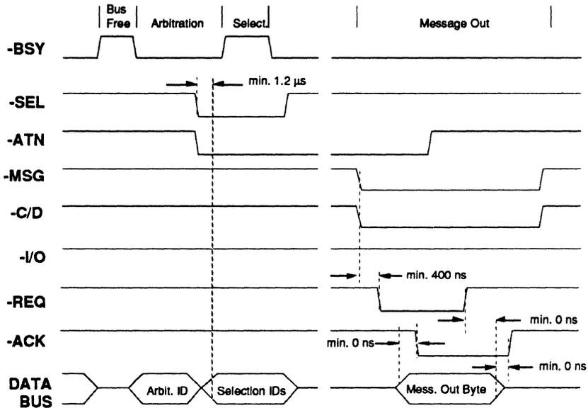
Figure 8.2 Arbitration, Selection and Message Out Phases
