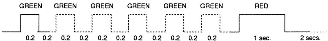
If the test is failing, the RED front LED will blink an eight-bit STM Error Code Message. The most significant bit will be blinked first (a short blink equals logical '0', a long blink equals logical '1').
