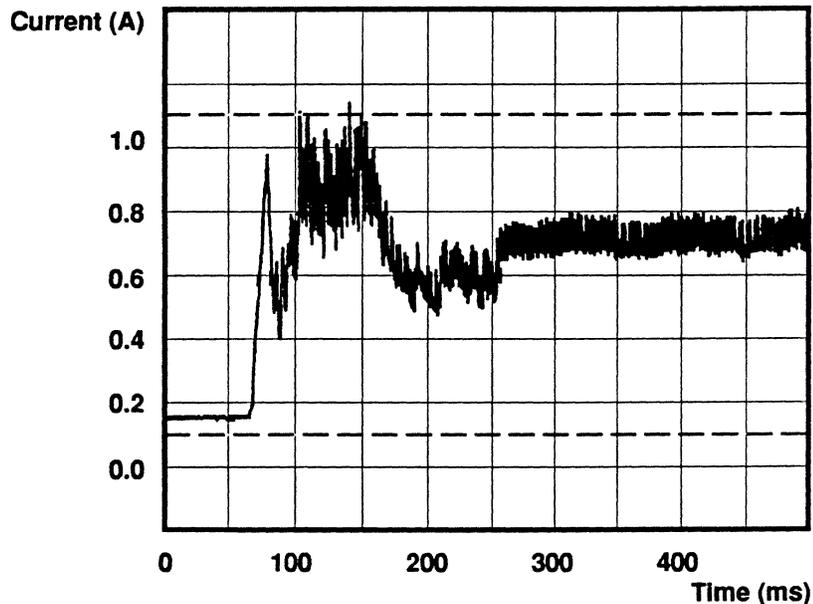
*Typical current curve for the +12 V power supply during capstan-motor start-up (80 ips)*
