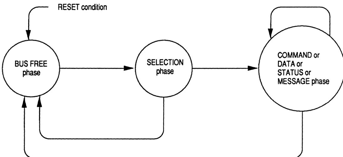
Figure 8.10 Phase Sequencing for non-arbitrating systems
