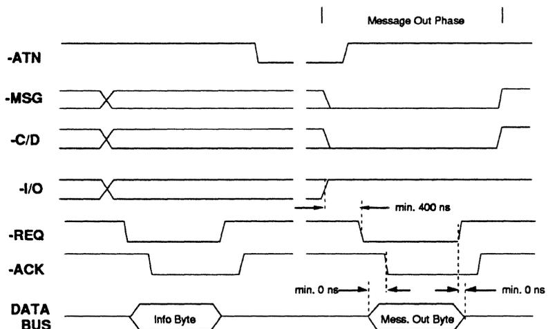
Figure 8.8 Attention Interlock and Message Out Transfer
