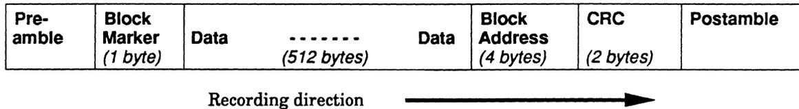
Figure 6.8 Block layout QIC-24/QIC-120/QIC-150
