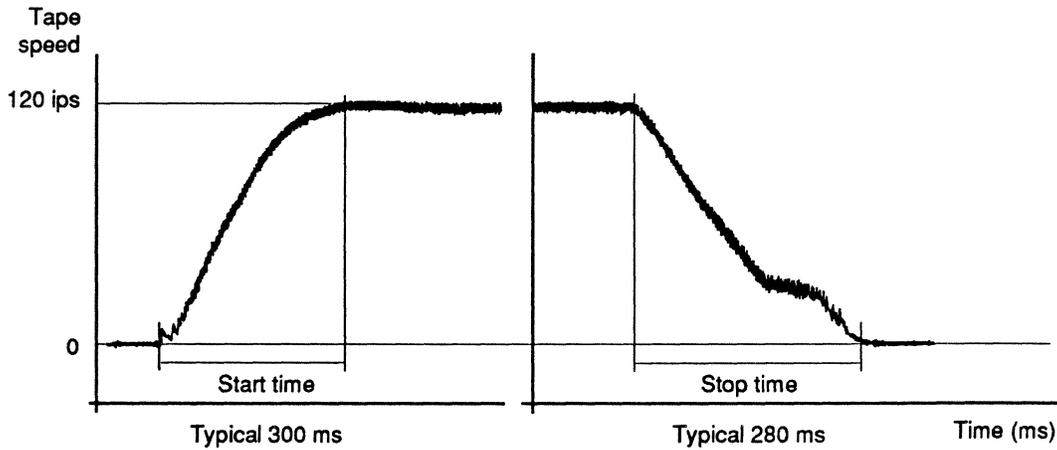
*Typical curves for tape speed during start / stop operations*
