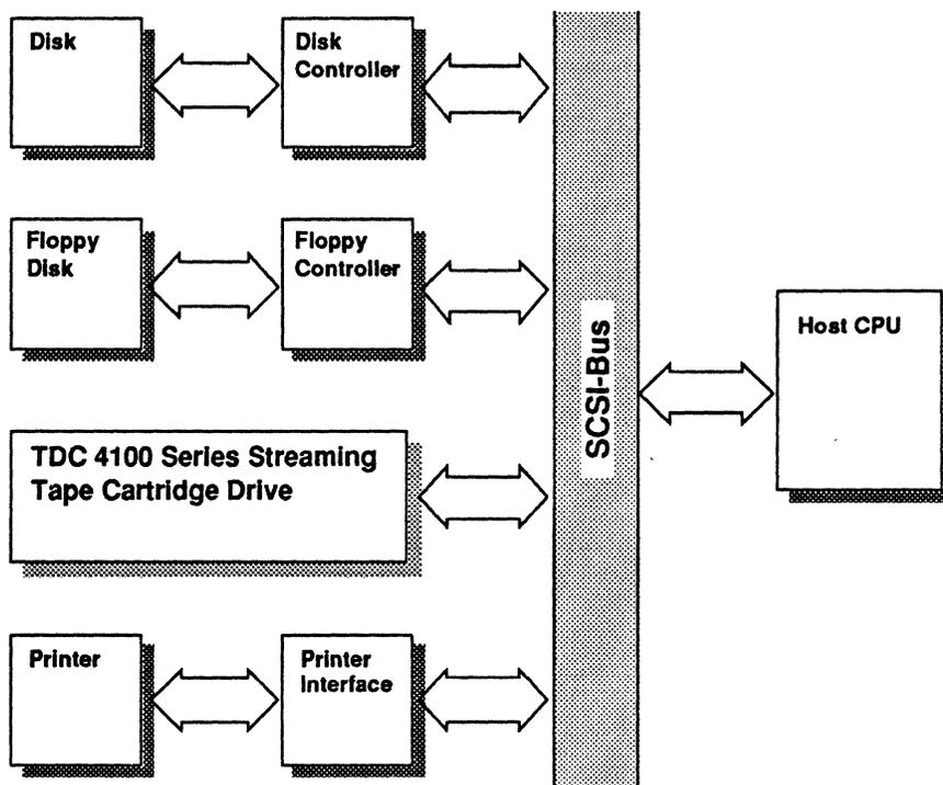
Figure 4.5 Block diagram of a system with SCSI-bus interface
