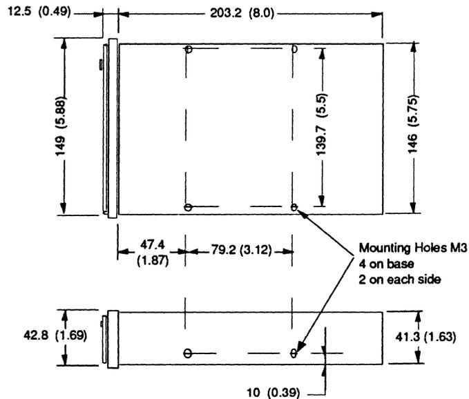
Figure 4.1 Drive Mounting Details (European Projection)
