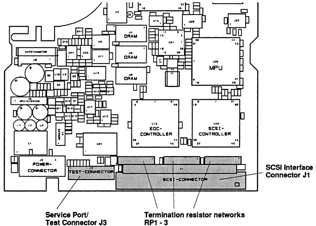
Figure 4.4 The TDC 4100 Mainboard
