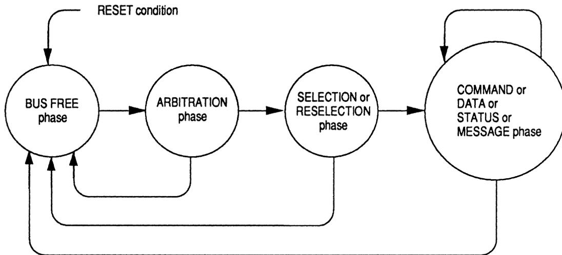
Figure 8.9 Phase Sequencing for systems using Arbitration
