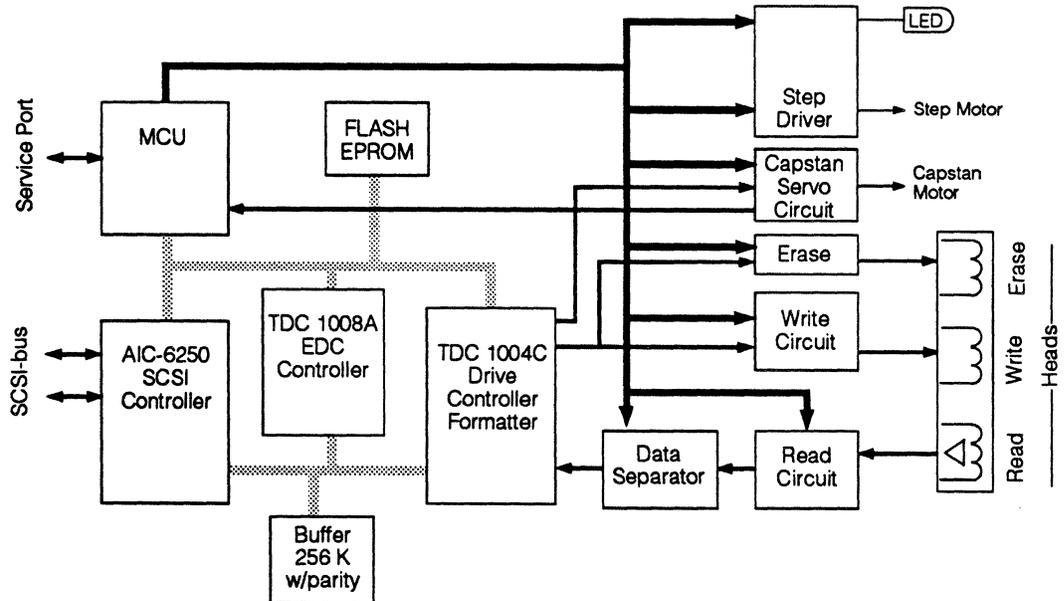
Figure 2.3 Drive block diagram
