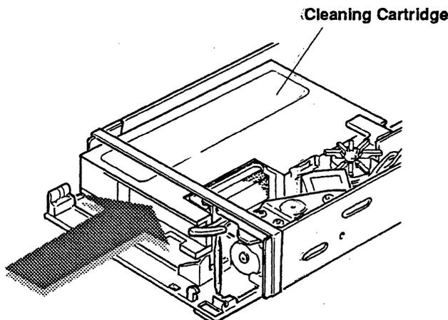
Figure 7.2 Head cleaning using the Cleaning Cartridge Kit
