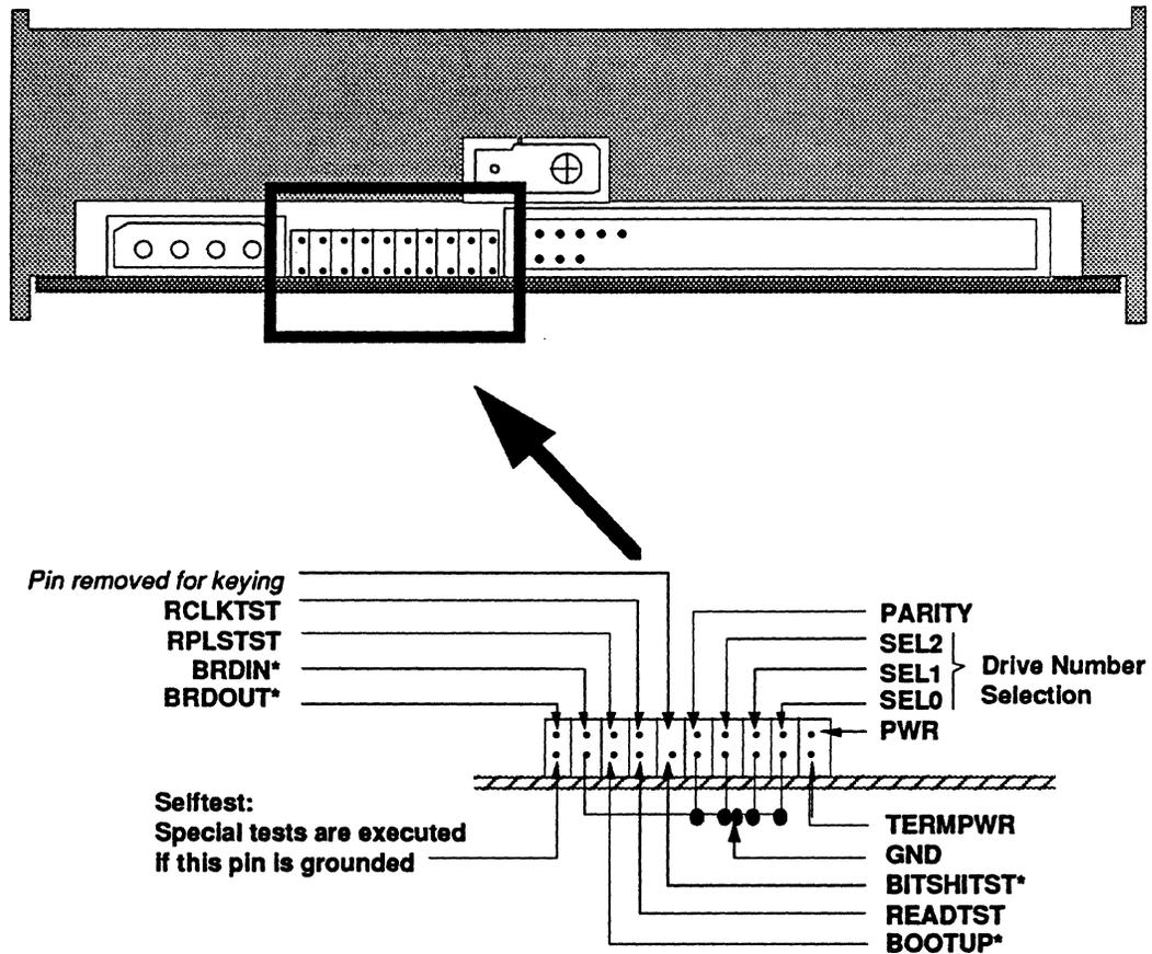
Figure 7.1 Rear view of a TDC 4100 Series Drive showing the Test Connector/Service Port
