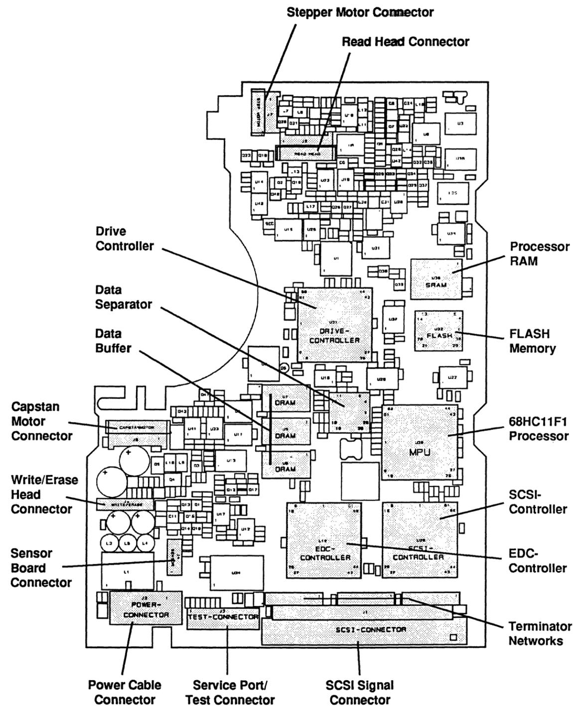
Figure 4.1 SCSI Mainboard Component Location
