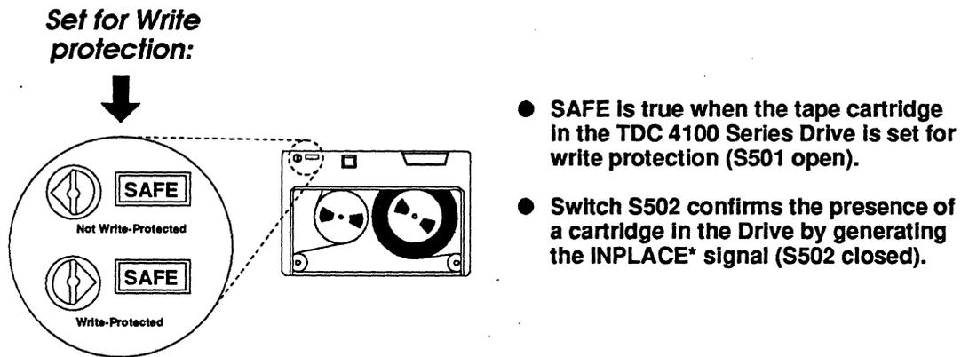
Light from the two light-emitting diodes CR51 and CR52 activates the corresponding photo transistors Q501 and Q502 when a hole in the tape opens the light path. Q501 will detect a hole in the upper part of the tape that results in UPSNS\* being generated. LWSNS\* is generated in the same way when Q502 detects a hole in the lower half of the tape. These signals are analyzed by the processor on the Mainboard in order to determine the position of the tape.
