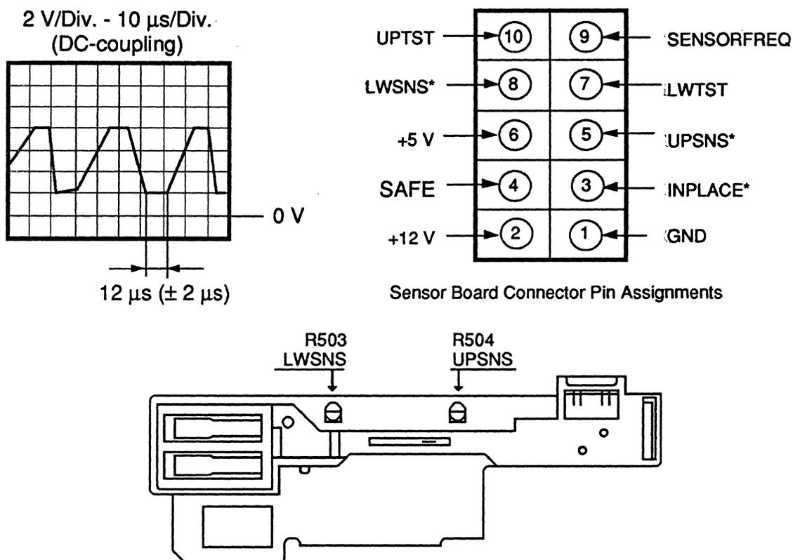
Figure 9.2 Sensor Sensitivity Adjustment
