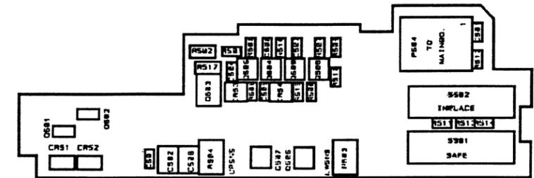
Figure 5.1 Layout of Sensor Board Assembly
