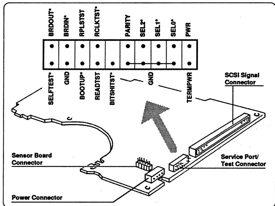
Figure 9.1 Location of Testpoints / Detail of Service Port
