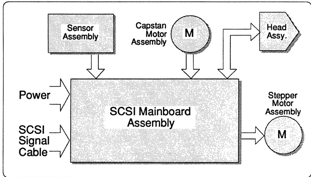
Figure 3.1 Overall Block Diagram
