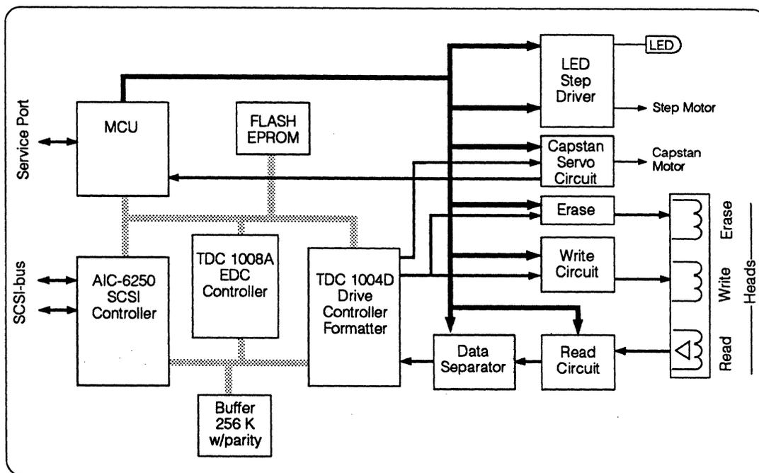
Figure 3.2 TDC 4100 Series Drive Block Diagram
