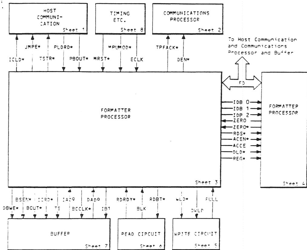
Signal connections between this circuit diagram sheet and other sheets of the Formatter circuit diagram.
