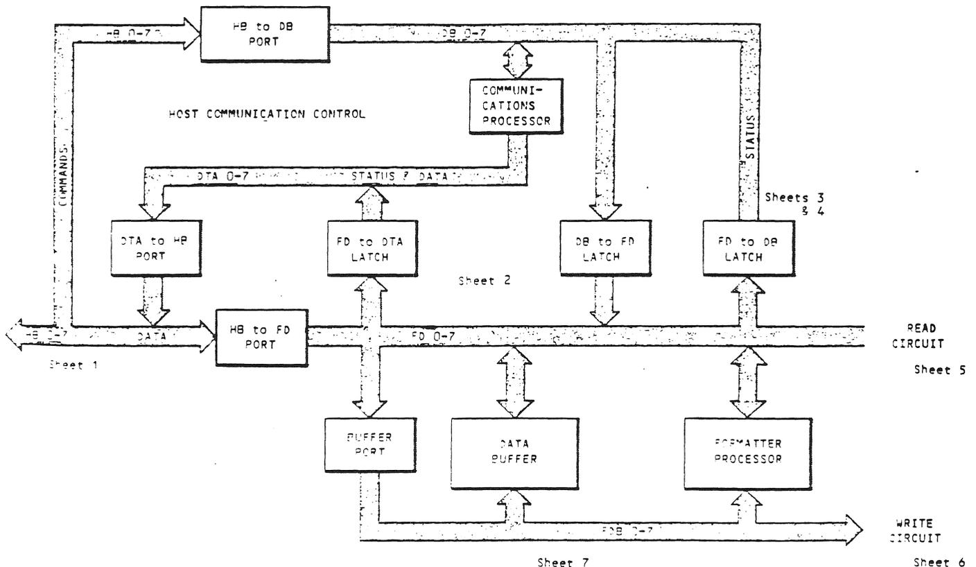
Block diagram of Formatter bus connections.
