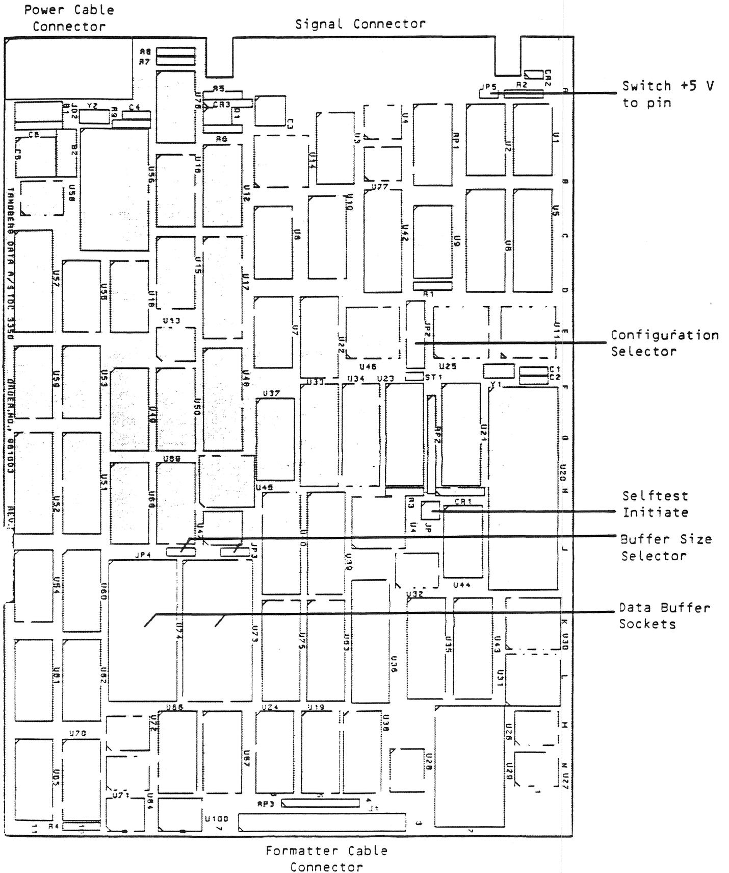
The mnemonics refer to the schematic diagrams for the Formatter Board.
