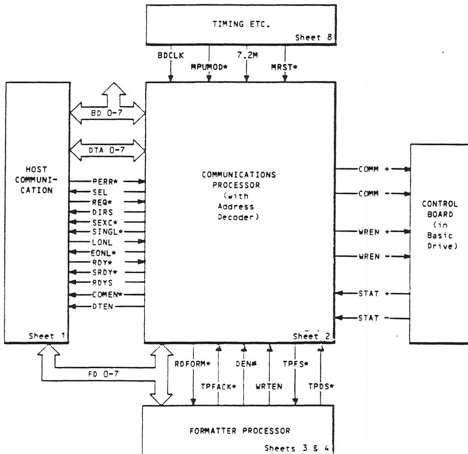
*Signal connections between this circuit diagram sheet and other sheets of the Formatter circuit diagram.*
