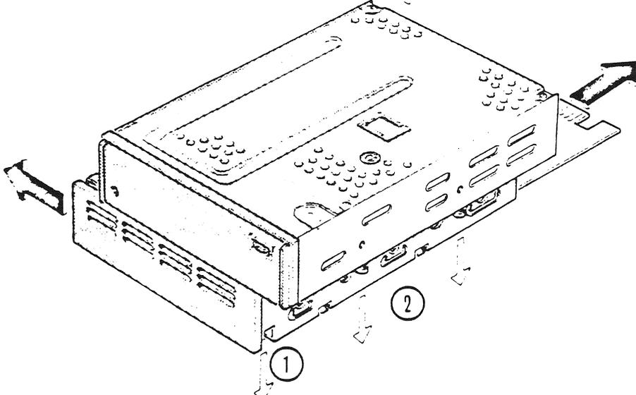
**9.2 Removing the Formatter B from the Drive**
