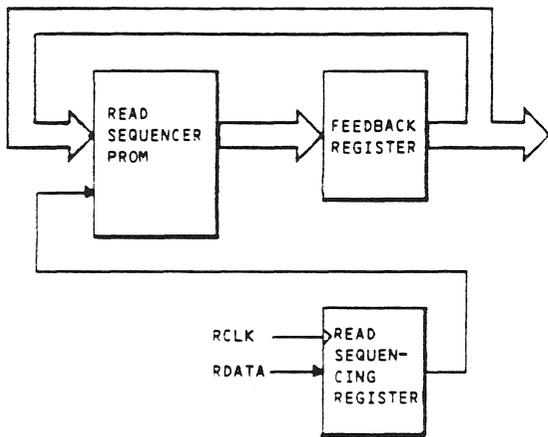
*Simplified diagram of Read Data Synchronizer and Code Converter.*
