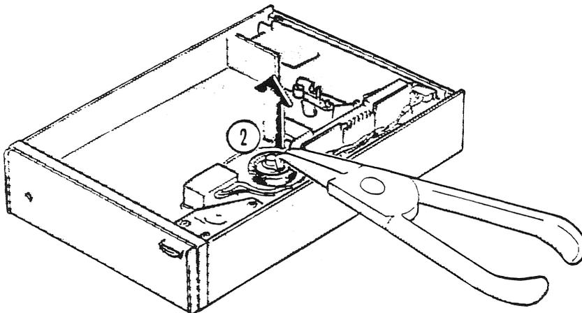
4. Insert a cartridge and adjust the capstan wheel so that it covers the cartridge roller (a and b > 0).
