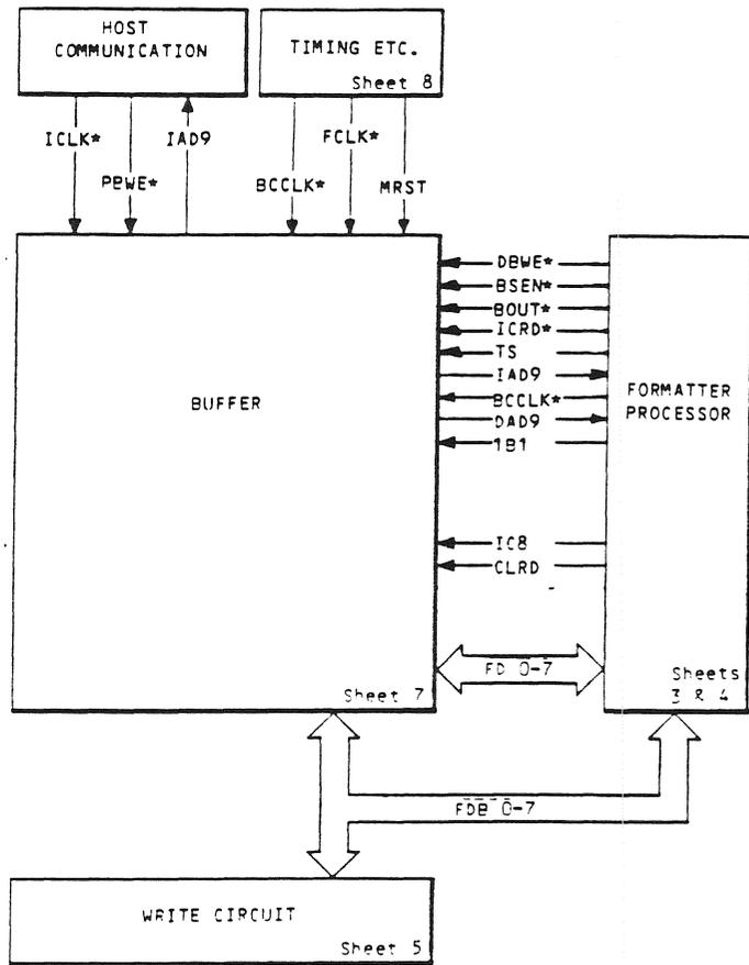
Signal connections between this circuit diagram sheet and other sheets of the Formatter circuit diagram.
