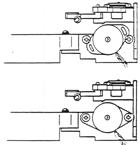
NOTE! Ensure correct orientation of the cable when replacing the motor. Check that the door moves freely when everything has been reassembled.
