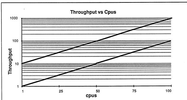
Figure 3. A graph showing the growth in throughput as processors are added to a cluster. The graph shows two families of processors, one capable of unit throughput per cpu and the other capable of 10 units per cpu. Distributed database software provides this kind of linear growth for clustered systems.
