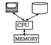
Figure 2.b: The first evolutionary step away from the Von Neumann model: multiple processors share memory. Some of the processors are functionally specialized to do IO while others execute programs. The processors communicate via shared memory and signal wires.
