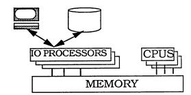
Figure 2.c: The next evolutionary step was to couple multiple independent processors on a high speed local network to form a cluster. The nodes of the cluster do not share memory, rather they communicate via messages. This architecture allows tens or hundreds of processors to be applied to one application. It is the thesis of this article that clusters require a distributed database system to be effective and distributed database transparency should only be used within a cluster.
