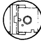
TO AVOID DAMAGE TO THE DISKETTE AND TO YOUR DRIVE, INSERT DISKETTE CAREFULLY UNTIL THE BACKSTOP IS ENCOUNTERED.
