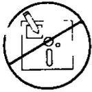
DO NOT WRITE ON THE JACKET WITH PEN OR PENCIL. USE A FELT TIPPED PEN.
