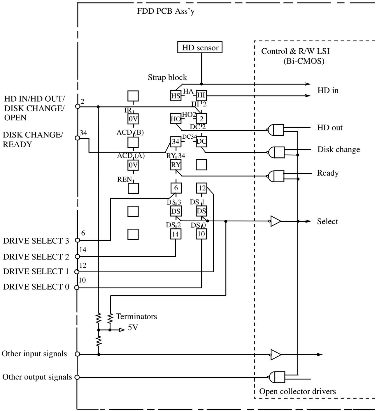
(Fig. 8.2-1) FDD signal interface circuit
