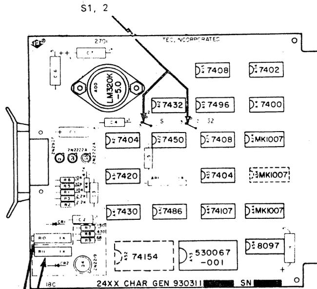
Variable resistor used to vary intensity of protected data in composite video output (optional) Increase lever by turning CW.
