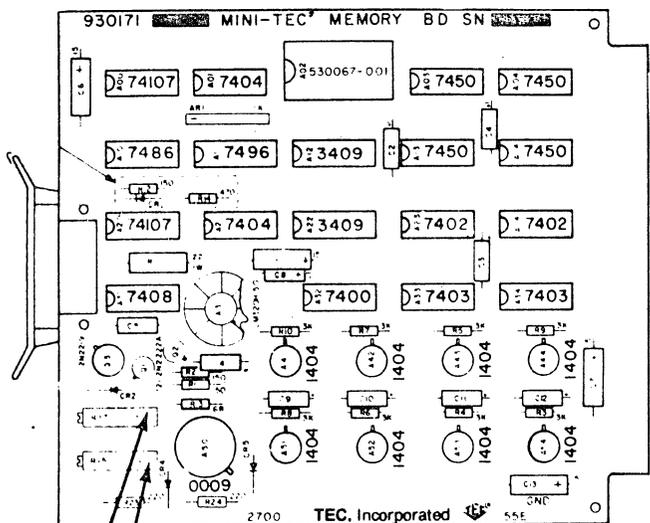
Variable resistor used to vary intensity of protected data in composite video output (optional). Increase level by turning CW.
