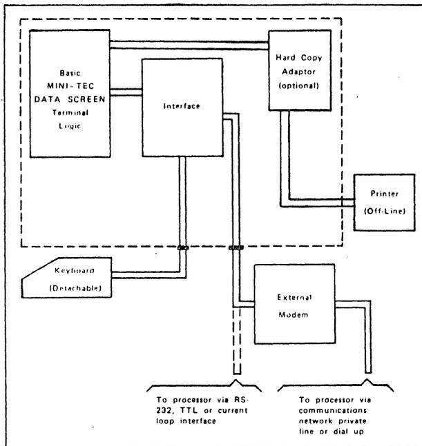
FIGURE 3. BASIC MINI-TEC TERMINAL
