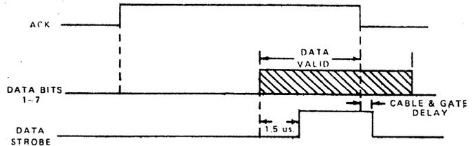
1.44 ms is the maximum transfer rate. Data Strobe will remain high until ACK falls.
