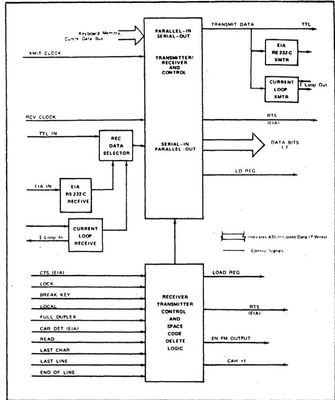
**FIGURE 30 FUNCTIONAL DIAGRAM - SERIAL I/O PCB**
