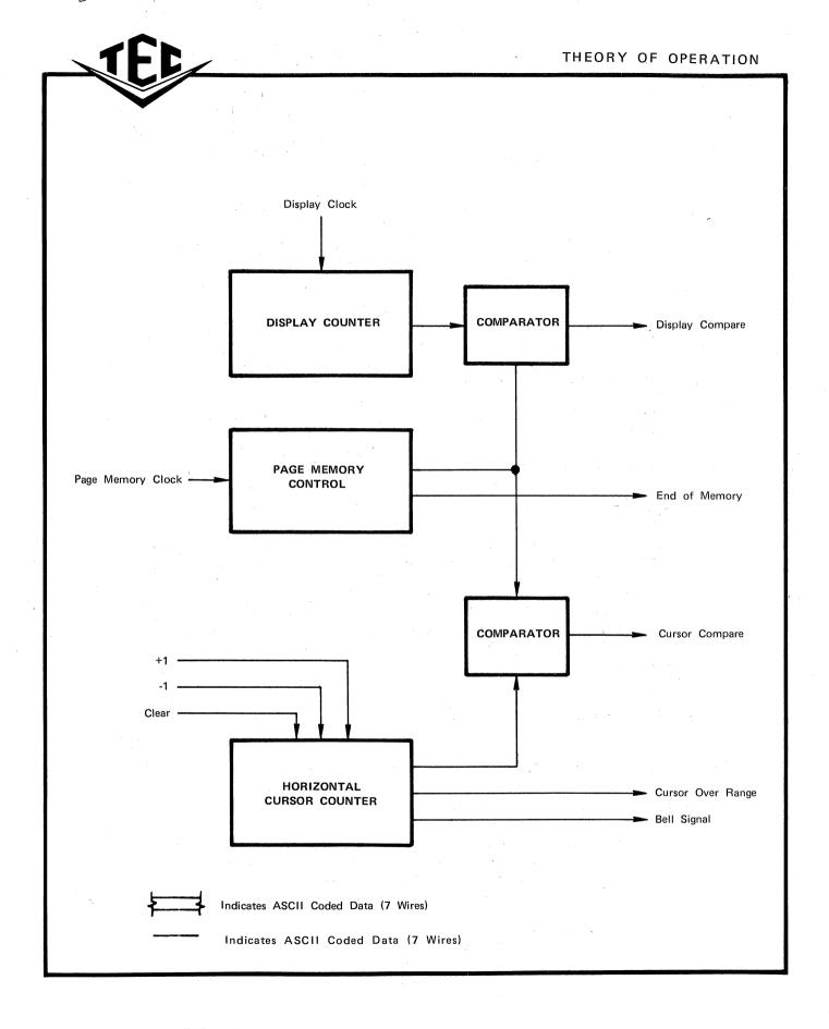
FIGURE 11 FUNCTIONAL DIAGRAM - PAGE CONTROL
