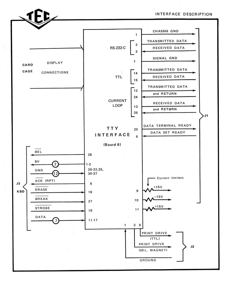
FIGURE 15 MODEL 440 TTY INTERFACE CONNECTIONS
