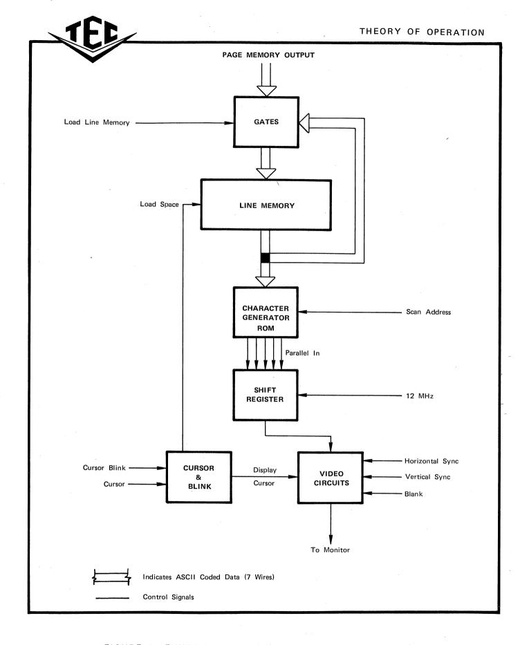
FIGURE 9 FUNCTIONAL DIAGRAM - CHARACTER GENERATOR
