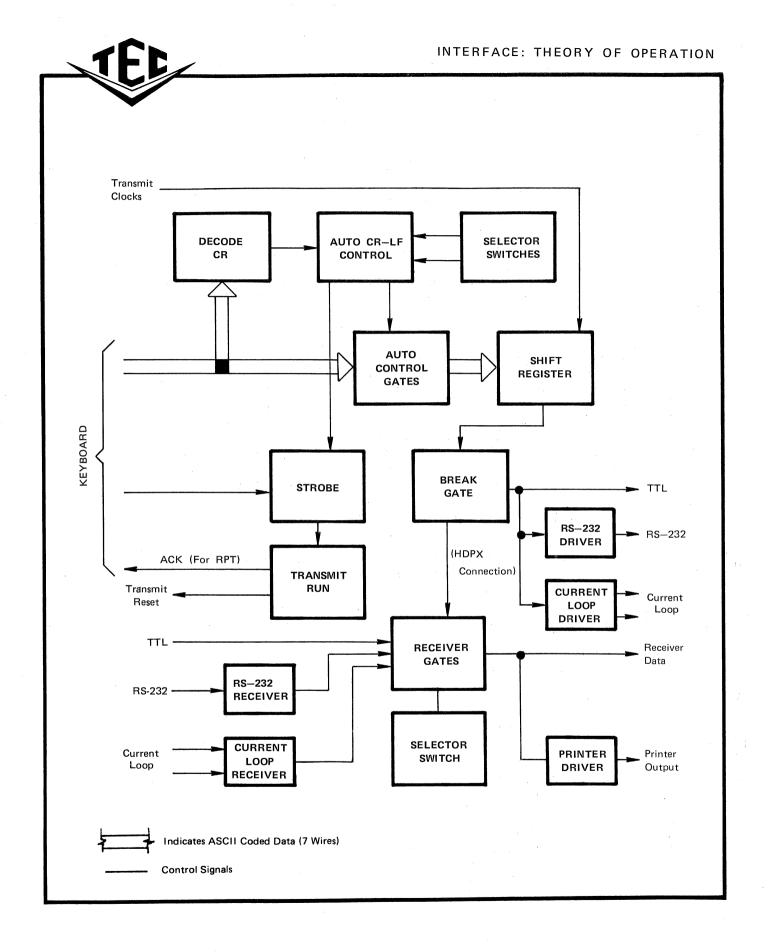
FIGURE 13 FUNCTIONAL DIAGRAM - TTY INTERFACE
