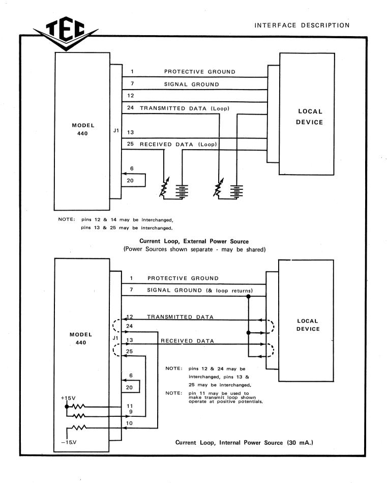
FIGURE 19 TYPICAL INTERFACE CONNECTIONS (CON'T)
