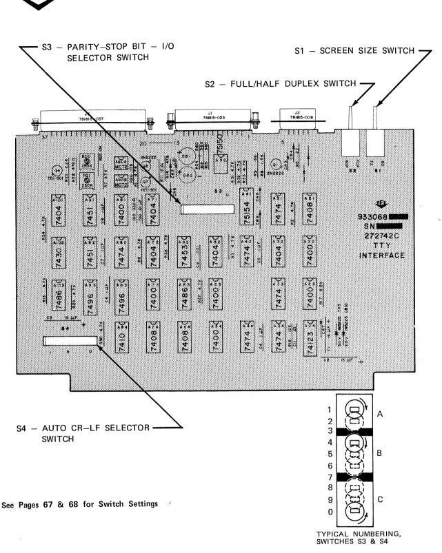
FIGURE 25 MODEL 440 OPTION SELECTIONS-TTY INTERFACE PCB
