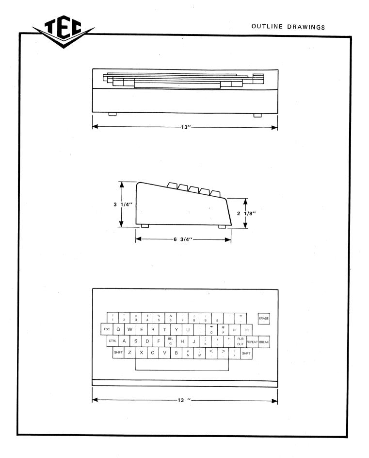
FIGURE 29 DIMENSIONS, MODEL 440 KEYBOARD
