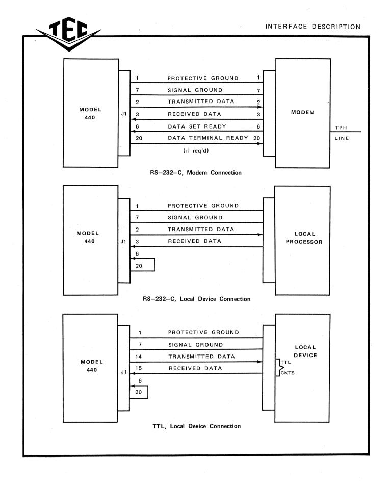
FIGURE 18 TYPICAL INTERFACE CONNECTIONS
