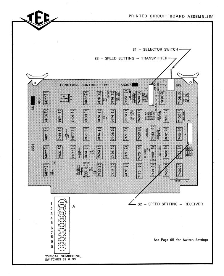
FIGURE 24 MODEL 440 OPTION SELECTIONS— FUNCTION CONTROL PCB
