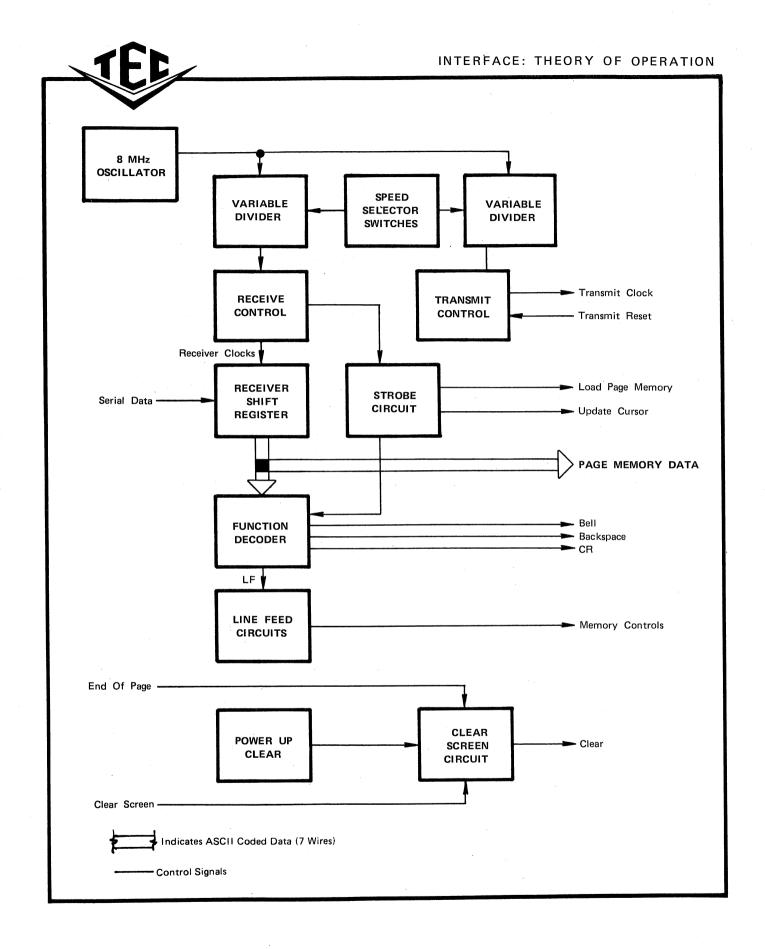
FIGURE 12 FUNCTIONAL DIAGRAM - FUNCTION CONTROL
