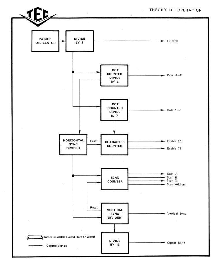
FIGURE 8 FUNCTIONAL DIAGRAM - TIMING GENERATOR
