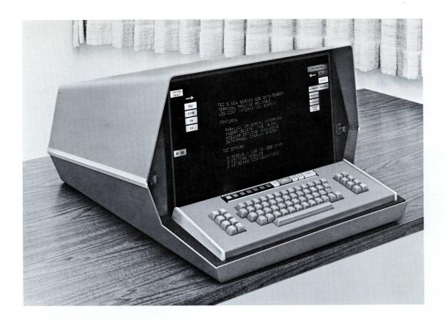
Series 500 Terminals are completely self-contained in an attractive, functional enclosure and utilize a 12-inch, rectangular CRT display tube, a display buffer and refresh memory, control and editing logic, input/output interface adaptor, and an optional electronic keyboard.
