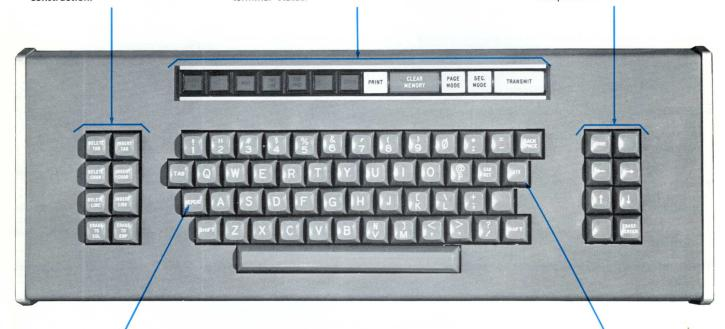
REPEAT key provides repetitive entry of any character or cursor movement. TEC's compact electronic keyboard is arranged in standard typewriter configuration for alphanumeric characters.
