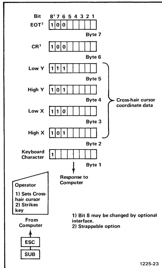
Fig. 3-11. 4010 response to computer command and operator control.
