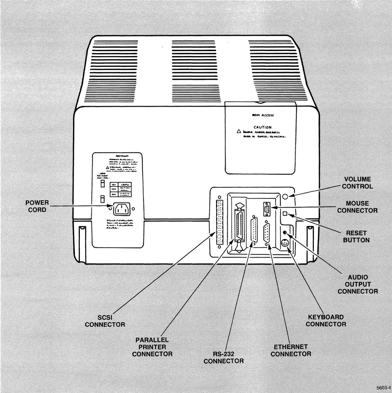
Figure 1-4. Display/CPU Rear Panel.
