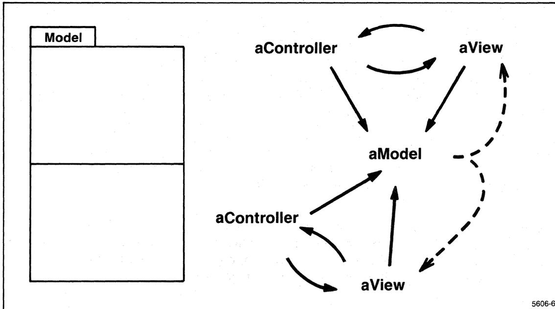
Figure 6. Double Window With Two Model-View-Controllers.
