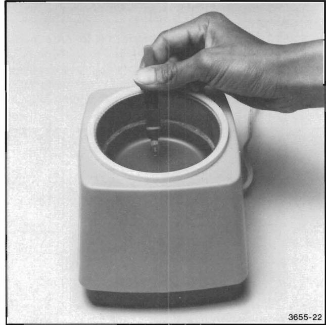
Figure 4-12. Using the Ultrasonic Tank to Clean Pen Tips.
