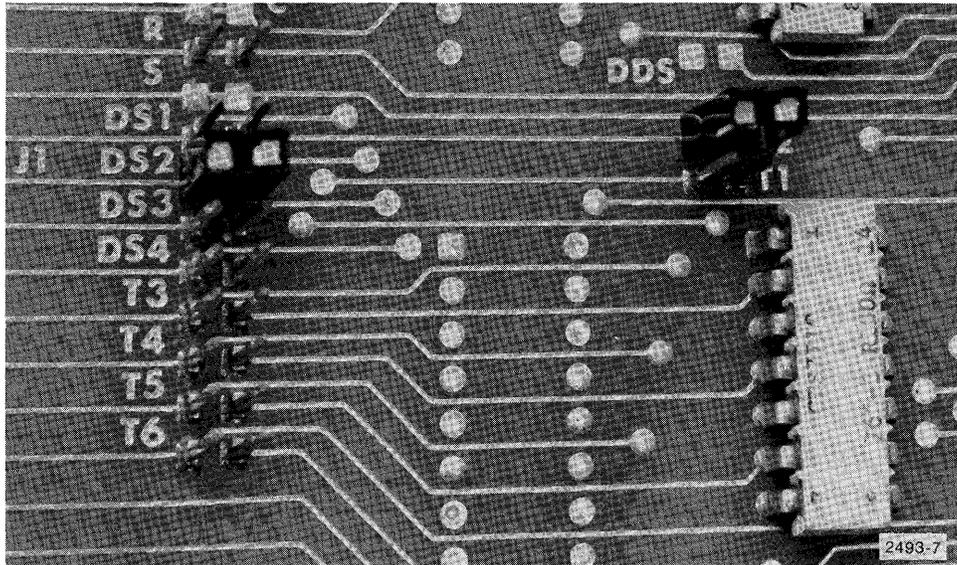
**Figure 3-4. Setting for device address 1 (DS2).**
