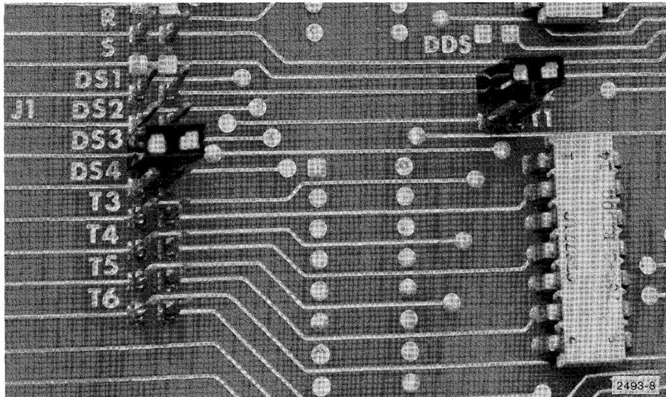
**Figure 3-5. Setting for device address 2 (DS3).**
