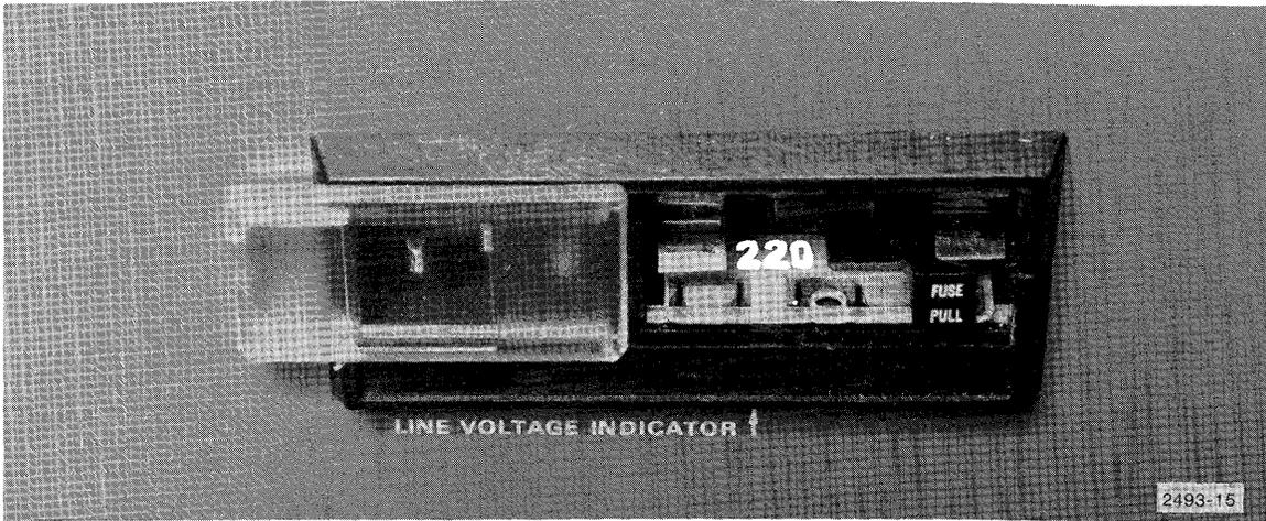
**Figure 3-12. Card position for 220 V.**
