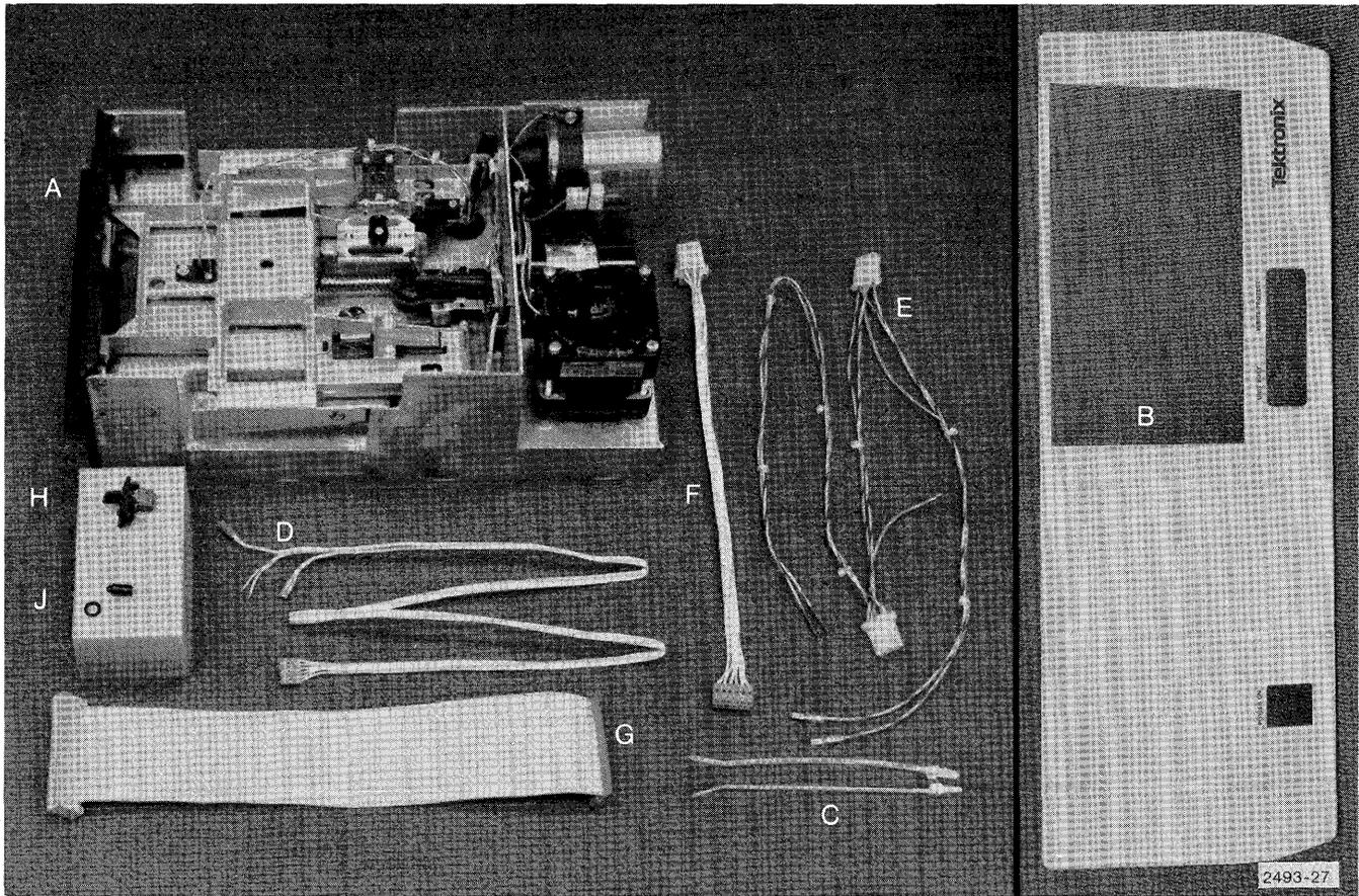
Figure 7-1. Field upgrade kit components.
