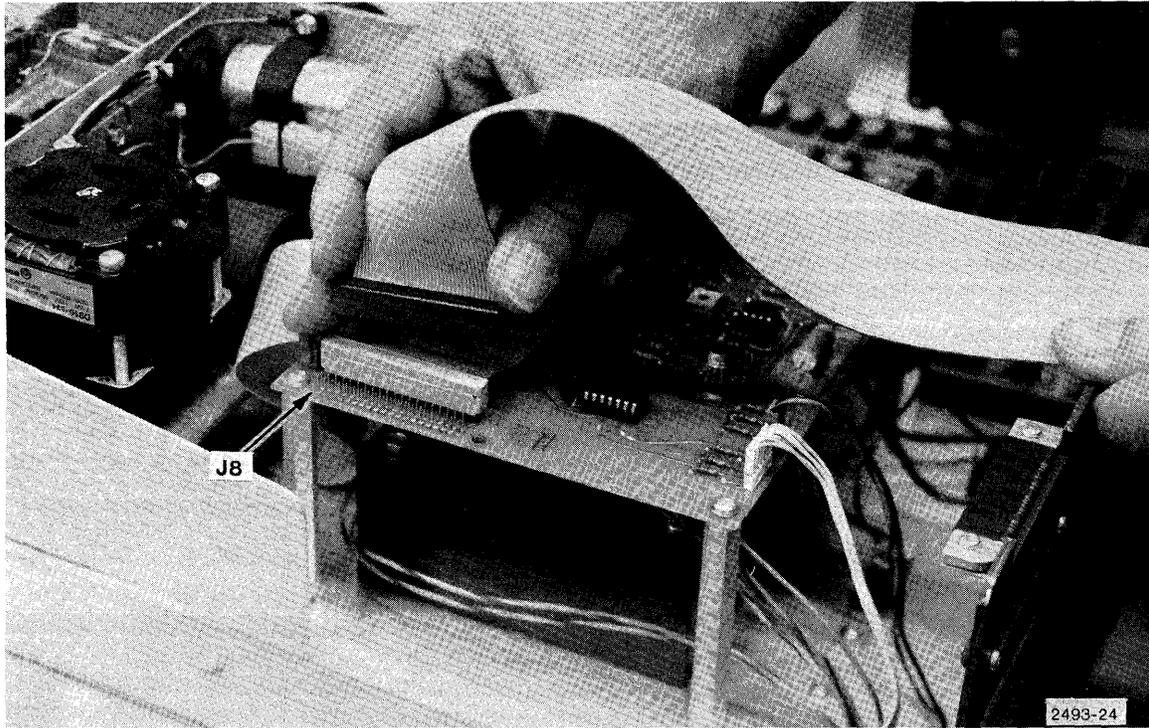
Figure 5-2. Connecting ribbon cable to J-8.
