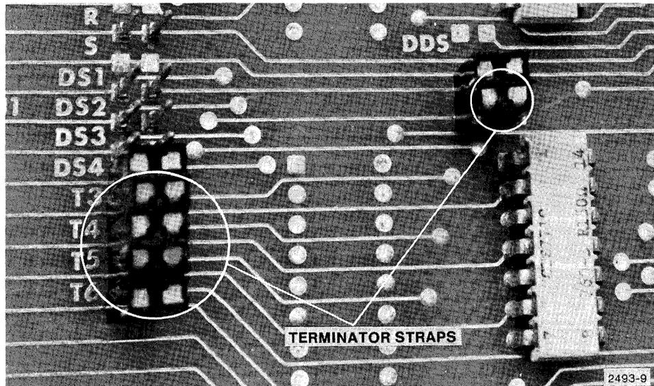
Figure 3-6. Setting for device address 3\* (DS4).
