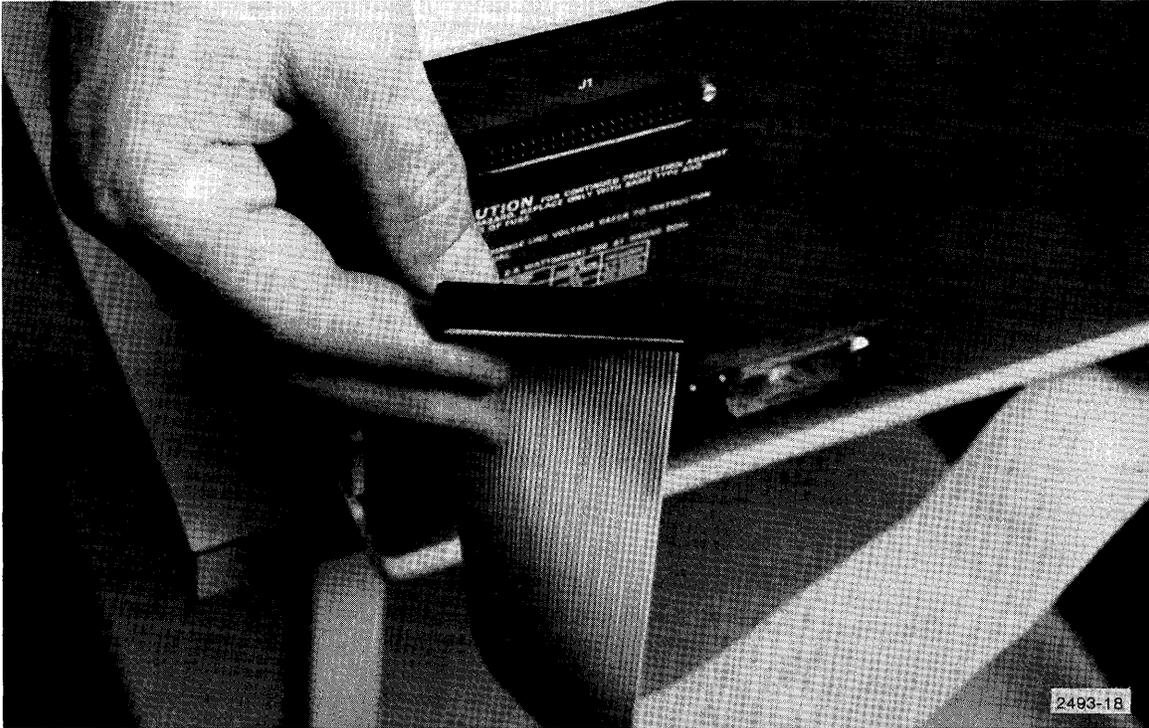
**Figure 3-15. Plugging ribbon cable to connector J-1 on auxiliary cabinet.**
