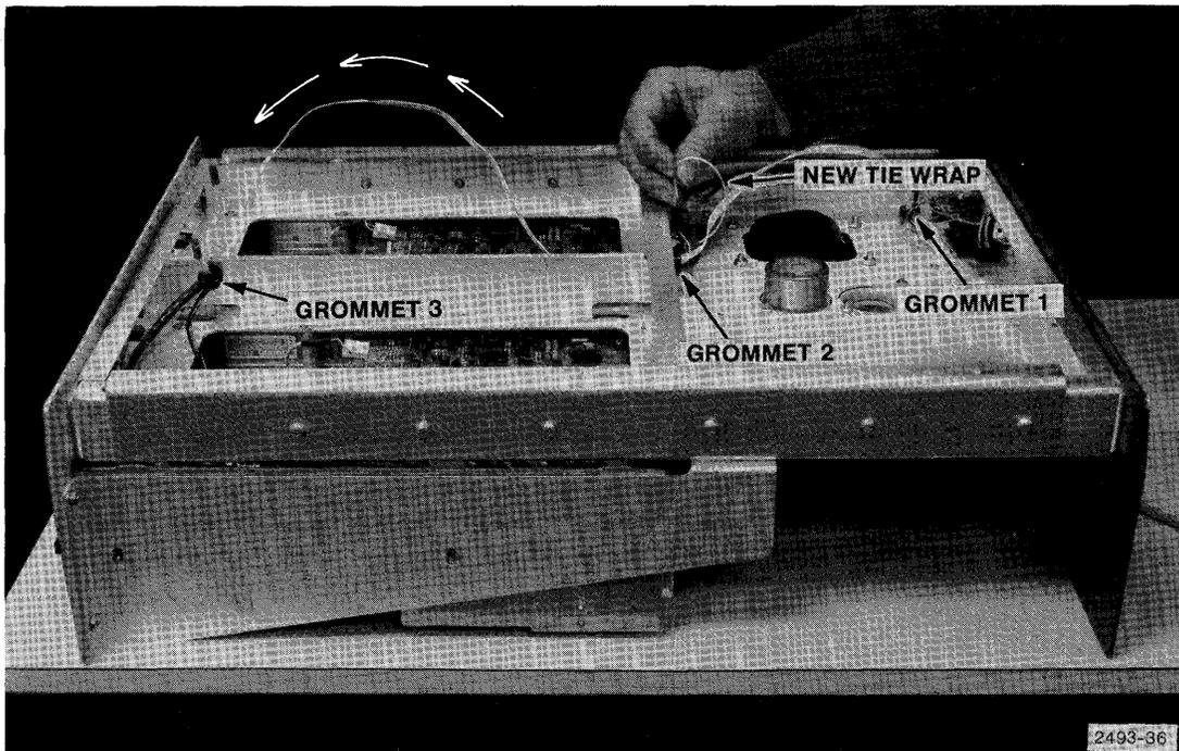
Figure 7-10. Threading ribbon cable D through grommets in cabinet chassis.
