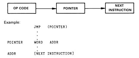
Indexed Indirect Addressing. Instructions using indexed indirect addressing have two bytes. The first byte contains the op code. The second byte contains the address of a table of pointers on page zero. Index register X selects a 16-bit address (pointer) from this table and that address points to the operand.
