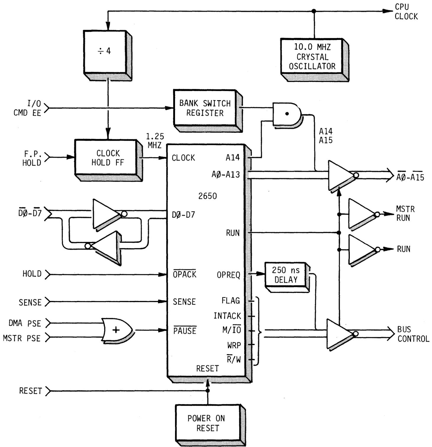
FIGURE 3-2 2650 PROCESSOR AND SUPPORT
