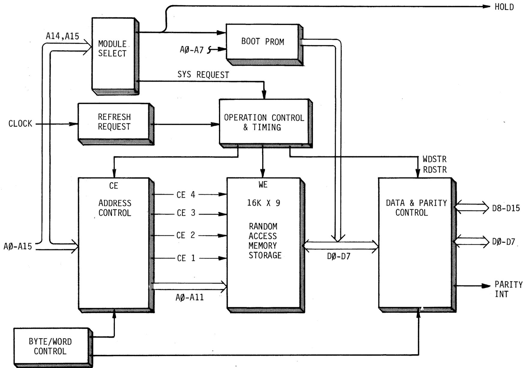
FIGURE 6-1 16K DYNAMIC RAM SIMPLIFIED BLOCK DIAGRAM
