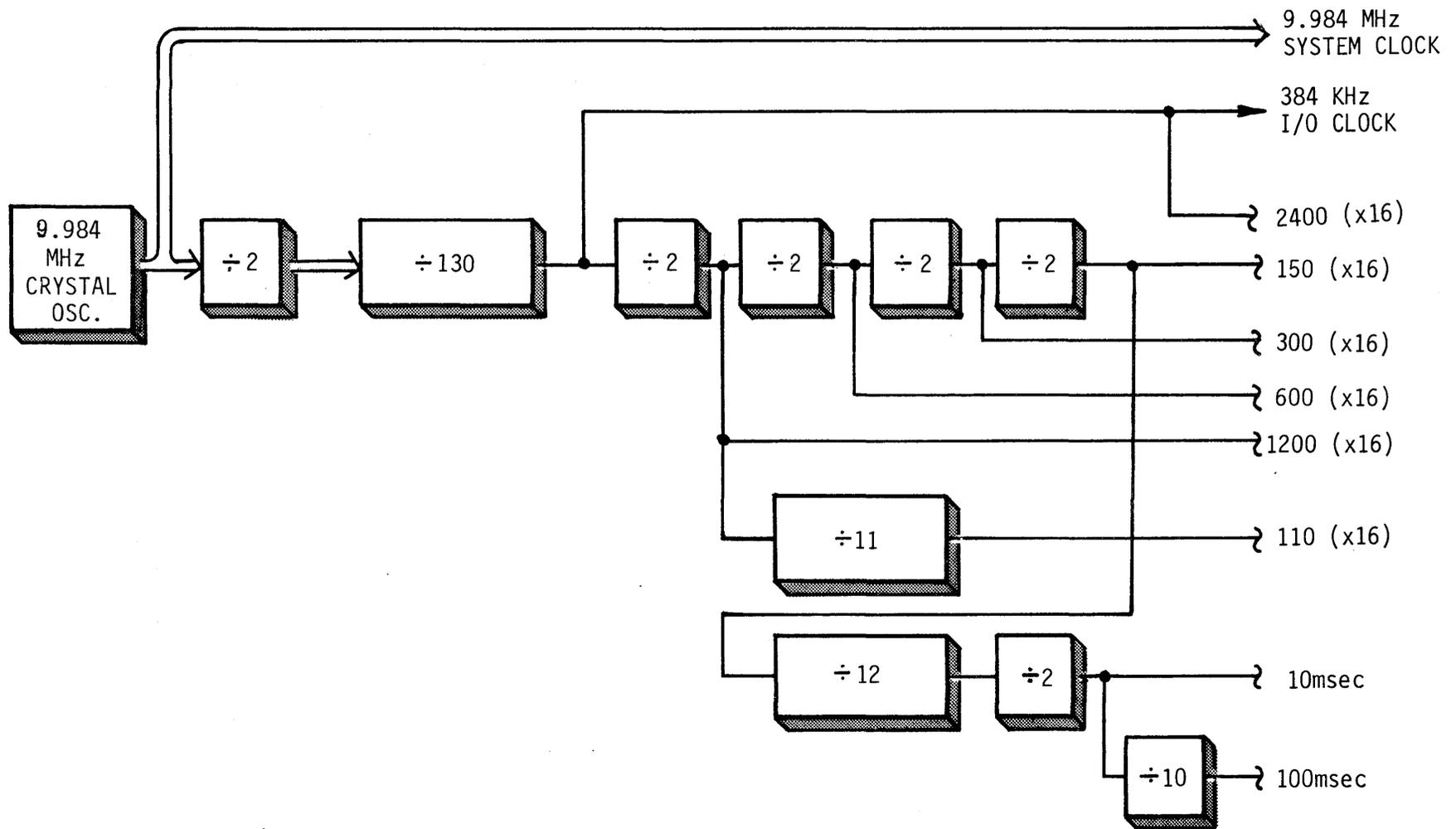
FIGURE 3-12 BAUD RATE AND TIMER LOGIC
