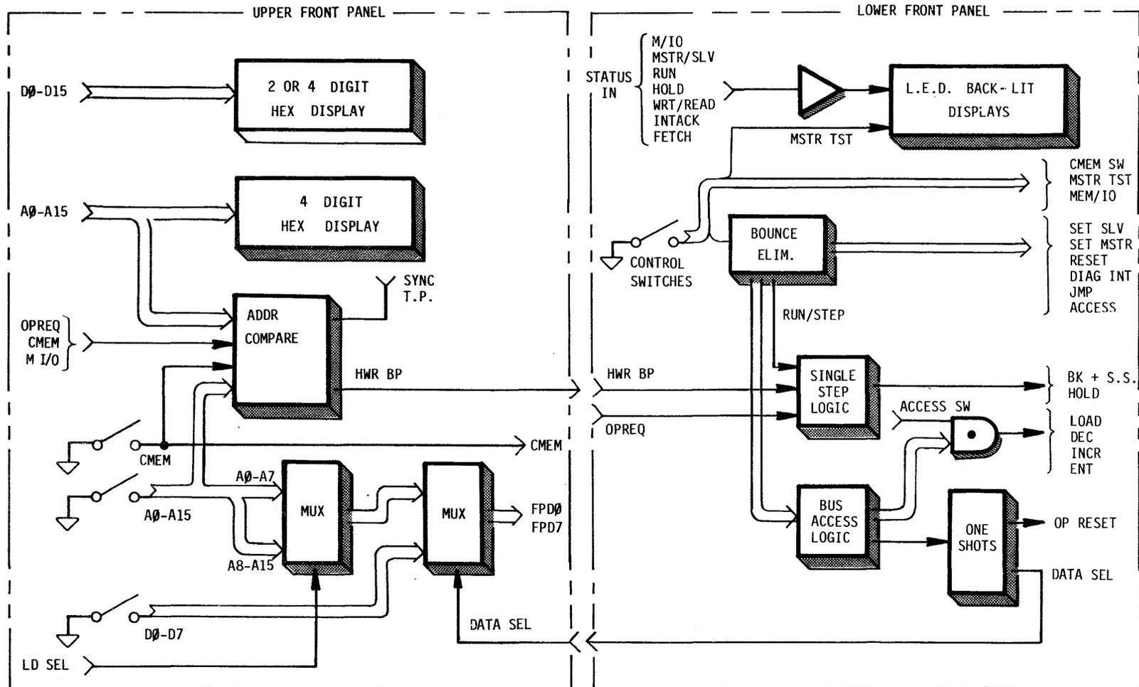
FIGURE 10-2 FULL DISPLAY FRONT PANEL BLOCK DIAGRAM
