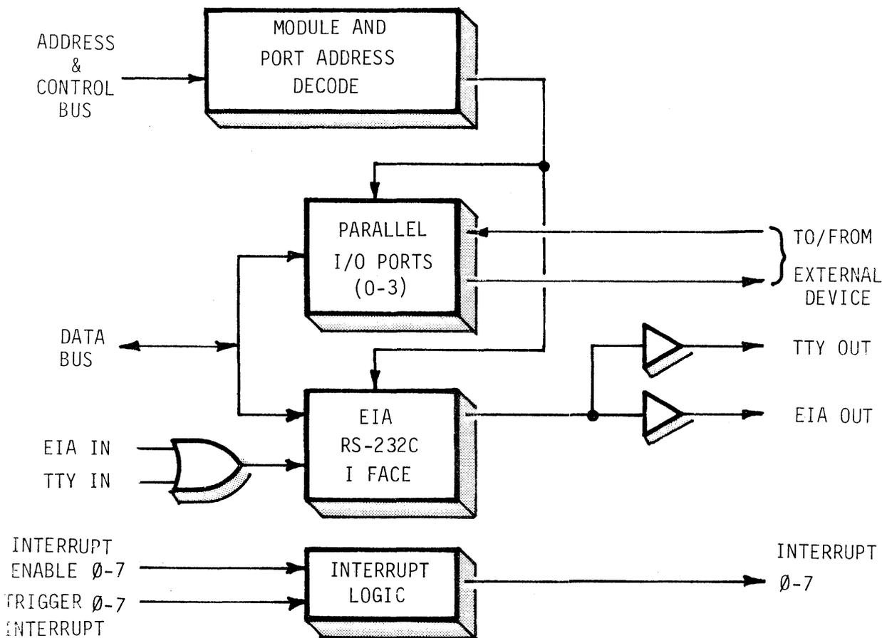
FIGURE 7-1 GP I/O SIMPLIFIED BLOCK DIAGRAM
