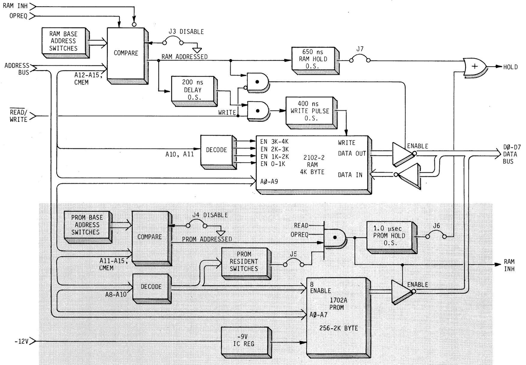
FIGURE 5-1 RAM/PROM MODULE BLOCK DIAGM
