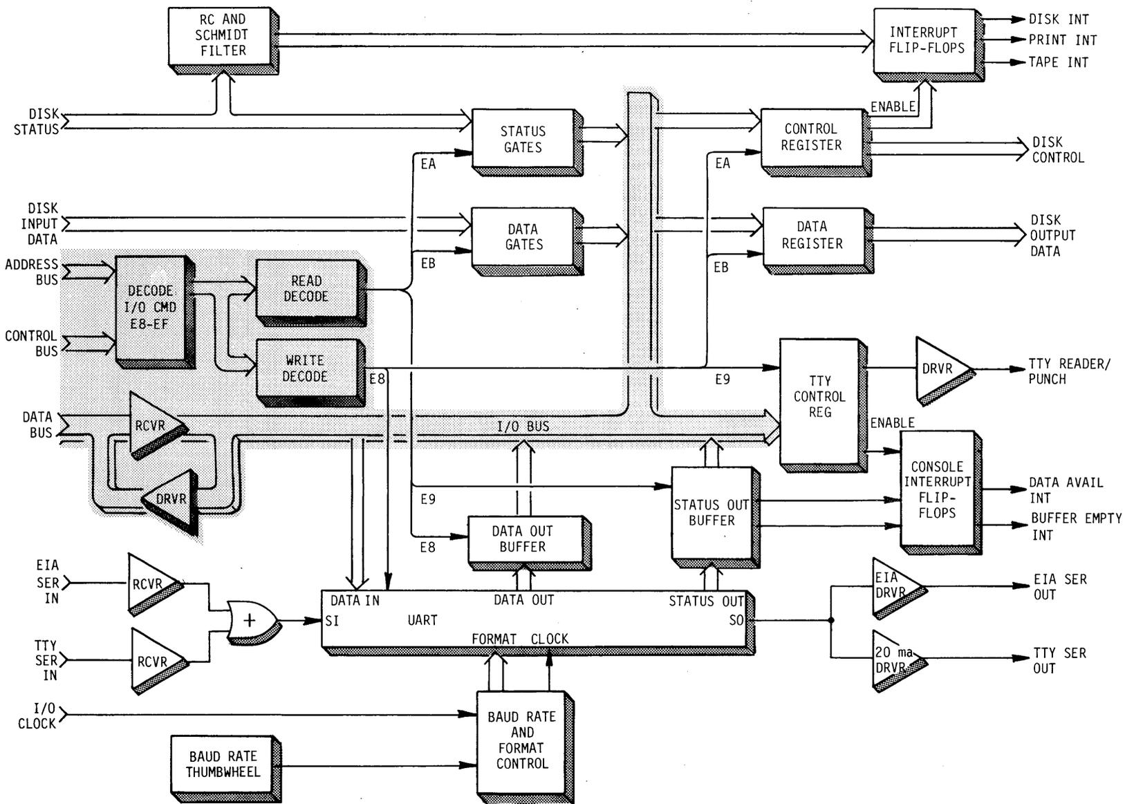
FIGURE 3-9 MASTER CPU I/O DECODING BLOCK DIAGRAM
