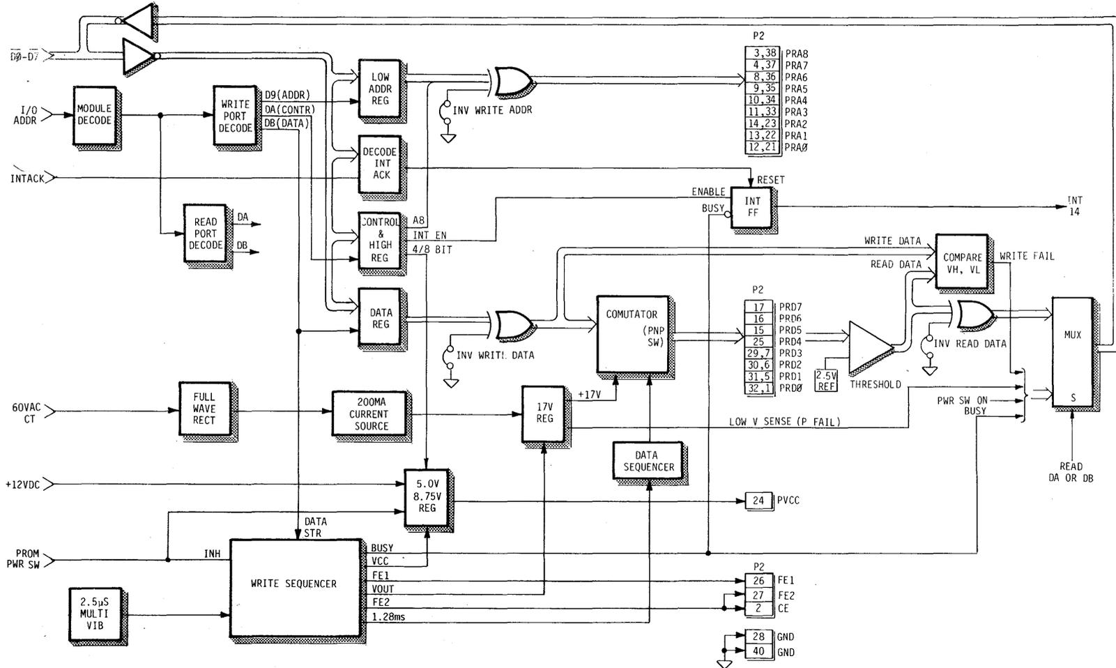
FIGURE 8-7 82S115 PROMGRAMMER BLOCK DIAGRAM
