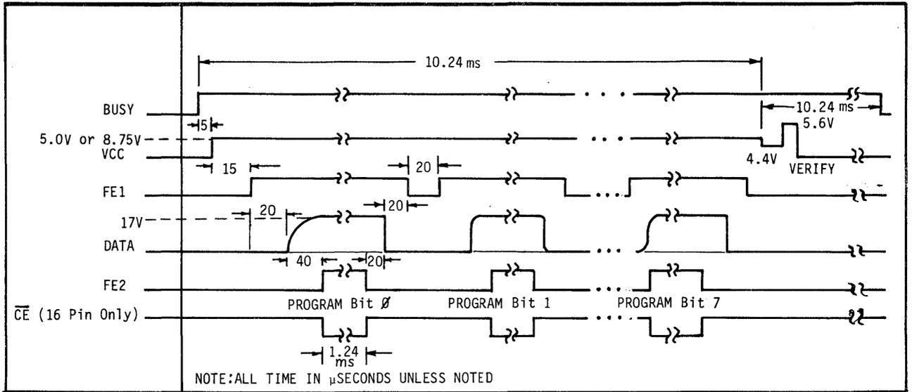
FIGURE 8-9 82S115 WRITE SEQUENCER TIMING DIAGRAM
