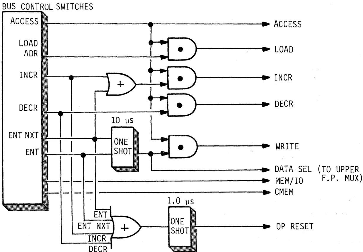
FIGURE 10-4 BUS ACCESS LOGIC
