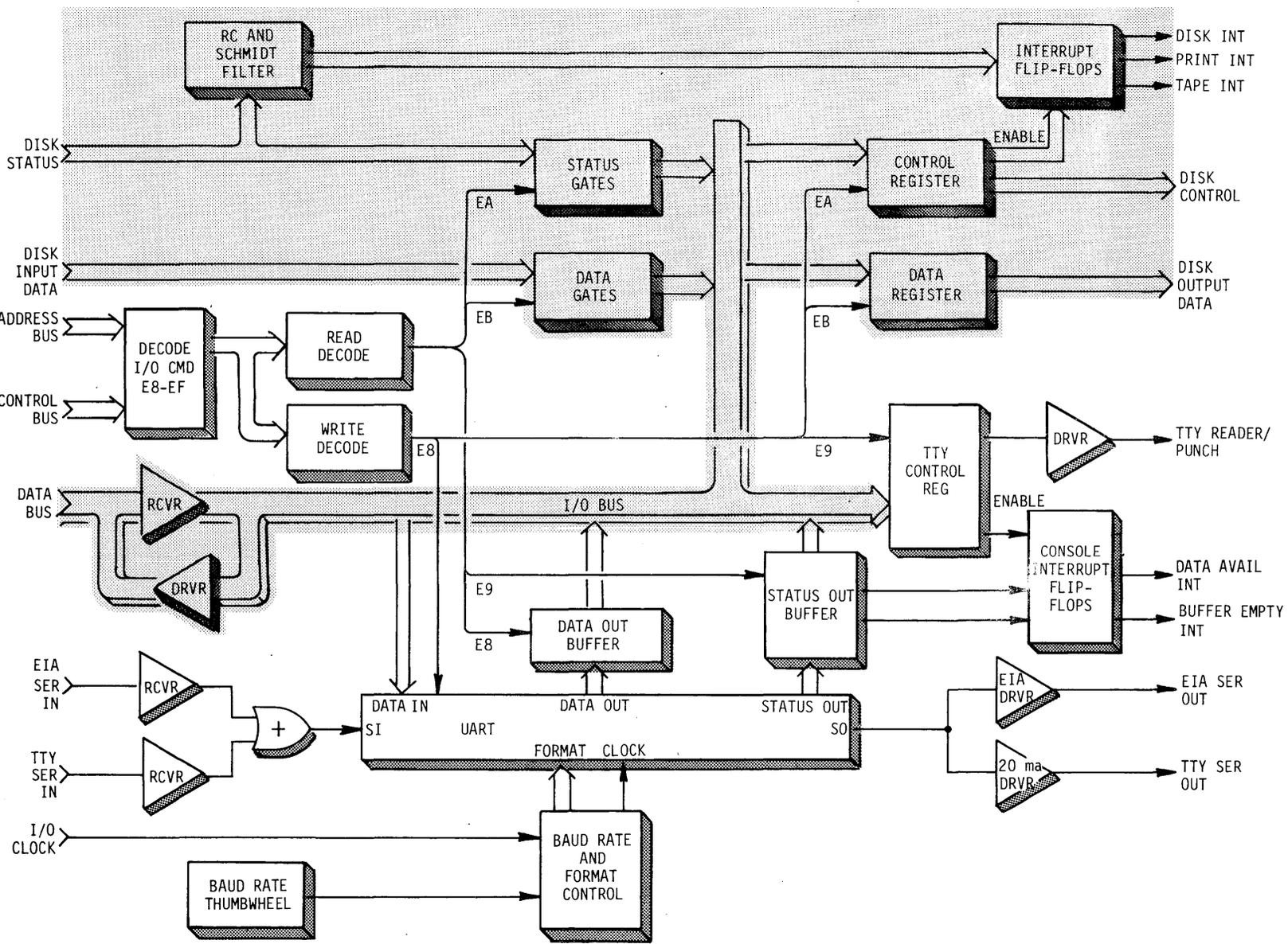
FIGURE 3-7 MASTER CPU DISK I/O BLOCK DIAGRAM
