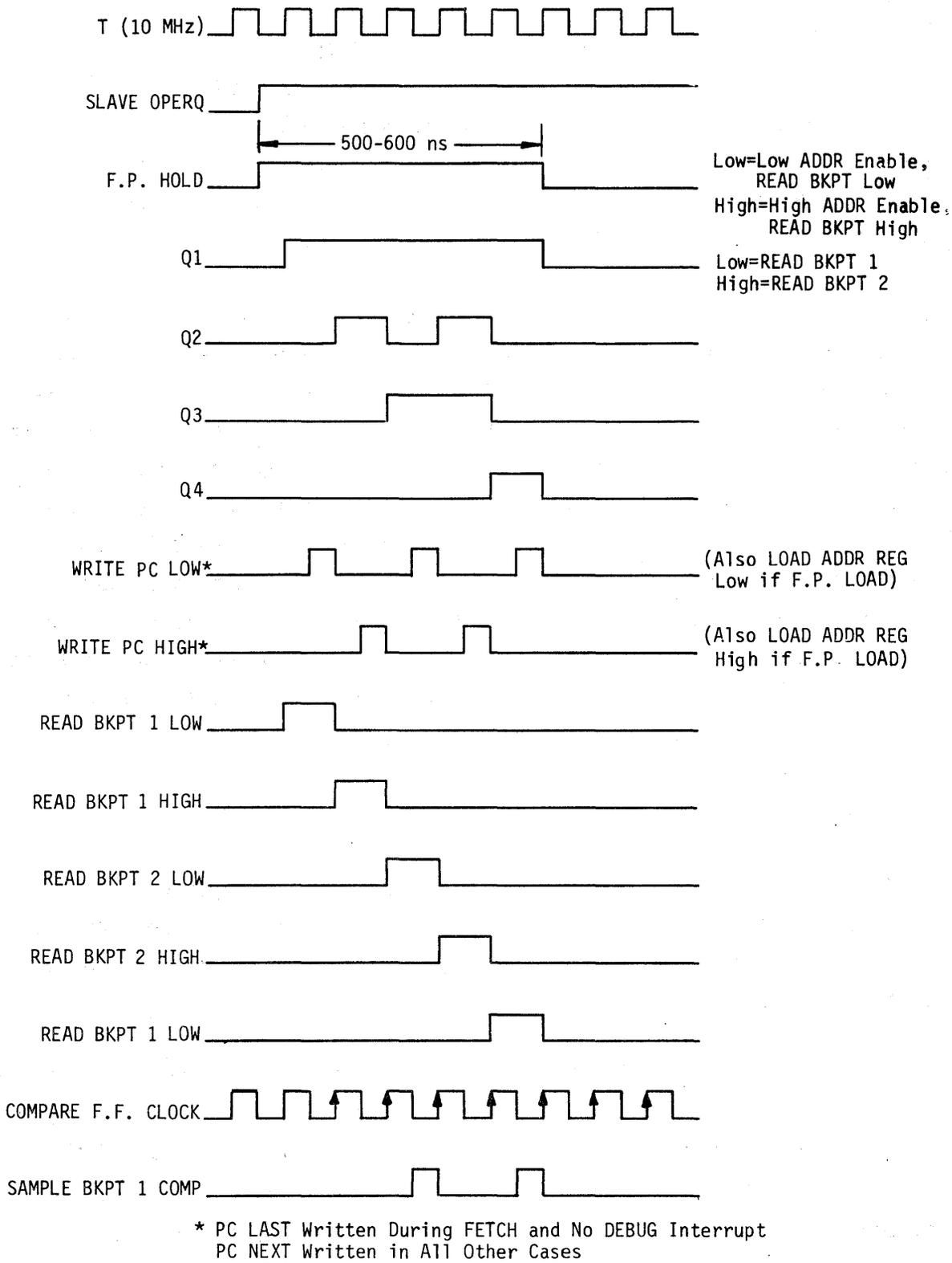
FIGURE 4-11 SEQUENCER TIMING
