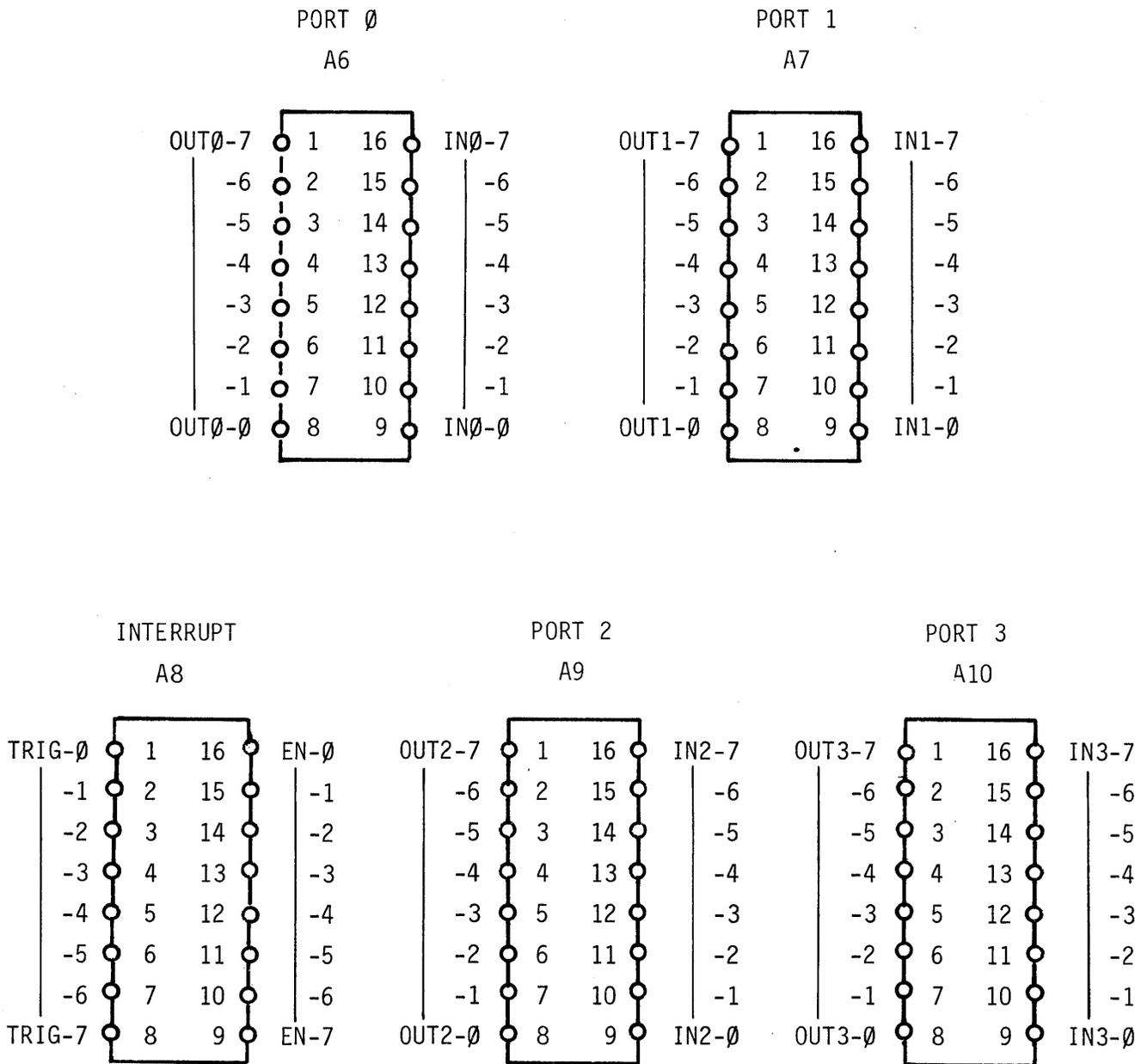
FIGURE 7-8 PARALLEL I/O AND INTERRUPT SIGNAL LOCATIONS
