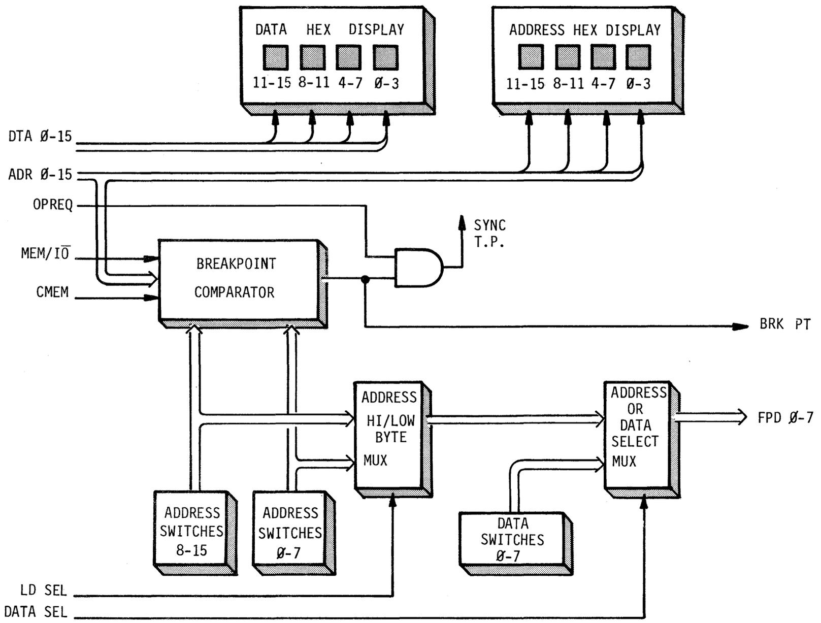
FIGURE 10-3 DATA AND ADDRESS LOGIC DETAILED BLOCK DIAGRAM
