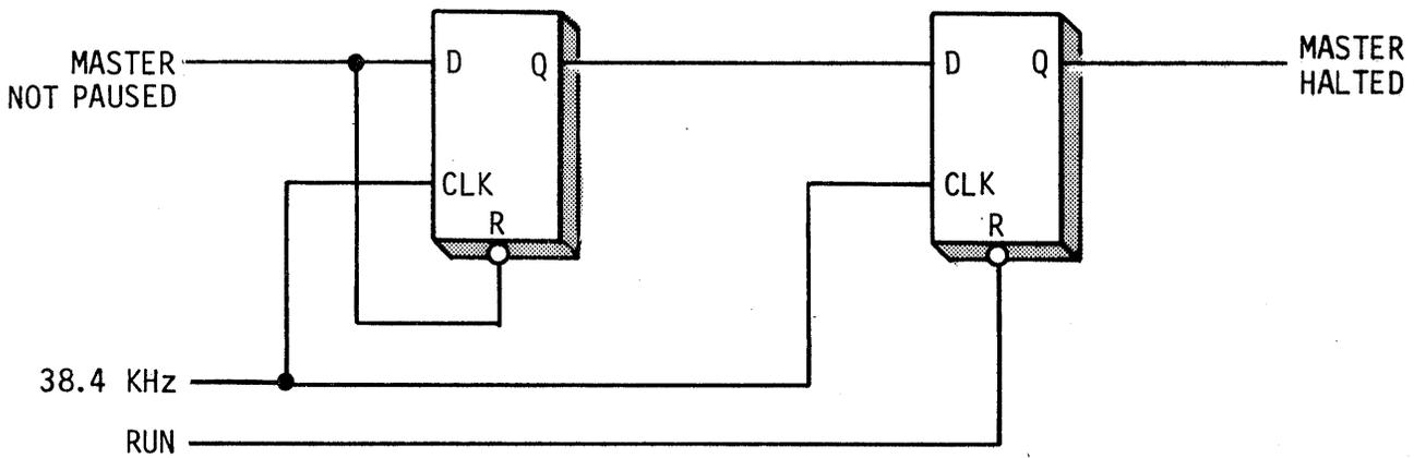
FIGURE 4-7 MASTER HALT DETECTOR
