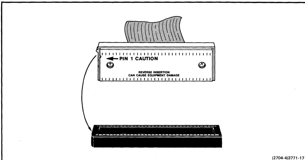
Fig. 3-7. Pin identification and proper plug insertion.
