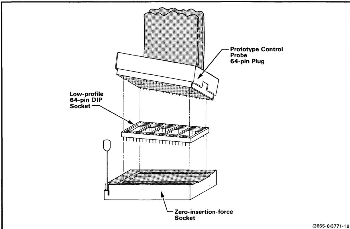
Fig. 3-8. Using a zero-insertion-force socket.
