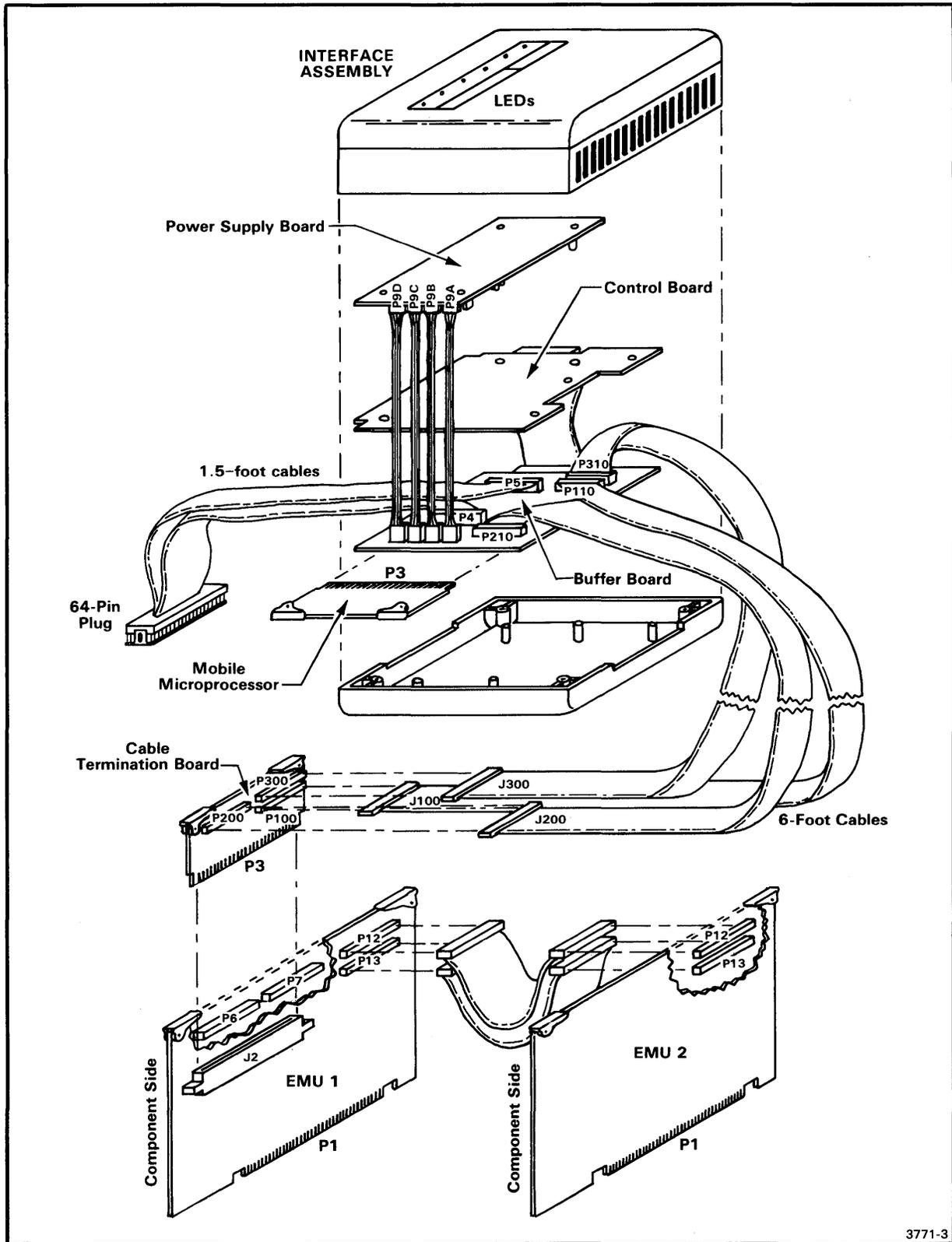
Fig. 1-2. 68000 Emulator Processor and Prototype Control Probe.
