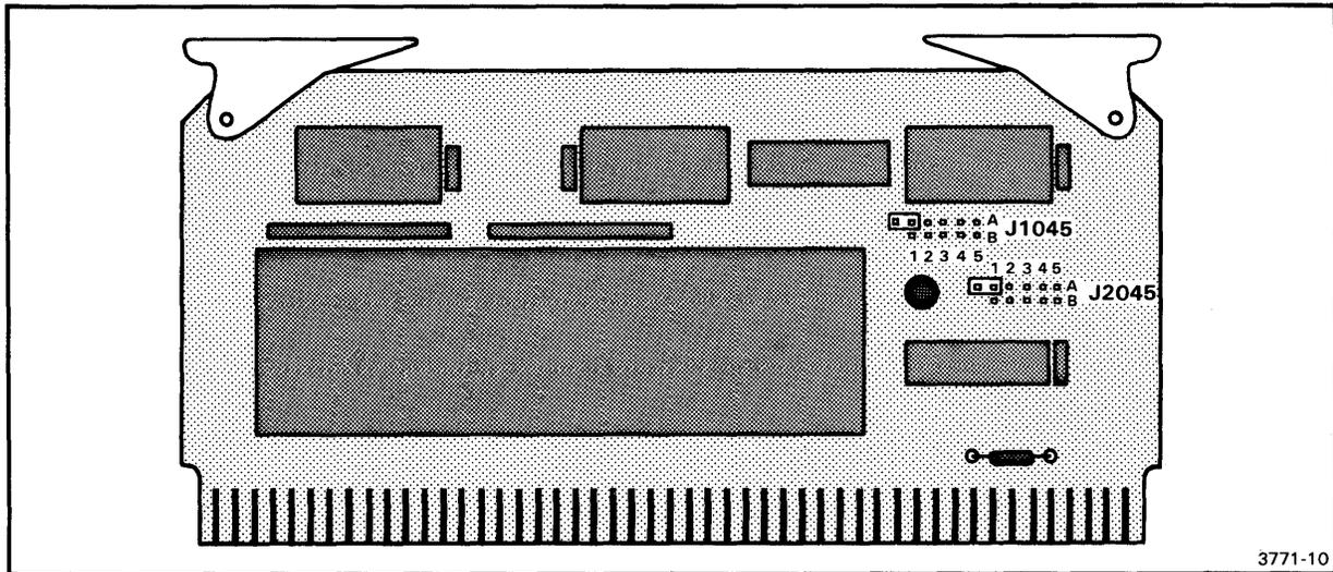
Fig. 2-7. Mobile Microprocessor board jumper locations.
