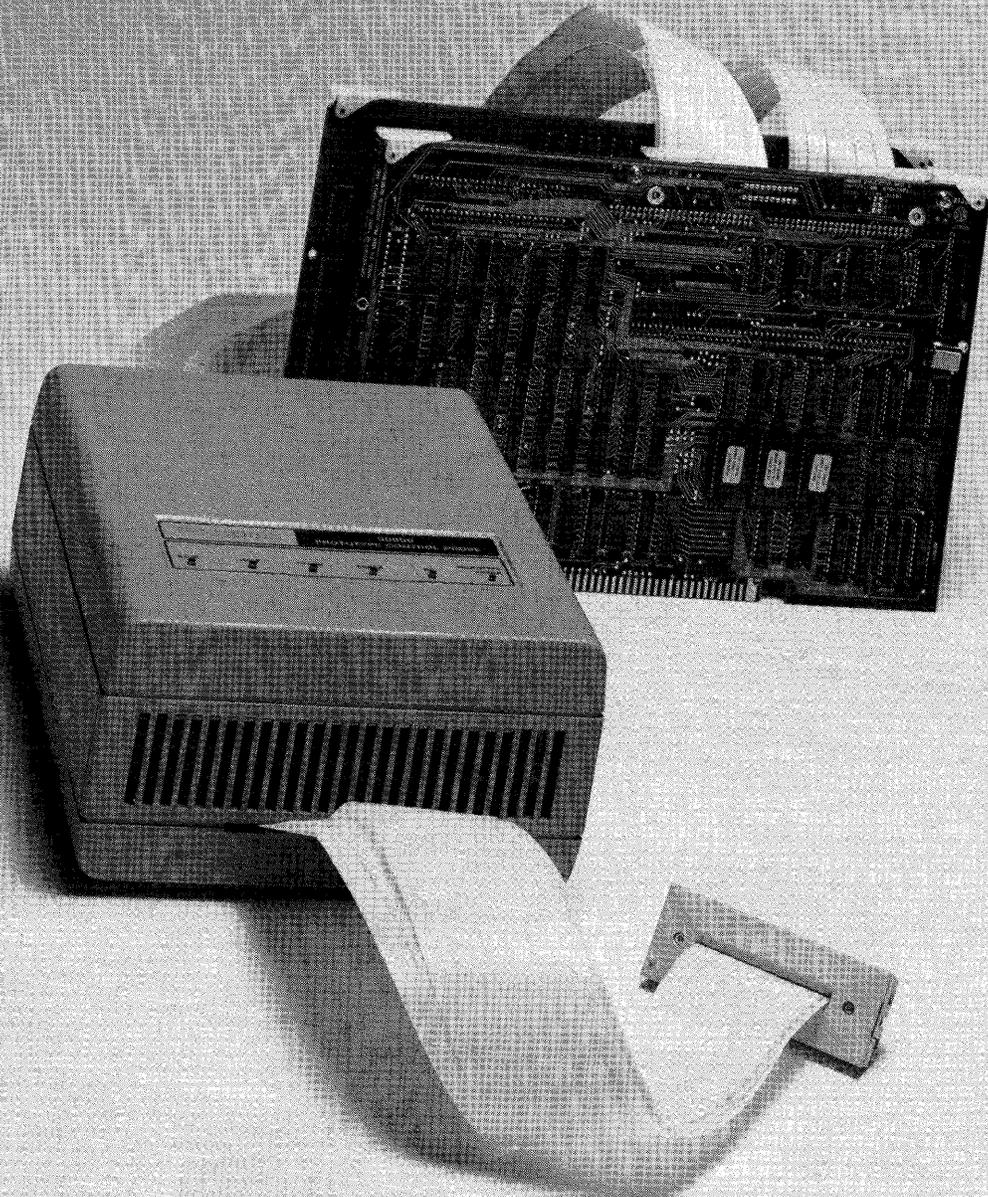
68000 Emulator Processor and Prototype Control Probe
