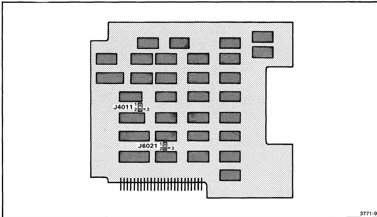
Fig. 2-6. Control board jumper locations.
