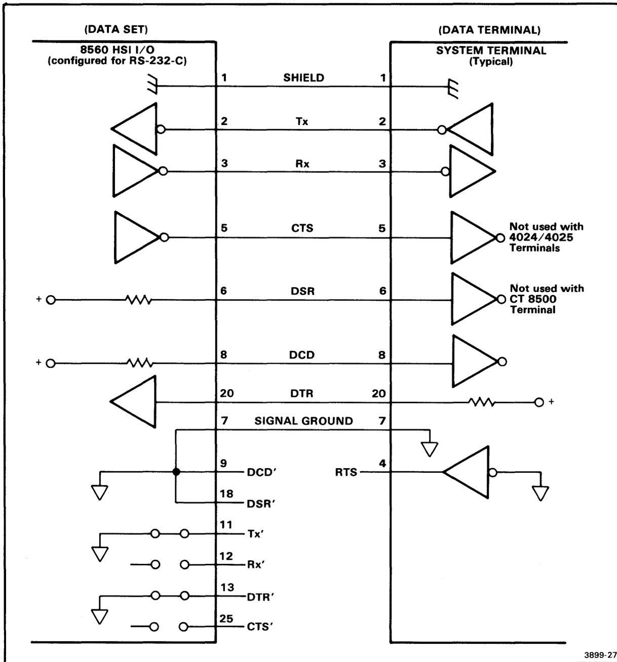
Fig. 5-3. Typical RS-232-C system terminal interface with the 8560 MUSDU.
