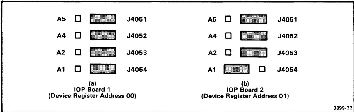
Fig. 4-7. Device Register jumper positions.
