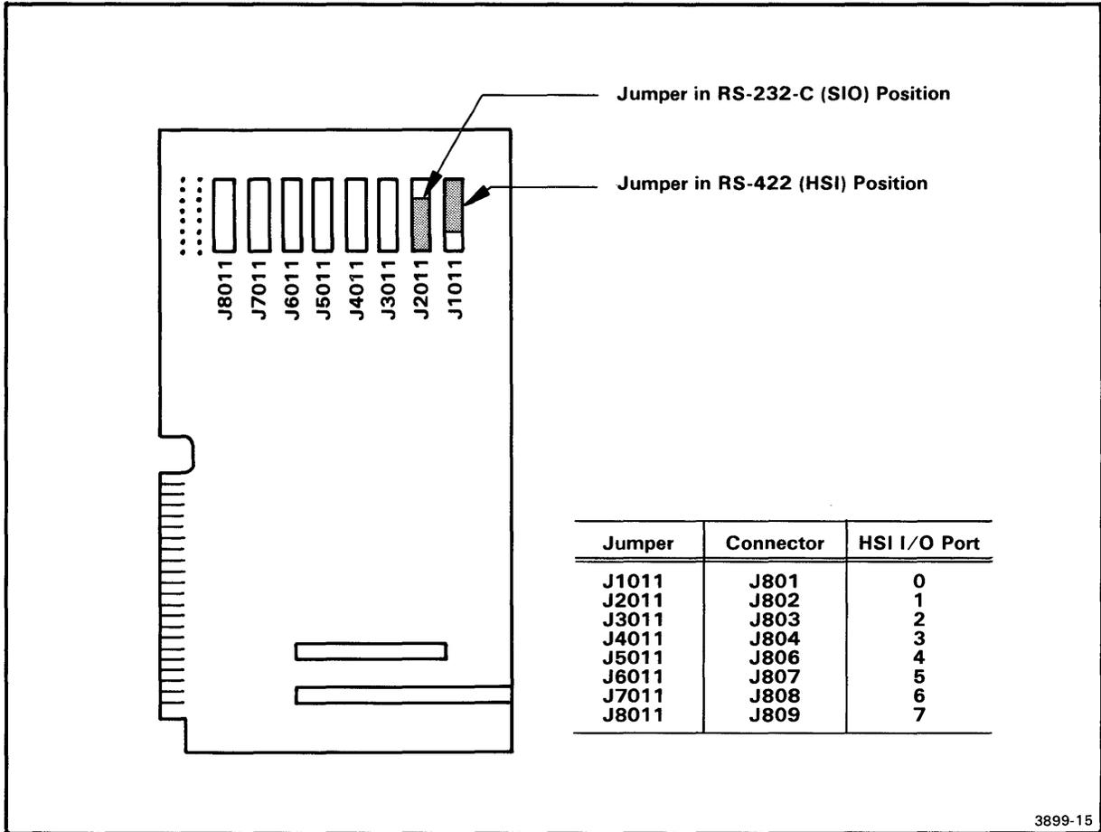
Fig. 4-10. Location of jumpers on the I/O Adapter board.
