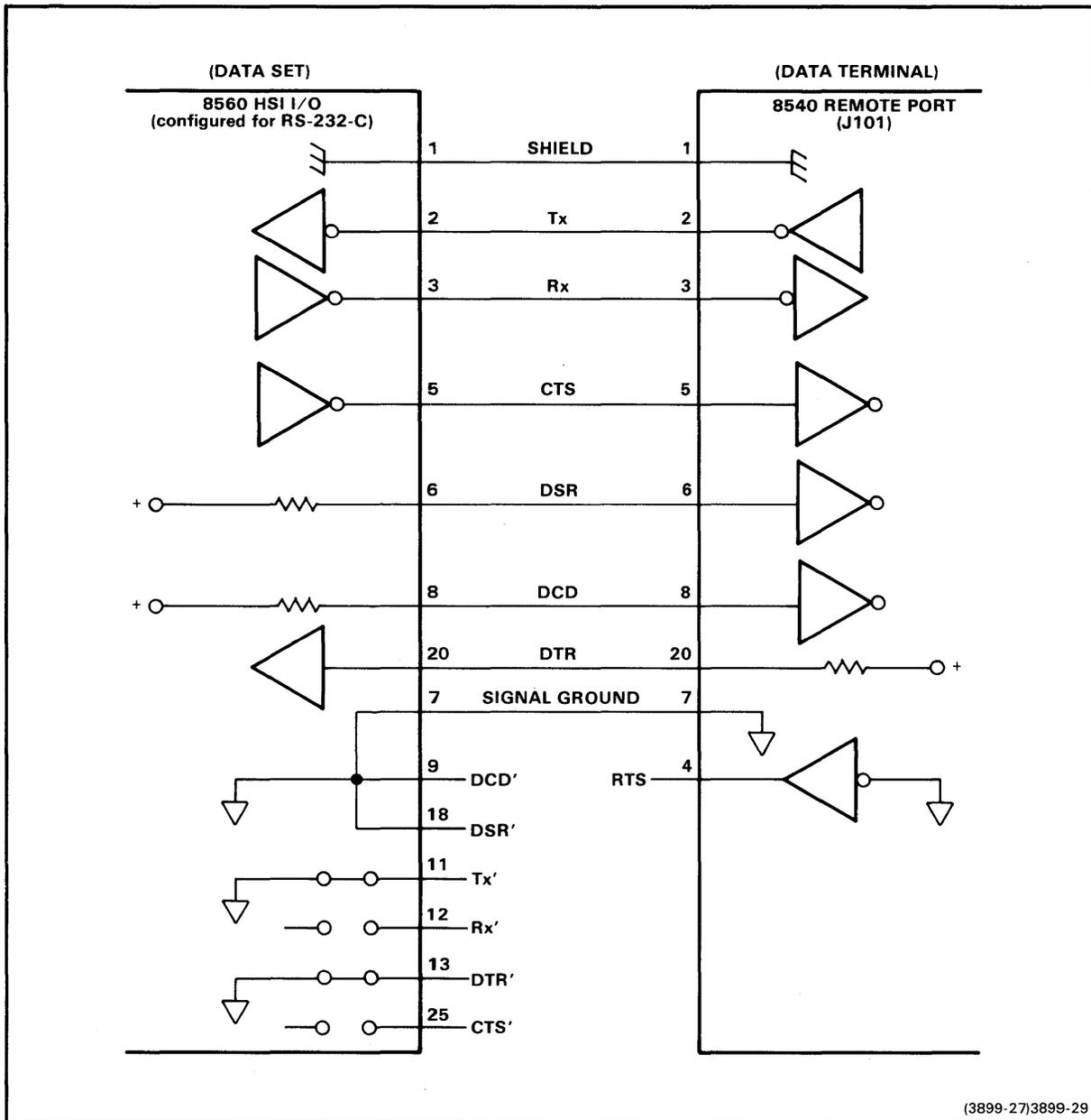
Fig. 5-5. RS-232-C interface lines between the 8560 and the 8540.
