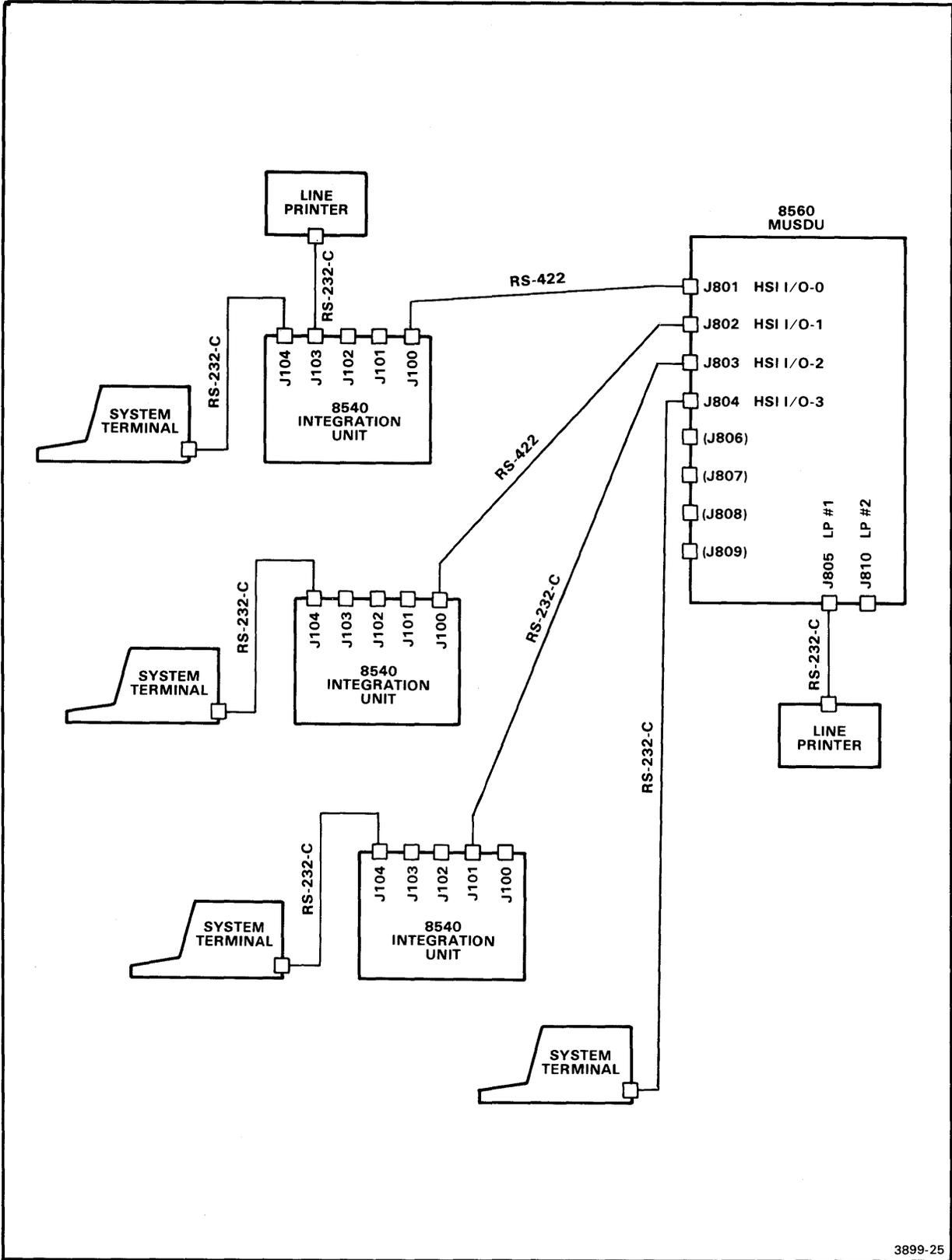
Fig. 5-1. Typical 8560 system configuration.
