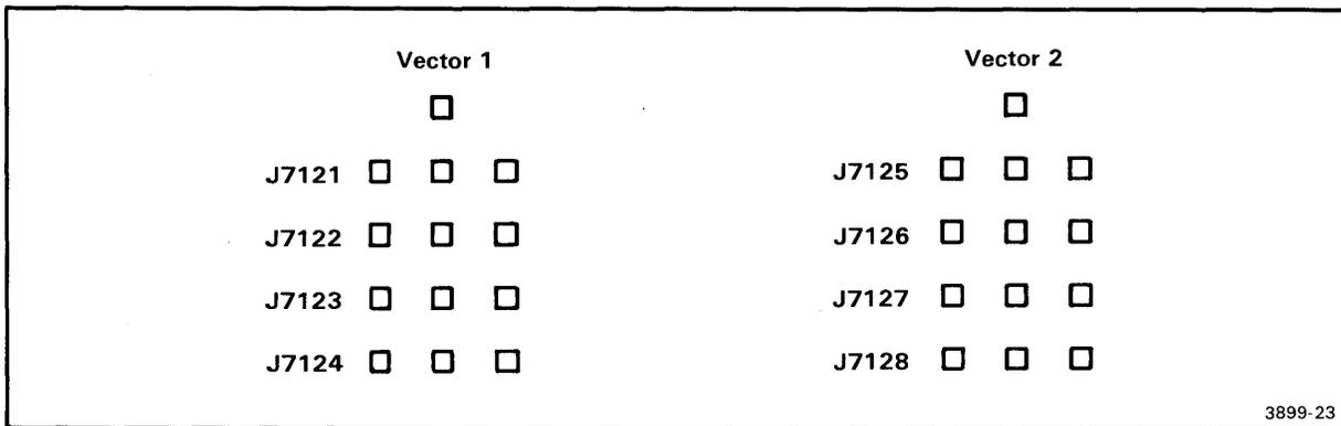
Fig. 4-8. Interrupt Priority jumper arrangement.
