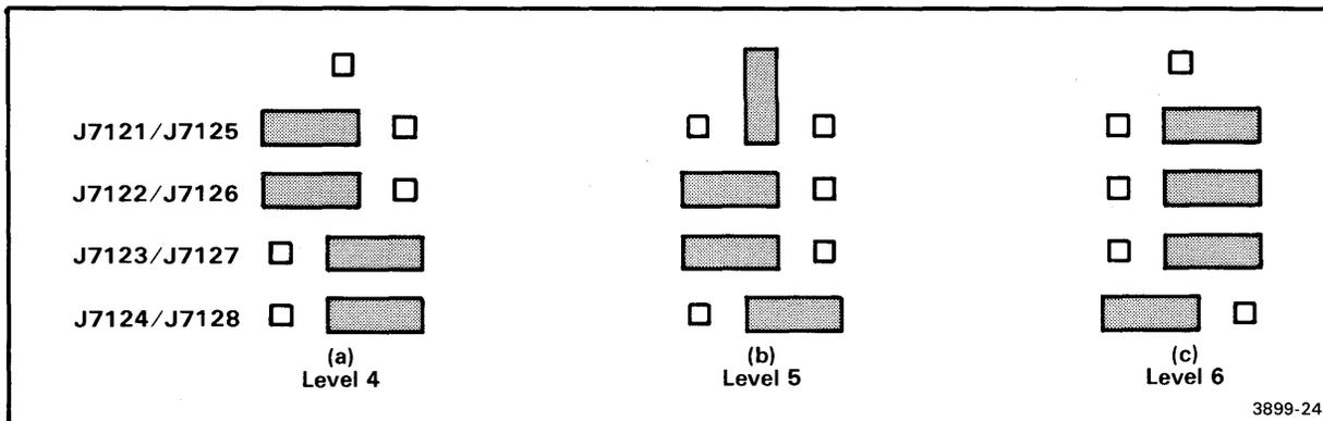
Fig. 4-9. Jumper configurations for interrupt priority levels.
