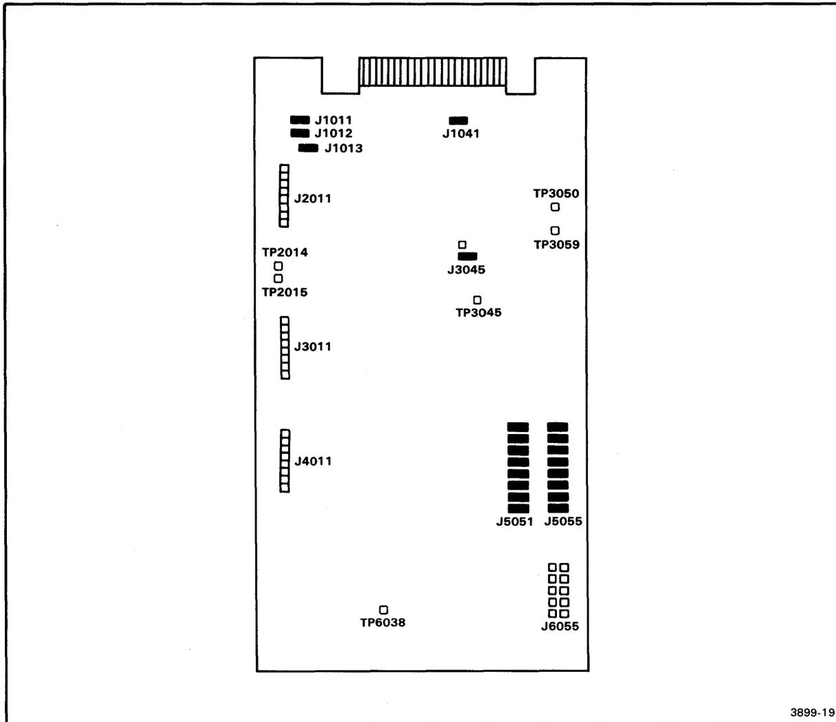
Fig. 4-4. M1220 Interface Card jumper locations.
