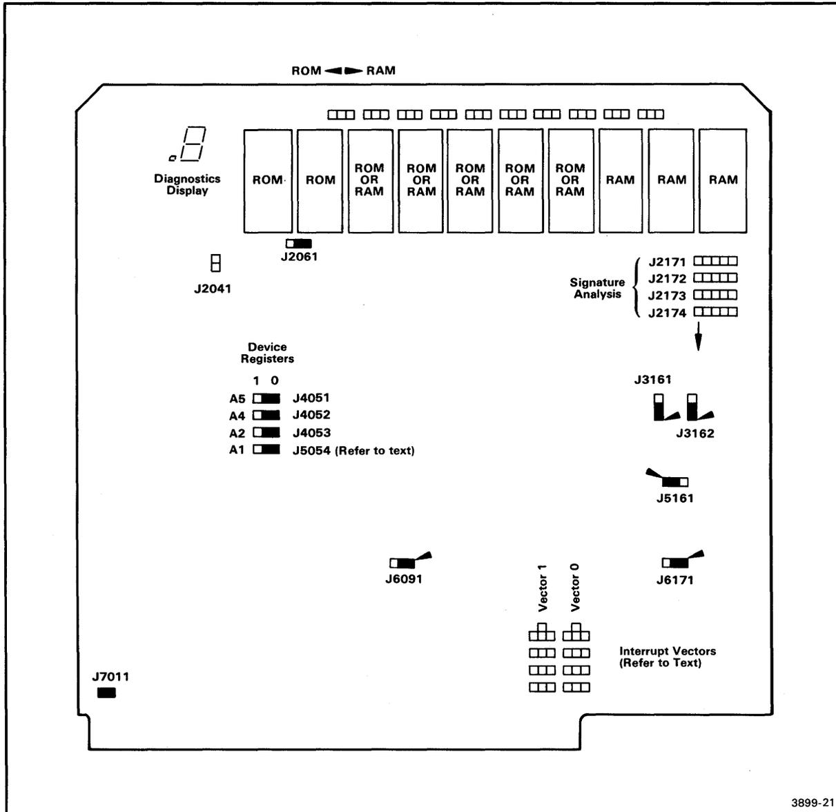
Fig. 4-6. I/O Processor board jumper locations.
