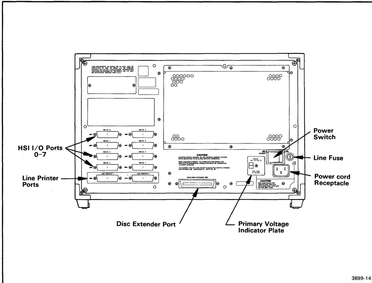
Fig. 3-2. 8560 Rear Panel Controls and Connectors.
