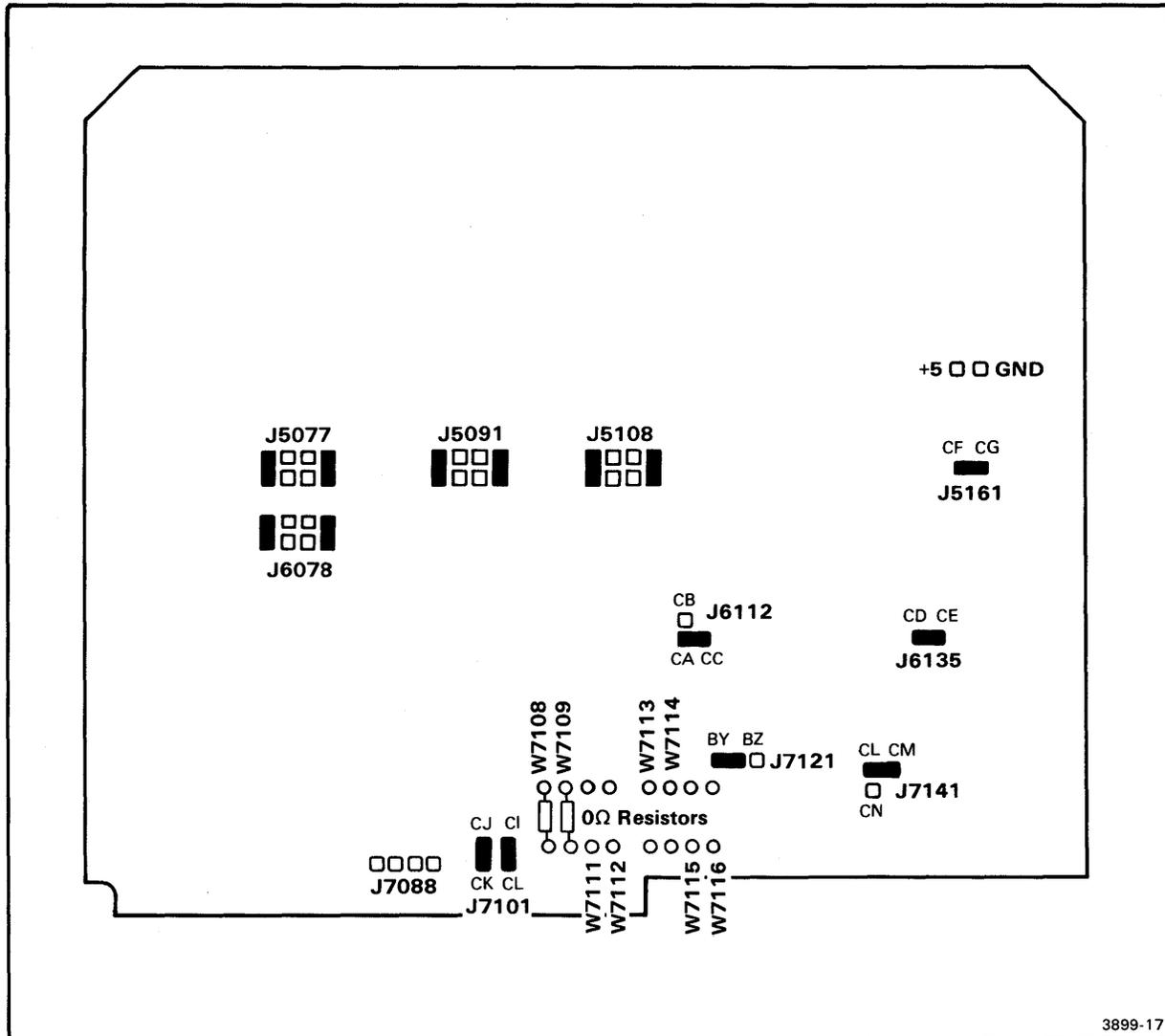
Fig. 4-2. 64K Memory board jumper and strap locations.
