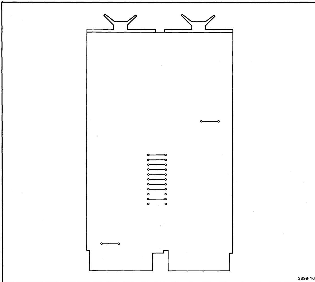
Fig. 4-1. Jumper configuration for the LSI-11/23 Processor board.
