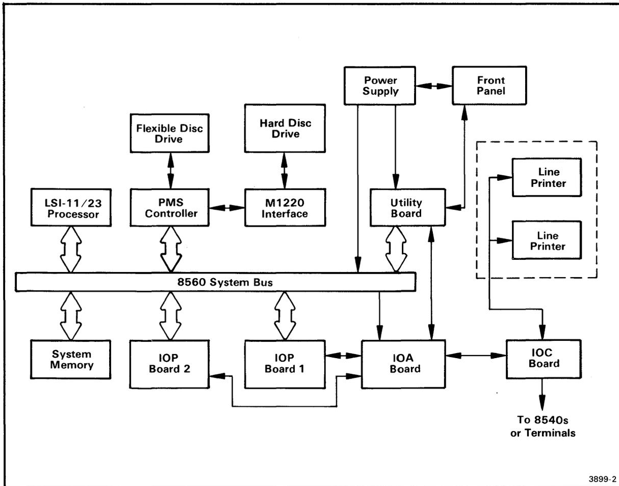
Fig. 1-1. Block Diagram of 8560 Multi-User Software Development Unit.
