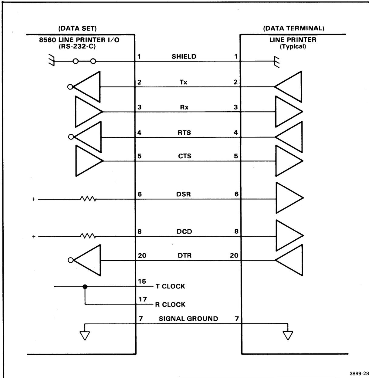
Fig. 5-4. Typical line printer interface with the 8560 MUSDU.
