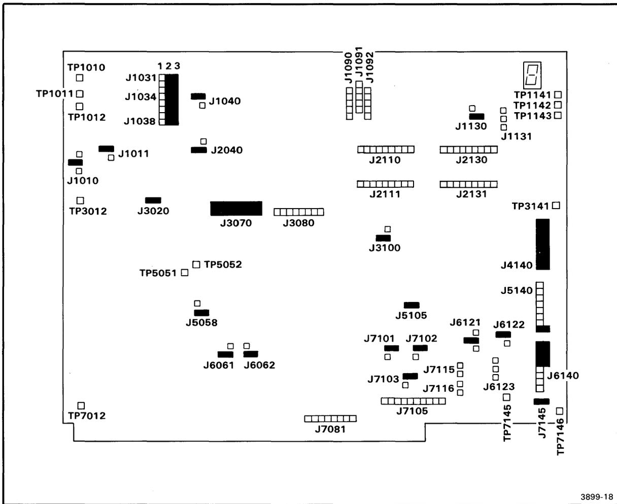
Fig. 4-3. PMS Controller board jumper locations.
